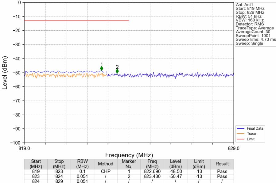
CA\_5B\_SISO\_NTNV\_CC1:5 CC2:3MHz\_CC1:QPSK CC2:QPSK\_CC1:826.5 CC2:830.4MHz\_CC1: 25@0 CC2: 15@0
