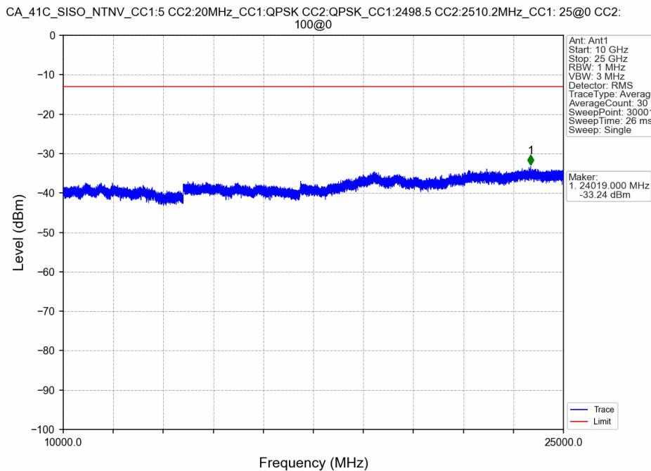
CA\_41C\_SISO\_NTNV\_CC1:5 CC2:20MHz\_CC1:QPSK CC2:QPSK\_CC1:2498.5 CC2:2510.2MHz\_CC1: 25@0 CC2: 100@0
