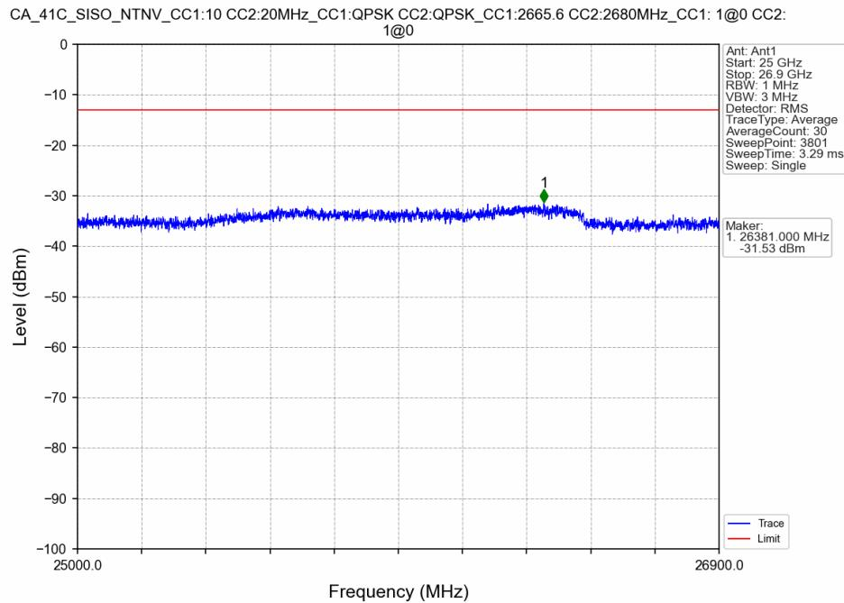
CA\_41C\_SISO\_NTNV\_CC1:10 CC2:20MHz\_CC1:QPSK CC2:QPSK\_CC1:2665.6 CC2:2680MHz\_CC1: 1@49 CC2: 1@99
