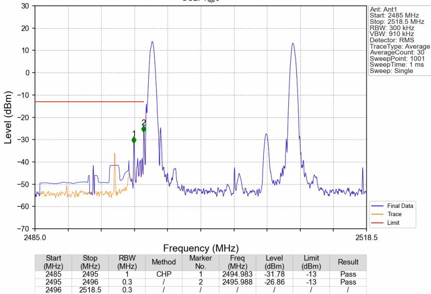
CA\_41C\_SISO\_NTNV\_CC1:15 CC2:10MHz\_CC1:16QAM CC2:16QAM\_CC1:2503.5 CC2:2515.5MHz\_CC1: 1@0 CC2: 1@0
