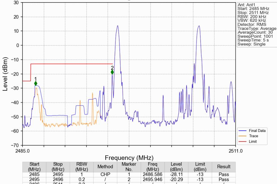
CA\_41C\_SISO\_NTNV\_CC1:10 CC2:20MHz\_CC1:QPSK CC2:QPSK\_CC1:2501 CC2:2515.4MHz\_CC1: 1@0 CC2: 1@0
