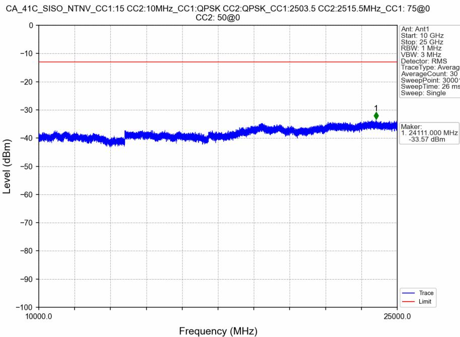
CA\_41C\_SISO\_NTNV\_CC1:15 CC2:10MHz\_CC1:QPSK CC2:QPSK\_CC1:2503.5 CC2:2515.5MHz\_CC1: 75@0 CC2: 50@0
