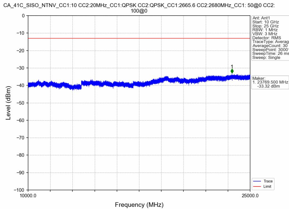
CA\_41C\_SISO\_NTNV\_CC1:10 CC2:20MHz\_CC1:QPSK CC2:QPSK\_CC1:2665.6 CC2:2680MHz\_CC1: 50@0 CC2:
