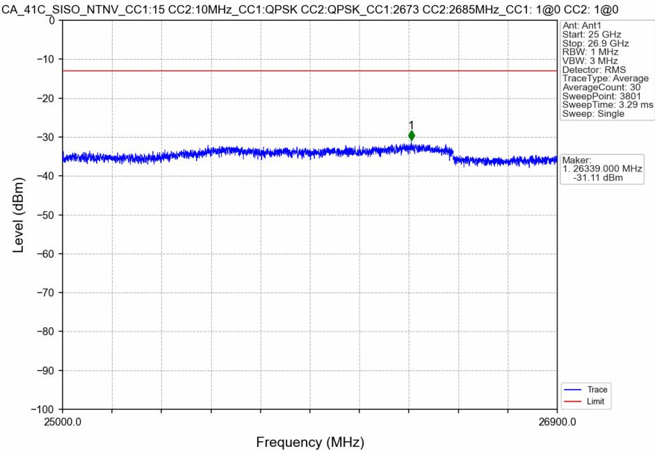
CA\_41C\_SISO\_NTNV\_CC1:15 CC2:10MHz\_CC1:QPSK CC2:QPSK\_CC1:2673 CC2:2685MHz\_CC1: 1@74 CC2: 1@49
