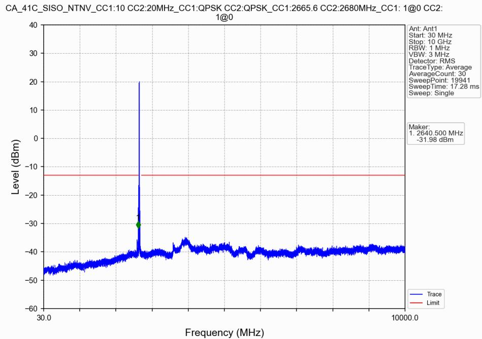
CA\_41C\_SISO\_NTNV\_CC1:10 CC2:20MHz\_CC1:QPSK CC2:QPSK\_CC1:2665.6 CC2:2680MHz\_CC1:1@0 CC2:1@0
