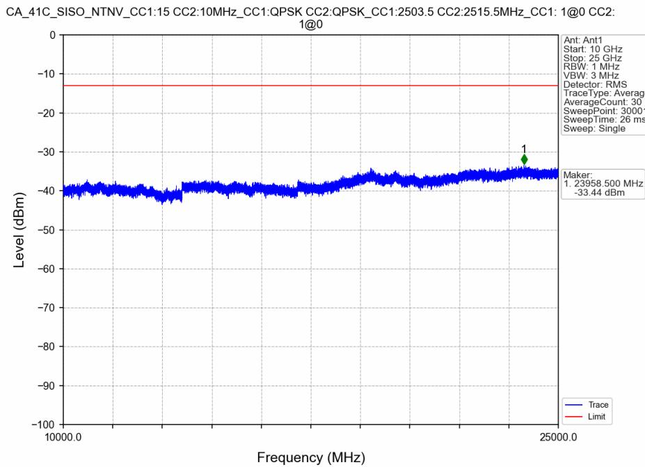
CA\_41C\_SISO\_NTNV\_CC1:15 CC2:10MHz\_CC1:QPSK CC2:QPSK\_CC1:2503.5 CC2:2515.5MHz\_CC1: 1@0 CC2: 1@0
