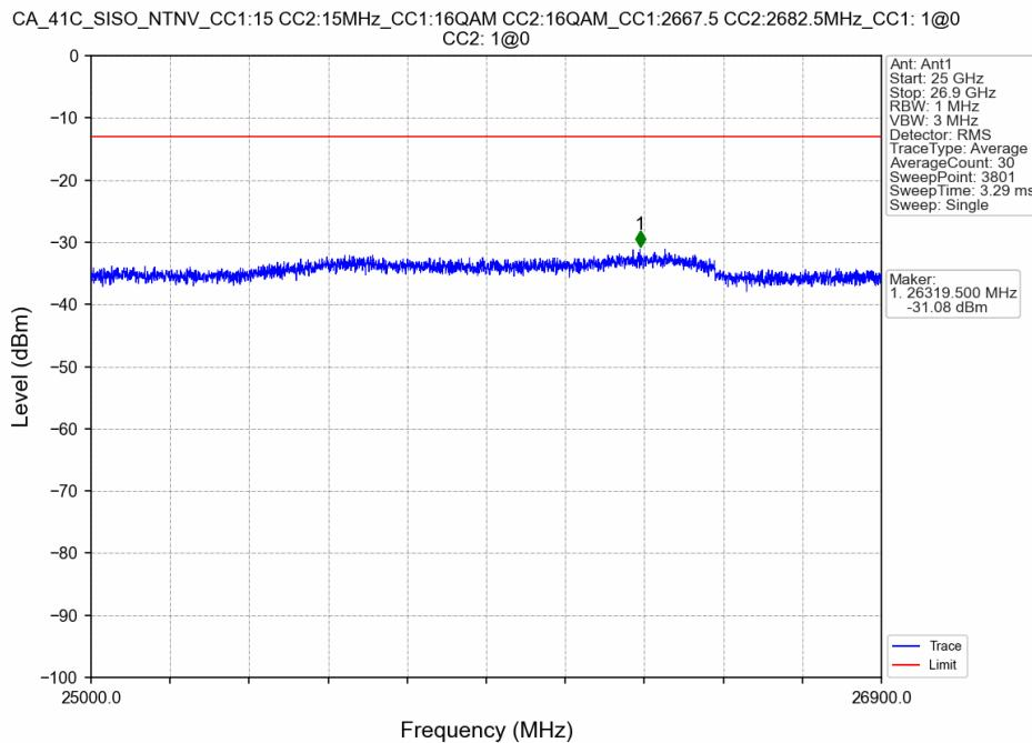
CA\_41C\_SISO\_NTNV\_CC1:15 CC2:15MHz\_CC1:16QAM CC2:16QAM\_CC1:2667.5 CC2:2682.5MHz\_CC1: 1@74
