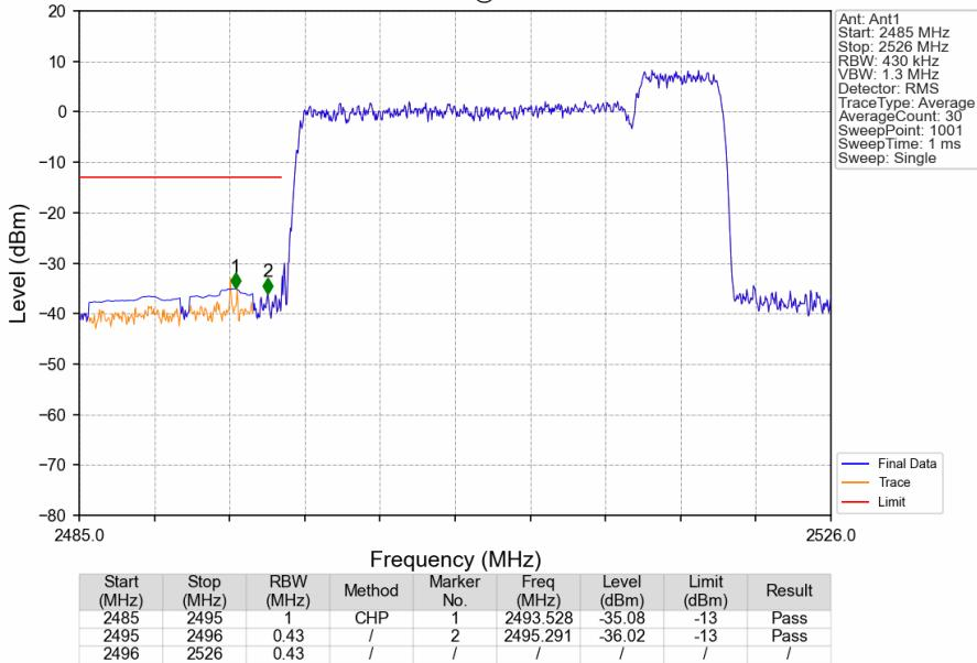
CA\_41C\_SISO\_NTNV\_CC1:20 CC2:5MHz\_CC1:16QAM CC2:16QAM\_CC1:2506 CC2:2517.7MHz\_CC1: 100@0 CC2: 25@0
