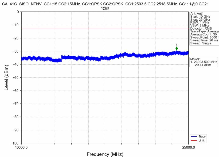
CA\_41C\_SISO\_NTNV\_CC1:15 CC2:15MHz\_CC1:QPSK CC2:QPSK\_CC1:2503.5 CC2:2518.5MHz\_CC1: 1@0 CC2: 1@0
