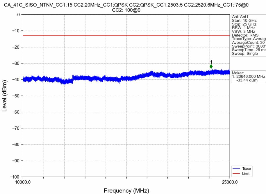
CA\_41C\_SISO\_NTNV\_CC1:15 CC2:20MHz\_CC1:QPSK CC2:QPSK\_CC1:2503.5 CC2:2520.6MHz\_CC1: 75@0 CC2: 100@0
