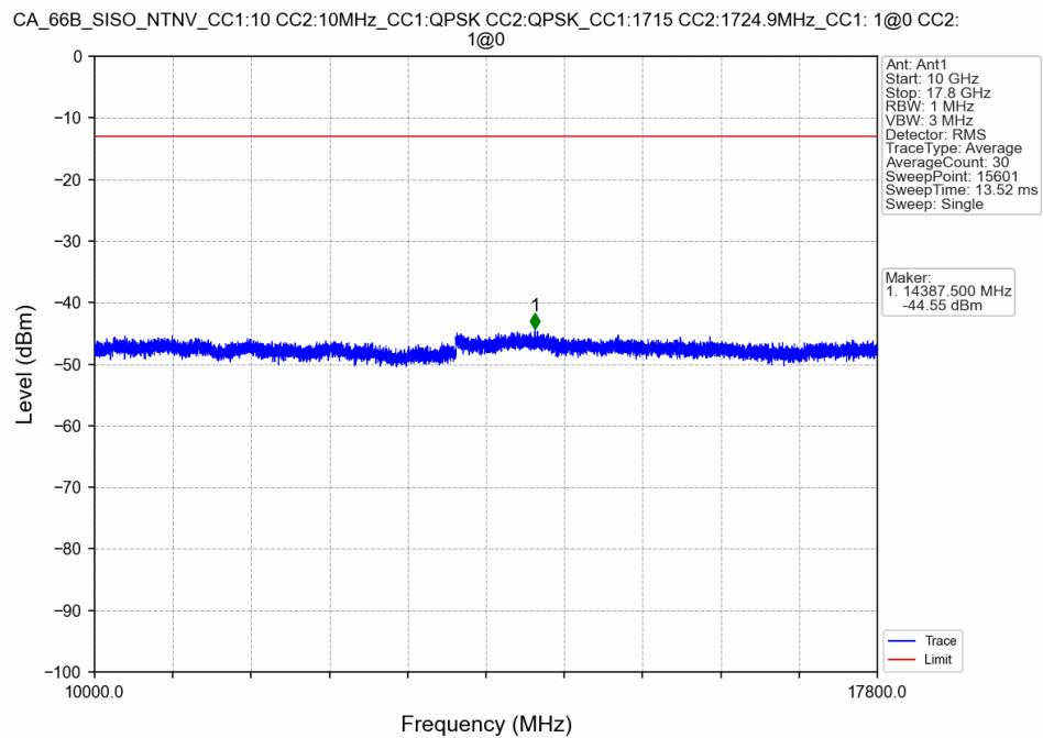
CA\_66B\_SISO\_NTNV\_CC1:10 CC2:10MHz\_CC1:QPSK CC2:QPSK\_CC1:1715 CC2:1724.9MHz\_CC1: 50@0 CC2: 50@0
