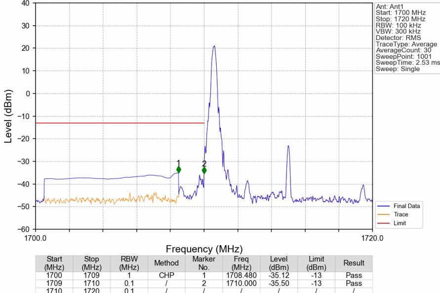
CA\_66B\_SISO\_NTNV\_CC1:10 CC2:10MHz\_CC1:QPSK CC2:QPSK\_CC1:1715 CC2:1724.9MHz\_CC1: 1@0 CC2: 1@0
