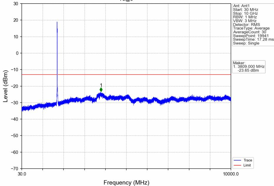
CA\_66B\_SISO\_NTNV\_CC1:5 CC2:15MHz\_CC1:QPSK CC2:QPSK\_CC1:1712.5 CC2:1721.8MHz\_CC1: 25@0 CC2: 75@0
