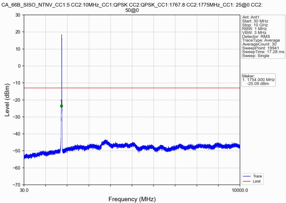
CA\_66B\_SISO\_NTNV\_CC1:5 CC2:10MHz\_CC1:QPSK CC2:QPSK\_CC1:1767.8 CC2:1775MHz\_CC1: 25@0 CC2: 50@0
