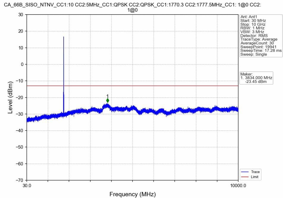
CA\_66B\_SISO\_NTNV\_CC1:10 CC2:5MHz\_CC1:QPSK CC2:QPSK\_CC1:1770.3 CC2:1777.5MHz\_CC1: 1@0 CC2: 1@0
