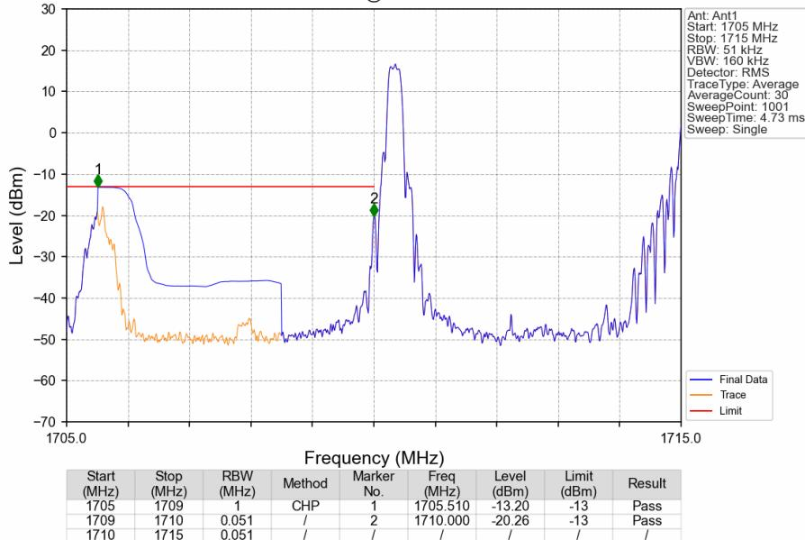
CA\_66B\_SISO\_NTNV\_CC1:5 CC2:15MHz\_CC1:QPSK CC2:QPSK\_CC1:1712.5 CC2:1721.8MHz\_CC1: 1@0 CC2: 1@0
