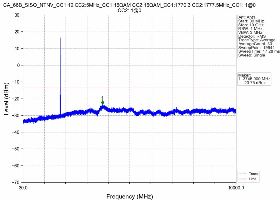
CA\_66B\_SISO\_NTNV\_CC1:10 CC2:5MHz\_CC1:16QAM CC2:16QAM\_CC1:1770.3 CC2:1777.5MHz\_CC1: 1@0 CC2: 1@0
