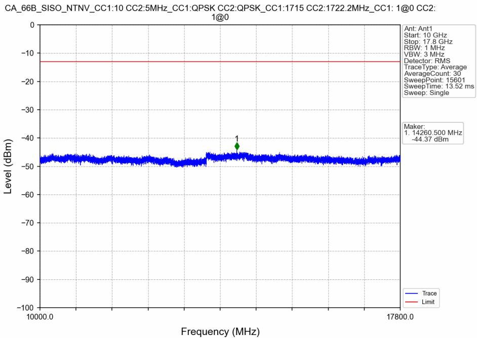
CA\_66B\_SISO\_NTNV\_CC1:10 CC2:5MHz\_CC1:QPSK CC2:QPSK\_CC1:1715 CC2:1722.2MHz\_CC1: 50@0 CC2: 25@0
