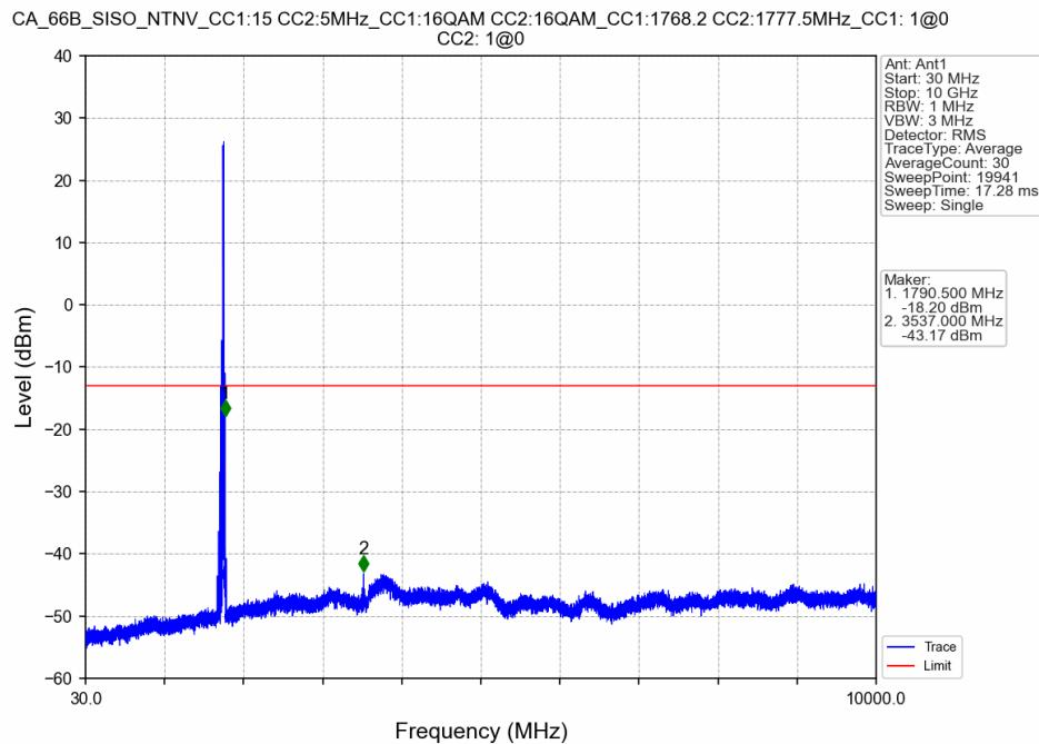
CA\_66B\_SISO\_NTNV\_CC1:15 CC2:5MHz\_CC1:16QAM CC2:16QAM\_CC1:1768.2 CC2:1777.5MHz\_CC1: 1@0 CC2: 1@0
