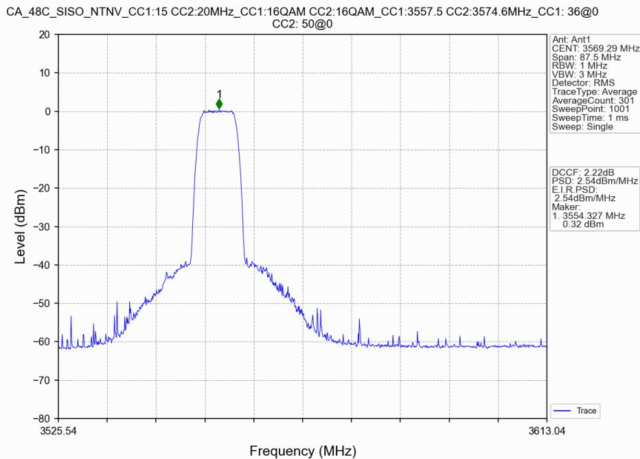
CA\_48C\_SISO\_NTNV\_CC1:15 CC2:20MHz\_CC1:16QAM CC2:16QAM\_CC1:3557.5 CC2:3574.6MHz\_CC1: 36@18
