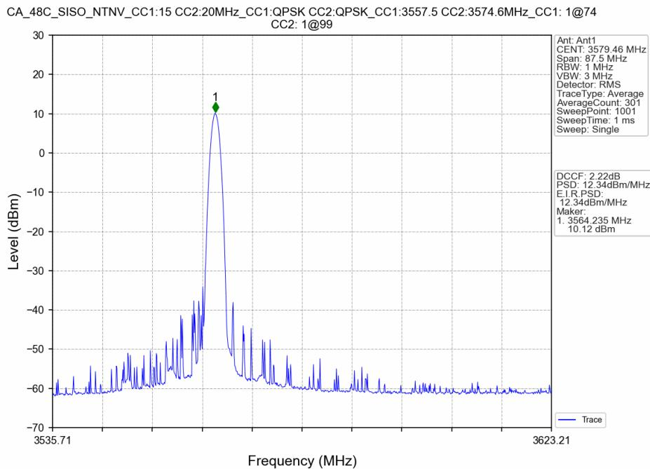
CA\_48C\_SISO\_NTNV\_CC1:15 CC2:20MHz\_CC1:QPSK CC2:QPSK\_CC1:3557.5 CC2:3574.6MHz\_CC1: 36@0 CC2:
