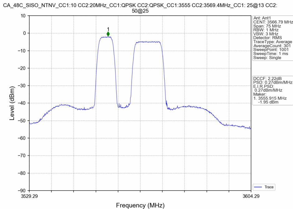
CA\_48C\_SISO\_NTNV\_CC1:10 CC2:20MHz\_CC1:QPSK CC2:QPSK\_CC1:3555 CC2:3569.4MHz\_CC1: 25@25 CC2:
