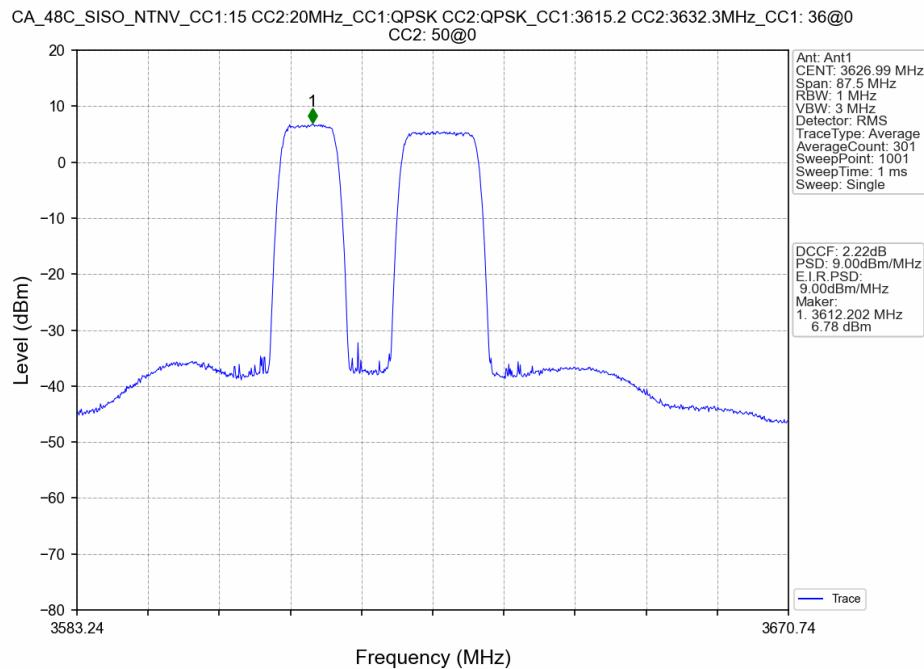
CA\_48C\_SISO\_NTNV\_CC1:15 CC2:20MHz\_CC1:QPSK CC2:QPSK\_CC1:3615.2 CC2:3632.3MHz\_CC1: 36@18 CC2: 50@25
