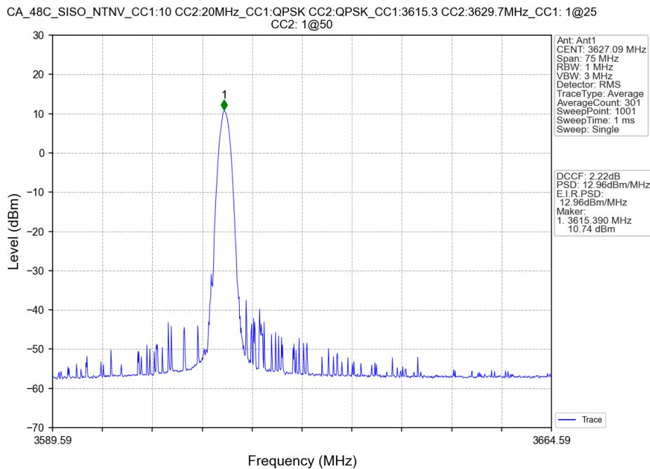
CA\_48C\_SISO\_NTNV\_CC1:10 CC2:20MHz\_CC1:QPSK CC2:QPSK\_CC1:3615.3 CC2:3629.7MHz\_CC1: 1@49 CC2:
