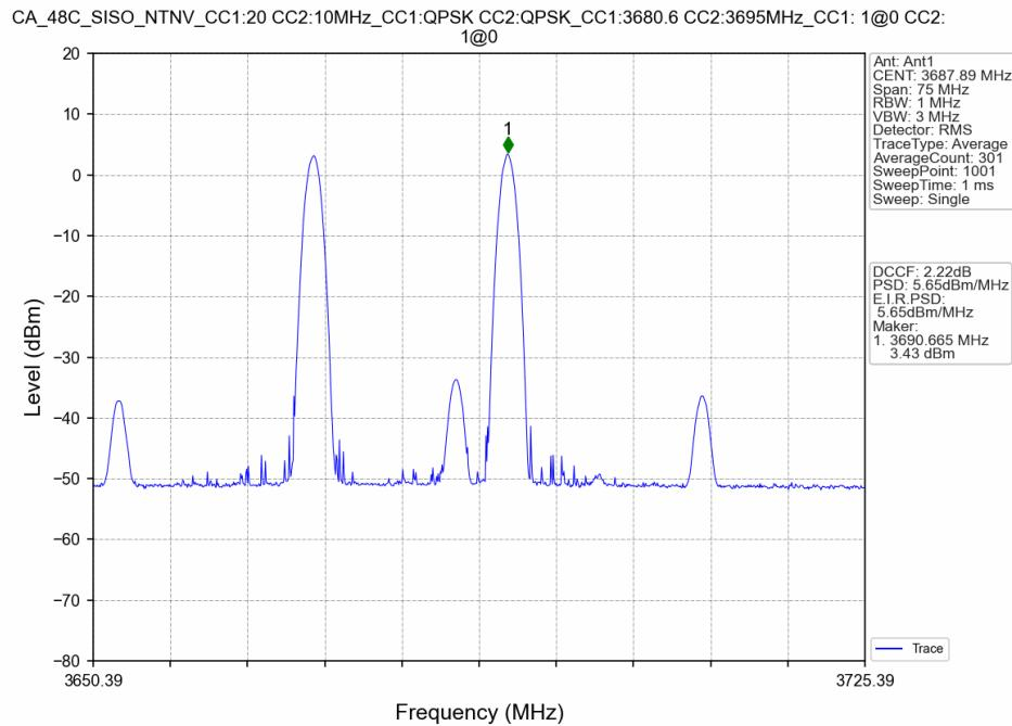
CA\_48C\_SISO\_NTNV\_CC1:20 CC2:10MHz\_CC1:QPSK CC2:QPSK\_CC1:3680.6 CC2:3695MHz\_CC1: 1@50 CC2: 1@25
