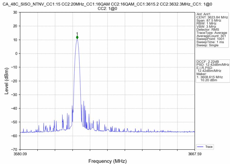
CA\_48C\_SISO\_NTNV\_CC1:15 CC2:20MHz\_CC1:16QAM CC2:16QAM\_CC1:3615.2 CC2:3632.3MHz\_CC1: 1@38 CC2: 1@50
