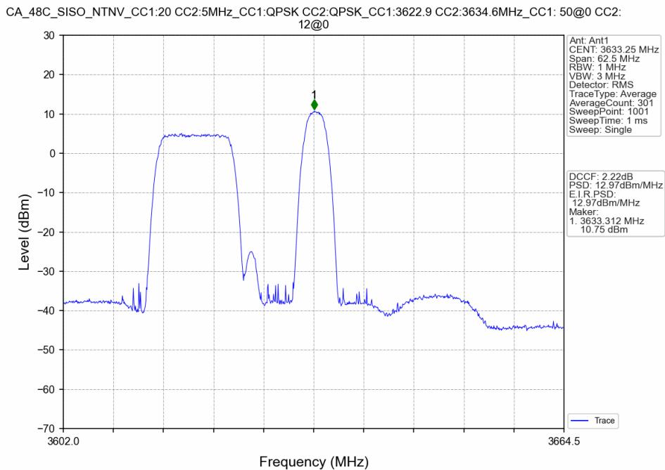
CA\_48C\_SISO\_NTNV\_CC1:20 CC2:5MHz\_CC1:QPSK CC2:QPSK\_CC1:3622.9 CC2:3634.6MHz\_CC1: 50@25 CC2: 12@6
