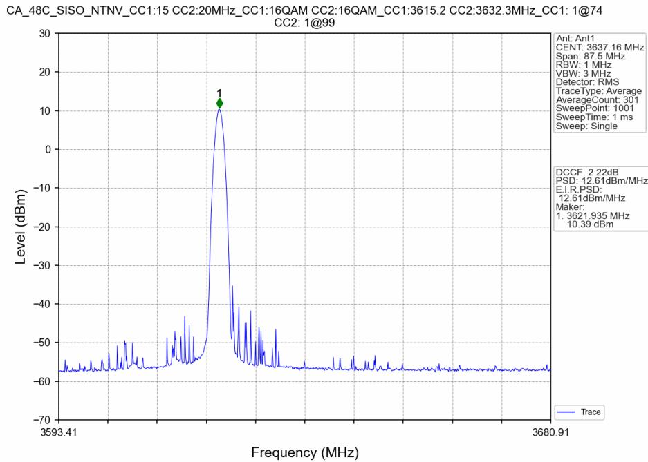
CA\_48C\_SISO\_NTNV\_CC1:15 CC2:20MHz\_CC1:16QAM CC2:16QAM\_CC1:3615.2 CC2:3632.3MHz\_CC1: 36@0
