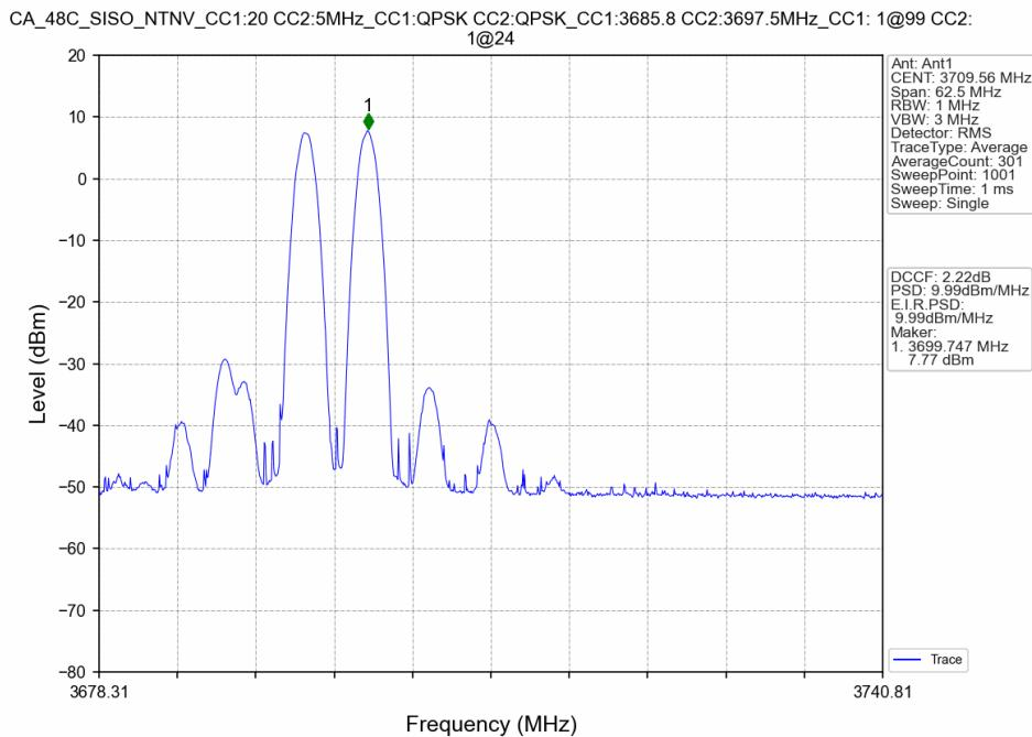
CA\_48C\_SISO\_NTNV\_CC1:20 CC2:5MHz\_CC1:QPSK CC2:QPSK\_CC1:3685.8 CC2:3697.5MHz\_CC1: 50@0 CC2: 12@0
