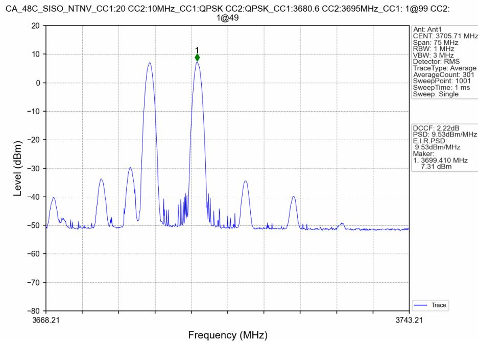
CA\_48C\_SISO\_NTNV\_CC1:20 CC2:10MHz\_CC1:QPSK CC2:QPSK\_CC1:3680.6 CC2:3695MHz\_CC1: 50@0 CC2:
