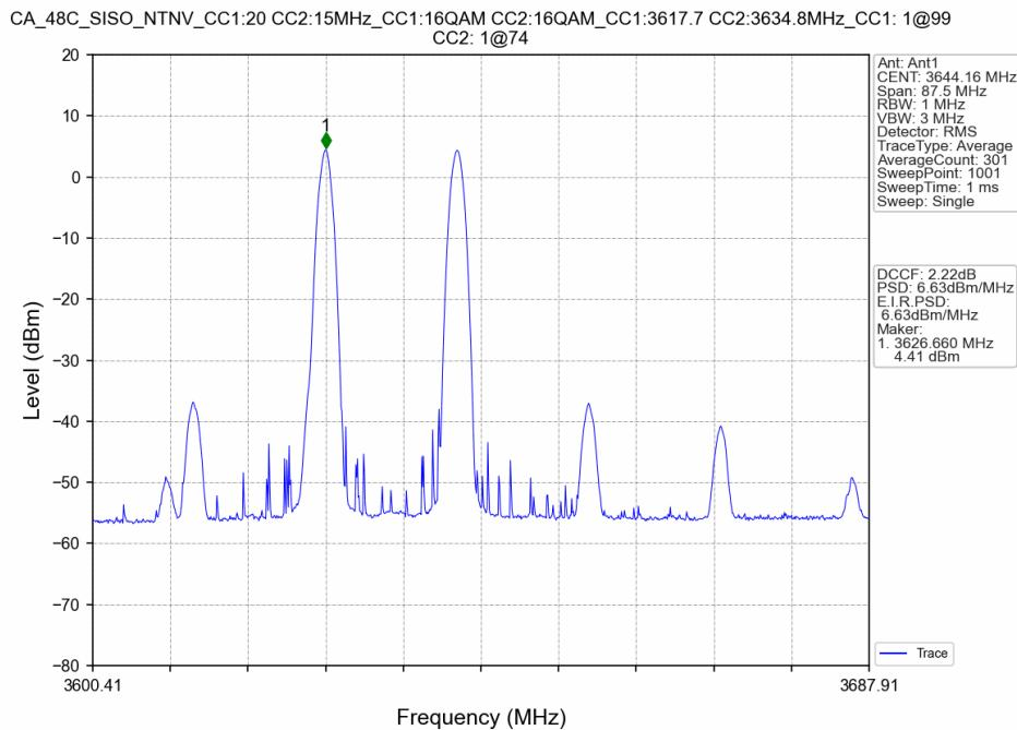
CA\_48C\_SISO\_NTNV\_CC1:20 CC2:15MHz\_CC1:16QAM CC2:16QAM\_CC1:3617.7 CC2:3634.8MHz\_CC1: 50@0
