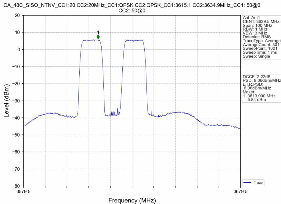
CA\_48C\_SISO\_NTNV\_CC1:20 CC2:20MHz\_CC1:QPSK CC2:QPSK\_CC1:3615.1 CC2:3634.9MHz\_CC1: 50@25 CC2: 50@25
