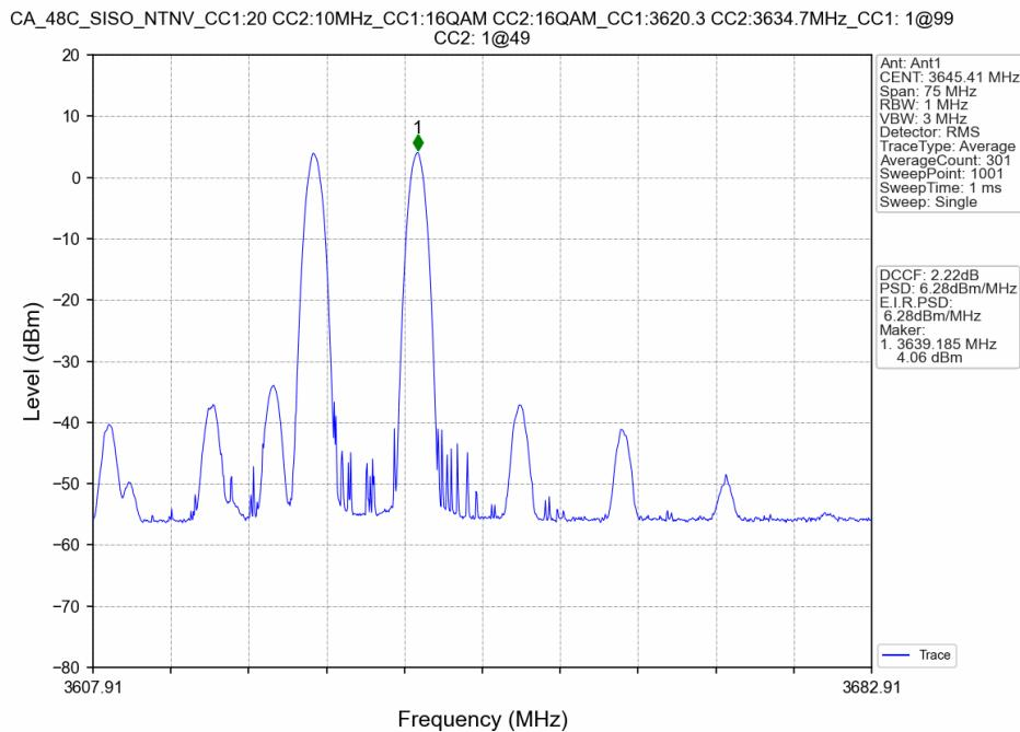
CA\_48C\_SISO\_NTNV\_CC1:20 CC2:10MHz\_CC1:16QAM CC2:16QAM\_CC1:3620.3 CC2:3634.7MHz\_CC1: 50@0
