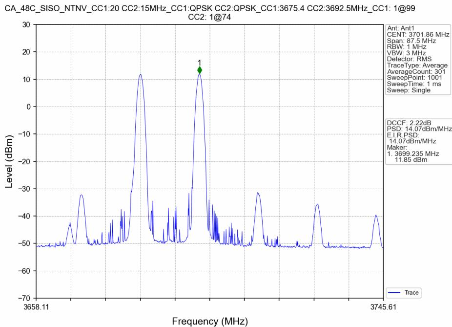
CA\_48C\_SISO\_NTNV\_CC1:20 CC2:15MHz\_CC1:QPSK CC2:QPSK\_CC1:3675.4 CC2:3692.5MHz\_CC1: 50@0 CC2:
