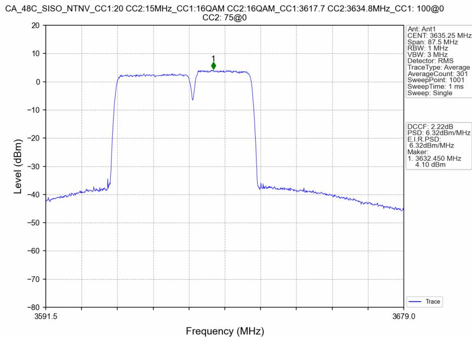
CA\_48C\_SISO\_NTNV\_CC1:20 CC2:15MHz\_CC1:16QAM CC2:16QAM\_CC1:3675.4 CC2:3692.5MHz\_CC1: 1@0 CC2: 1@0
