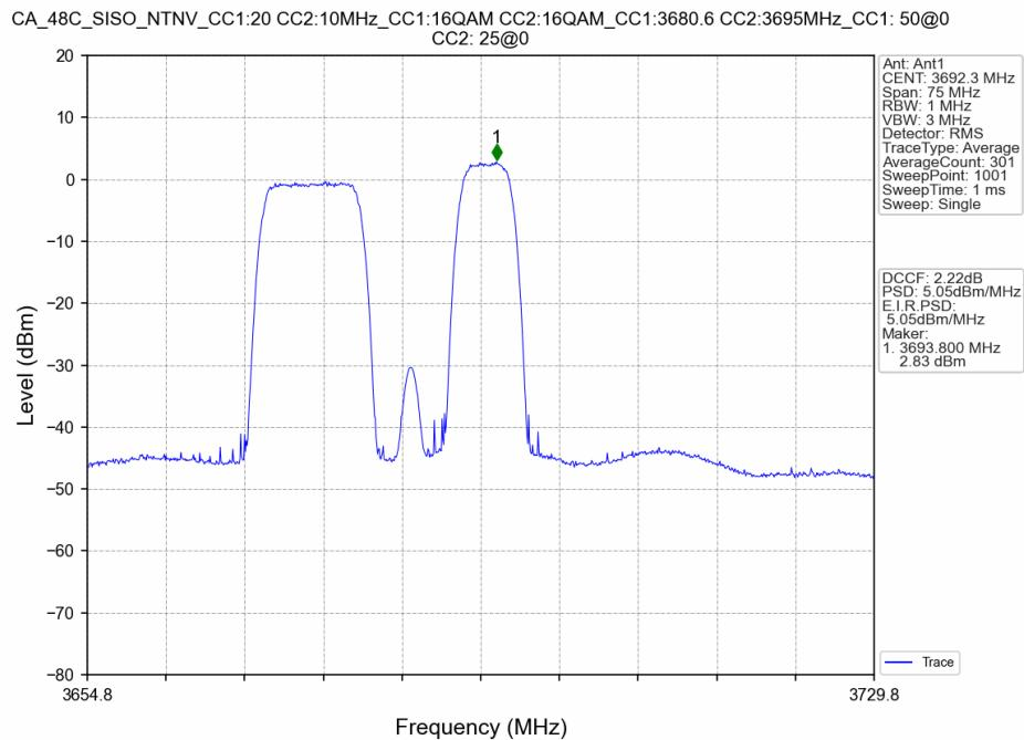
CA\_48C\_SISO\_NTNV\_CC1:20 CC2:10MHz\_CC1:16QAM CC2:16QAM\_CC1:3680.6 CC2:3695MHz\_CC1: 50@25
