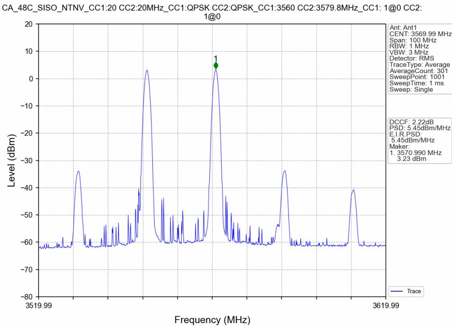
CA\_48C\_SISO\_NTNV\_CC1:20 CC2:20MHz\_CC1:QPSK CC2:QPSK\_CC1:3560 CC2:3579.8MHz\_CC1: 1@50 CC2: 1@50
