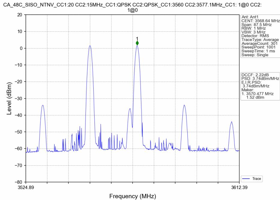
CA\_48C\_SISO\_NTNV\_CC1:20 CC2:15MHz\_CC1:QPSK CC2:QPSK\_CC1:3560 CC2:3577.1MHz\_CC1: 1@50 CC2: 1@38
