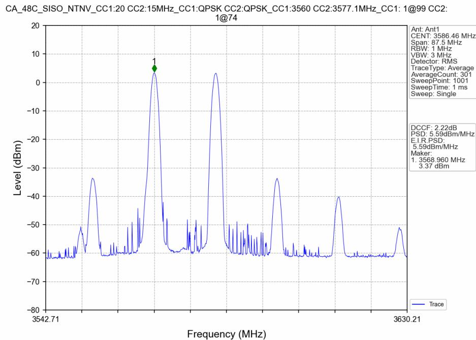
CA\_48C\_SISO\_NTNV\_CC1:20 CC2:15MHz\_CC1:QPSK CC2:QPSK\_CC1:3560 CC2:3577.1MHz\_CC1: 50@0 CC2:
