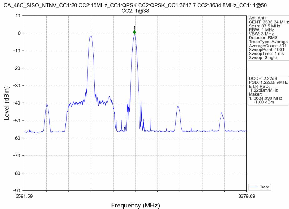
CA\_48C\_SISO\_NTNV\_CC1:20 CC2:15MHz\_CC1:QPSK CC2:QPSK\_CC1:3617.7 CC2:3634.8MHz\_CC1: 1@99 CC2:
