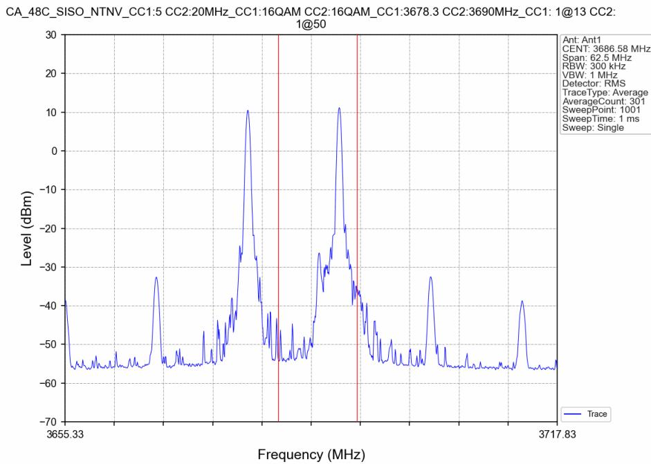
CA\_48C\_SISO\_NTNV\_CC1:5 CC2:20MHz\_CC1:16QAM CC2:16QAM\_CC1:3678.3 CC2:3690MHz\_CC1: 1@24 CC2: 1@99
