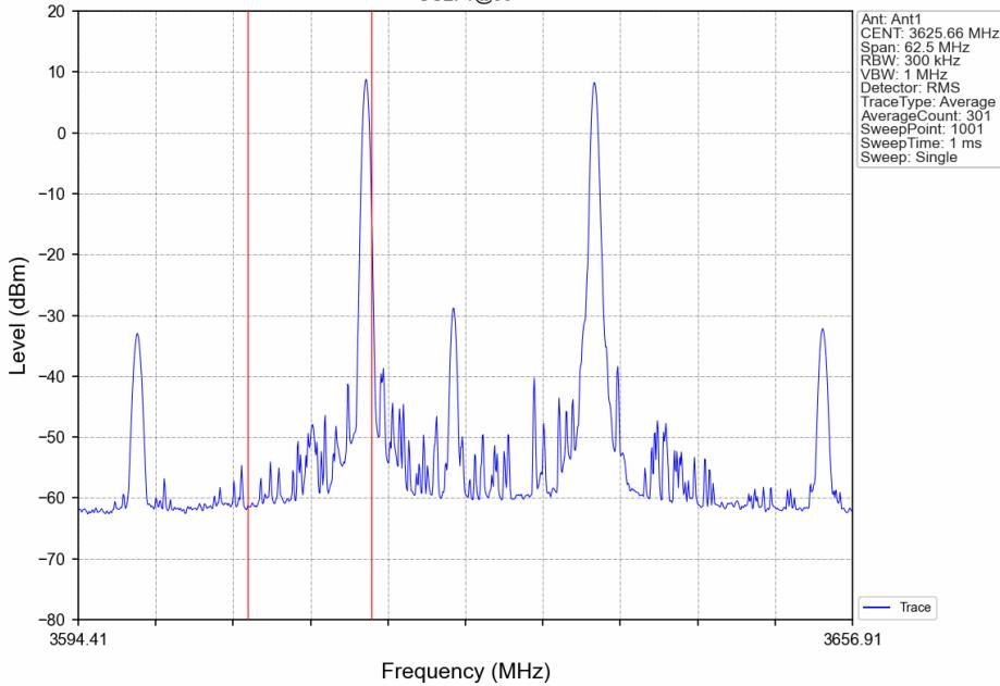
CA\_48C\_SISO\_NTNV\_CC1:5 CC2:20MHz\_CC1:16QAM CC2:16QAM\_CC1:3615.4 CC2:3627.1MHz\_CC1: 12@0 CC2: 50@0
