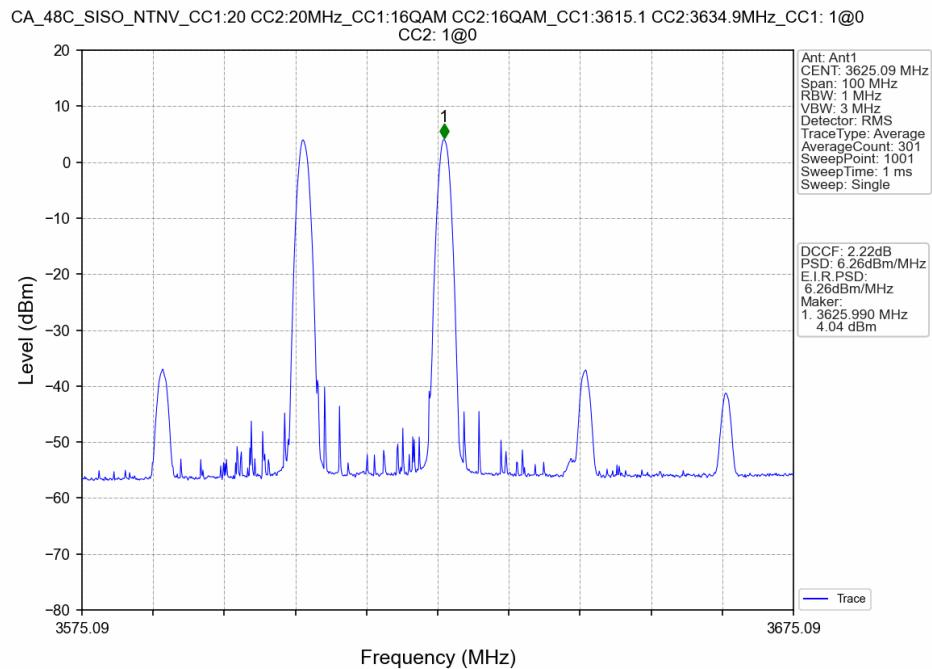
CA\_48C\_SISO\_NTNV\_CC1:20 CC2:20MHz\_CC1:16QAM CC2:16QAM\_CC1:3615.1 CC2:3634.9MHz\_CC1: 1@50
