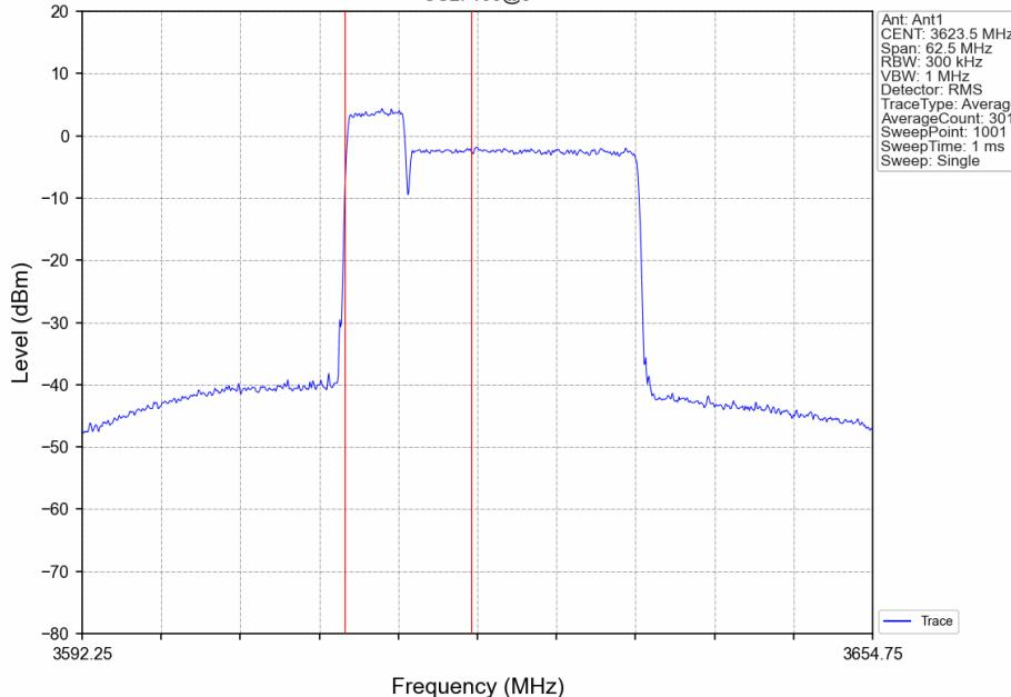
CA\_48C\_SISO\_NTNV\_CC1:5 CC2:20MHz\_CC1:16QAM CC2:16QAM\_CC1:3678.3 CC2:3690MHz\_CC1: 1@0 CC2: 1@0
