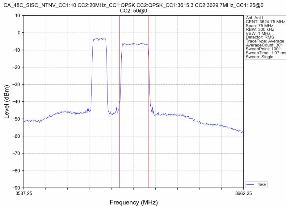
CA\_48C\_SISO\_NTNV\_CC1:10 CC2:20MHz\_CC1:QPSK CC2:QPSK\_CC1:3615.3 CC2:3629.7MHz\_CC1: 25@13 CC2: 50@25
