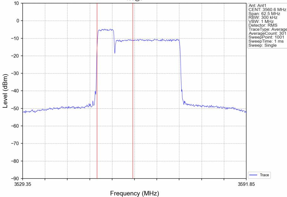
CA\_48C\_SISO\_NTNV\_CC1:5 CC2:20MHz\_CC1:QPSK CC2:QPSK\_CC1:3615.4 CC2:3627.1MHz\_CC1: 1@0 CC2: 1@0
