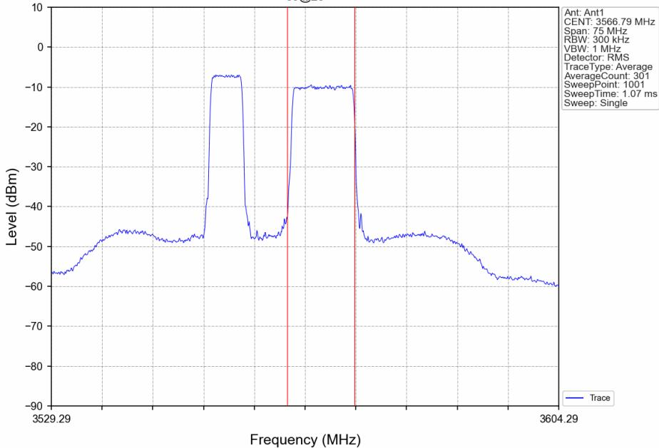
**CA\_48C\_SISO\_NTNV\_CC1:10 CC2:20MHz\_CC1:QPSK CC2:QPSK\_CC1:3555 CC2:3569.4MHz\_CC1: 25@25 CC2: 50@50**
