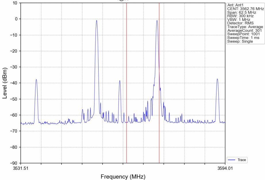
CA\_48C\_SISO\_NTNV\_CC1:5 CC2:20MHz\_CC1:QPSK CC2:QPSK\_CC1:3552.5 CC2:3564.2MHz\_CC1: 12@0 CC2: 50@0
