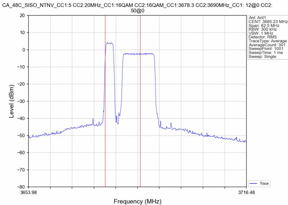
CA\_48C\_SISO\_NTNV\_CC1:5 CC2:20MHz\_CC1:16QAM CC2:16QAM\_CC1:3678.3 CC2:3690MHz\_CC1: 12@6 CC2: 50@25
