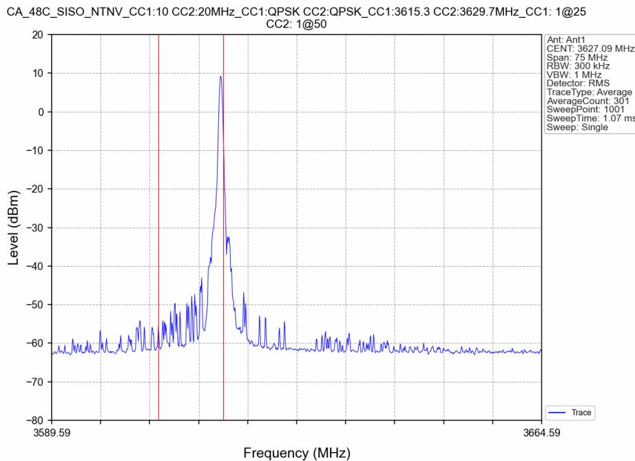
CA\_48C\_SISO\_NTNV\_CC1:10 CC2:20MHz\_CC1:QPSK CC2:QPSK\_CC1:3615.3 CC2:3629.7MHz\_CC1: 1@49 CC2: 1@99
