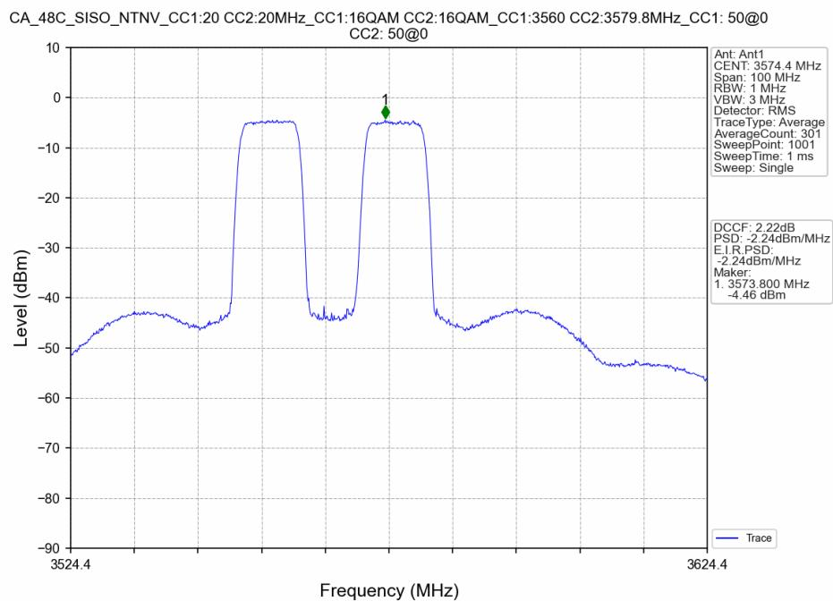
CA\_48C\_SISO\_NTNV\_CC1:20 CC2:20MHz\_CC1:16QAM CC2:16QAM\_CC1:3560 CC2:3579.8MHz\_CC1: 50@25
