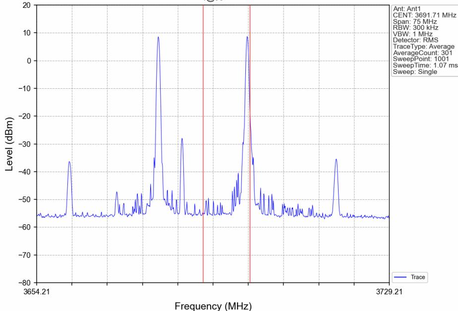
CA\_48C\_SISO\_NTNV\_CC1:10 CC2:20MHz\_CC1:QPSK CC2:QPSK\_CC1:3675.6 CC2:3690MHz\_CC1: 25@0 CC2:
