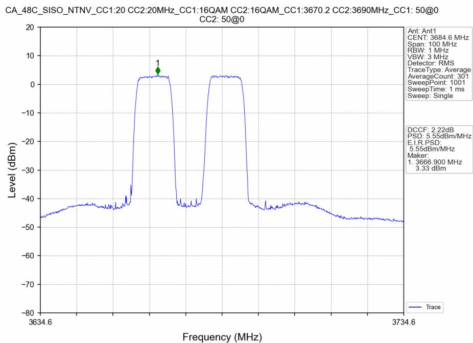
CA\_48C\_SISO\_NTNV\_CC1:20 CC2:20MHz\_CC1:16QAM CC2:16QAM\_CC1:3670.2 CC2:3690MHz\_CC1: 50@25
