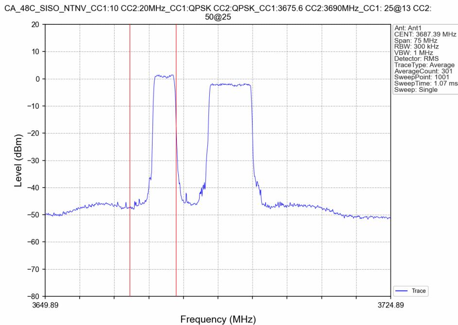
CA\_48C\_SISO\_NTNV\_CC1:10 CC2:20MHz\_CC1:QPSK CC2:QPSK\_CC1:3675.6 CC2:3690MHz\_CC1: 25@25 CC2:
