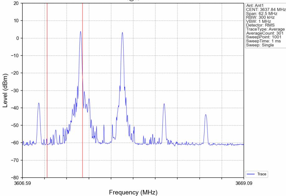
CA\_48C\_SISO\_NTNV\_CC1:20 CC2:5MHz\_CC1:QPSK CC2:QPSK\_CC1:3622.9 CC2:3634.6MHz\_CC1: 1@99 CC2: 1@24
