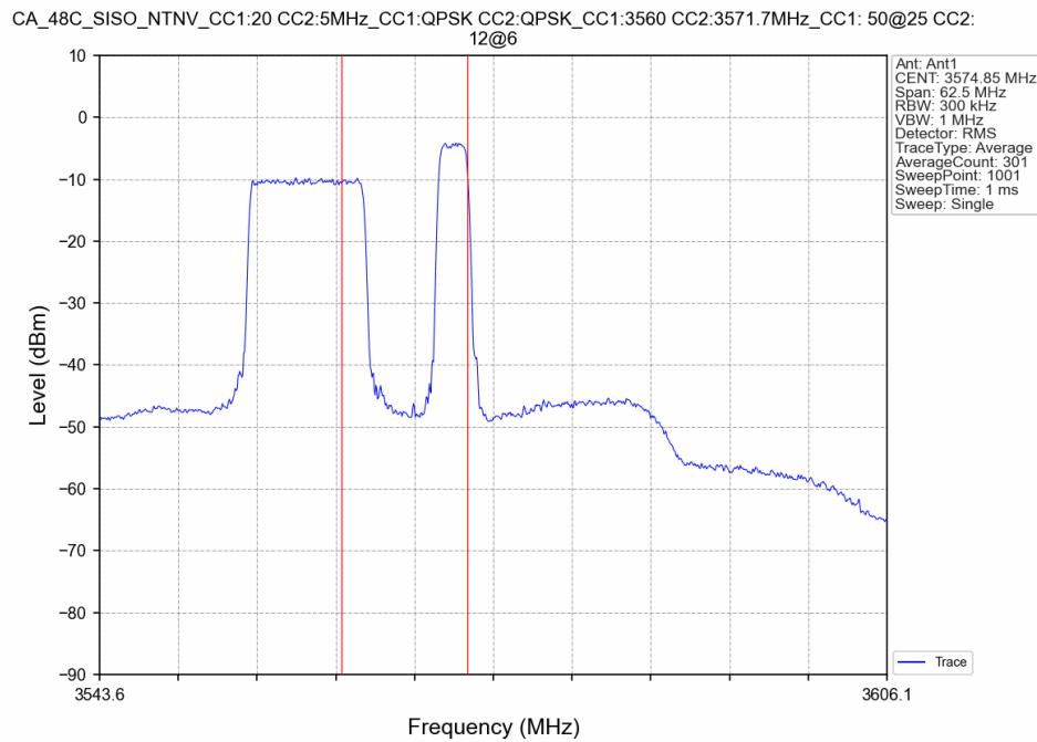
CA\_48C\_SISO\_NTNV\_CC1:20 CC2:5MHz\_CC1:QPSK CC2:QPSK\_CC1:3560 CC2:3571.7MHz\_CC1: 50@50 CC2:
