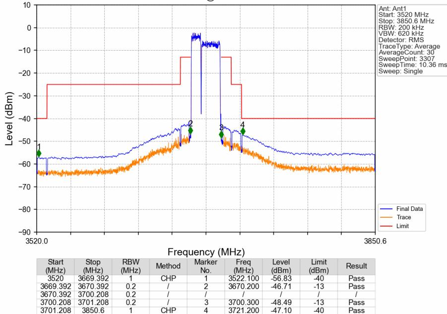
CA\_48C\_SISO\_NTNV\_CC1:10 CC2:20MHz\_CC1:QPSK CC2:QPSK\_CC1:3675.6 CC2:3690MHz\_CC1: 50@0 CC2:
