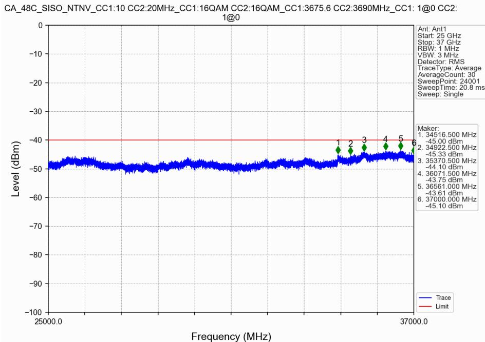
CA\_48C\_SISO\_NTNV\_CC1:10 CC2:20MHz\_CC1:16QAM CC2:16QAM\_CC1:3675.6 CC2:3690MHz\_CC1:1@49
