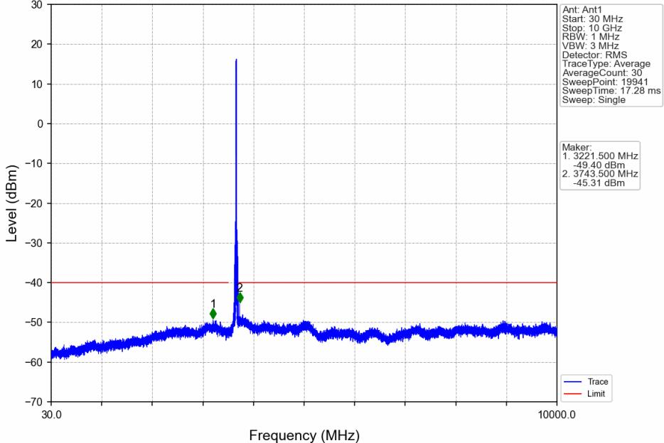
CA\_48C\_SISO\_NTNV\_CC1:10 CC2:20MHz\_CC1:QPSK CC2:QPSK\_CC1:3675.6 CC2:3690MHz\_CC1: 1@0 CC2: 1@0
