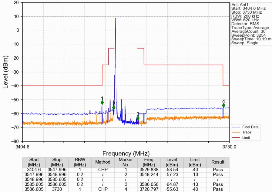
CA\_48C\_SISO\_NTNV\_CC1:15 CC2:20MHz\_CC1:16QAM CC2:16QAM\_CC1:3557.5 CC2:3574.6MHz\_CC1: 1@0
