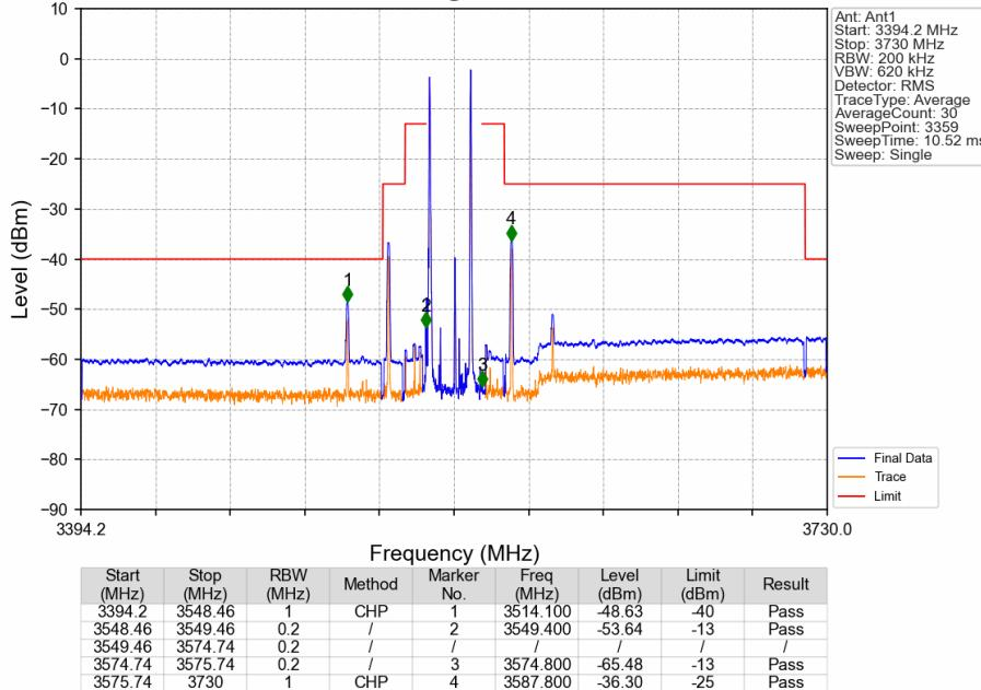
CA\_48C\_SISO\_NTNV\_CC1:20 CC2:5MHz\_CC1:16QAM CC2:16QAM\_CC1:3560 CC2:3571.7MHz\_CC1: 1@0 CC2: 1@0
