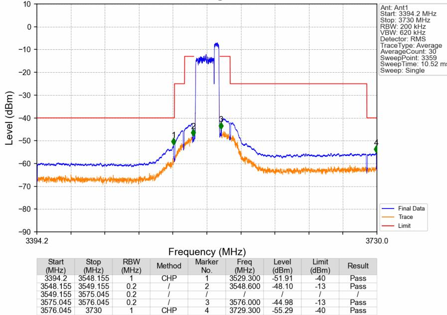
CA\_48C\_SISO\_NTNV\_CC1:20 CC2:5MHz\_CC1:16QAM CC2:16QAM\_CC1:3560 CC2:3571.7MHz\_CC1: 100@0
