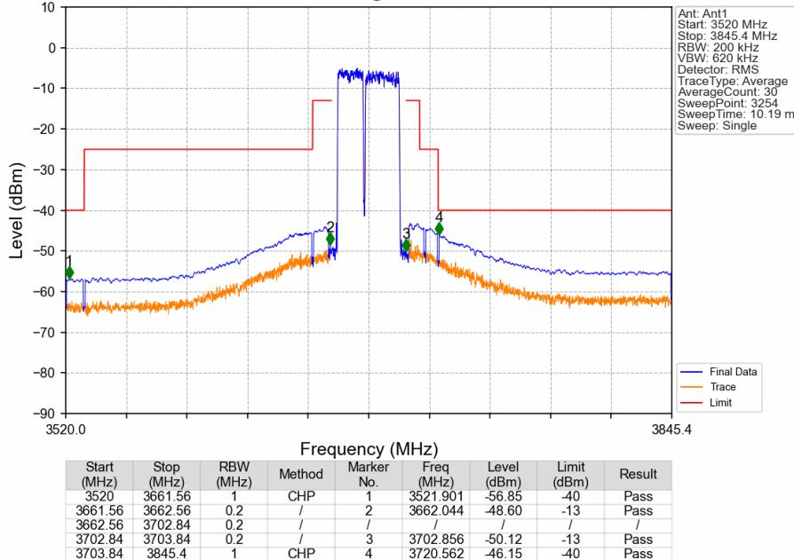
CA\_48C\_SISO\_NTNV\_CC1:15 CC2:20MHz\_CC1:QPSK CC2:QPSK\_CC1:3672.9 CC2:3690MHz\_CC1: 75@0 CC2:
