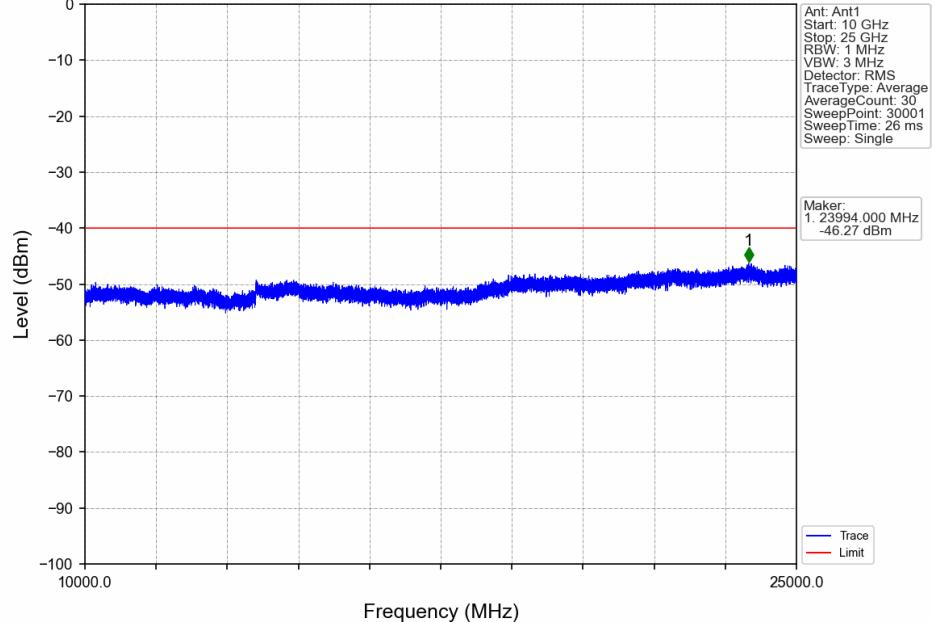
CA\_48C\_SISO\_NTNV\_CC1:20 CC2:10MHz\_CC1:QPSK CC2:QPSK\_CC1:3560 CC2:3574.4MHz\_CC1: 1@0 CC2: 1@0
