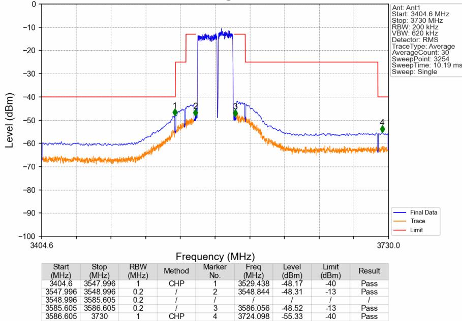
CA\_48C\_SISO\_NTNV\_CC1:20 CC2:15MHz\_CC1:16QAM CC2:16QAM\_CC1:3560 CC2:3577.1MHz\_CC1: 100@0
