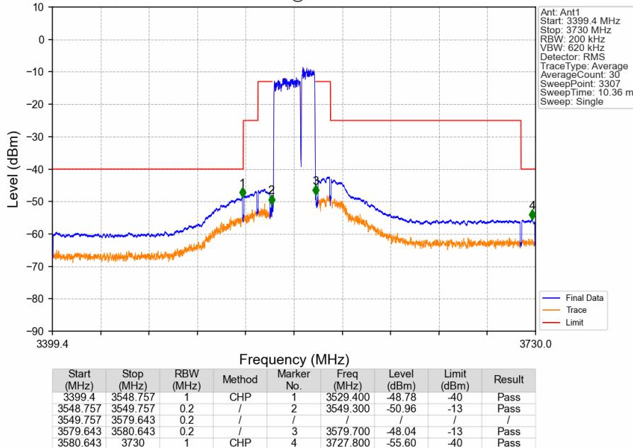
CA\_48C\_SISO\_NTNV\_CC1:20 CC2:10MHz\_CC1:QPSK CC2:QPSK\_CC1:3560 CC2:3574.4MHz\_CC1: 100@0 CC2: 50@0
