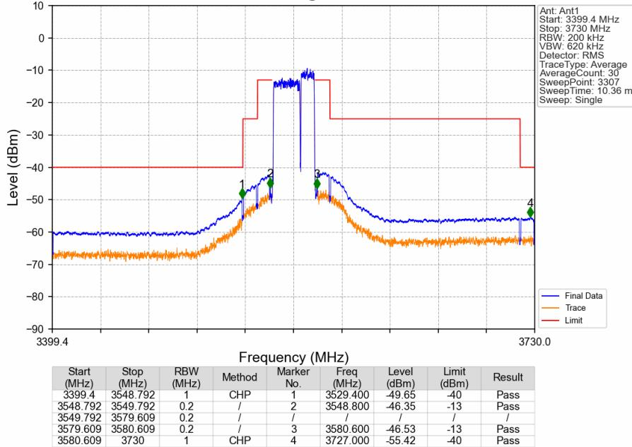
CA\_48C\_SISO\_NTNV\_CC1:20 CC2:10MHz\_CC1:16QAM CC2:16QAM\_CC1:3560 CC2:3574.4MHz\_CC1: 100@0
