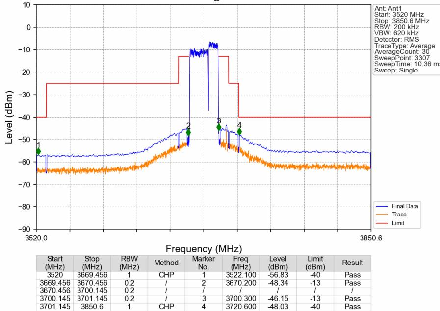
CA\_48C\_SISO\_NTNV\_CC1:20 CC2:10MHz\_CC1:16QAM CC2:16QAM\_CC1:3680.6 CC2:3695MHz\_CC1: 100@0
