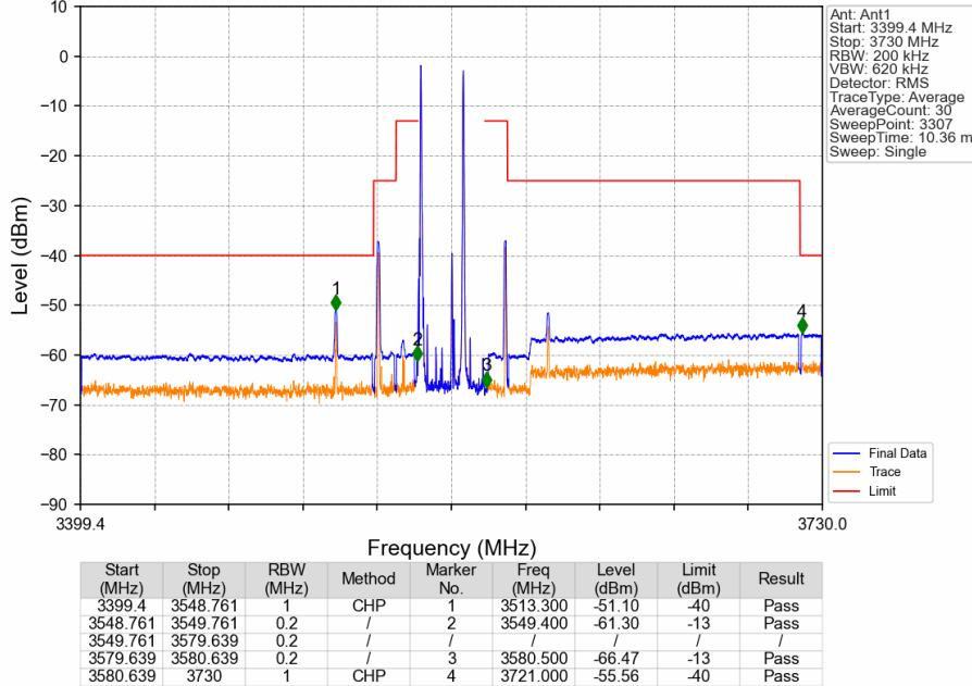
CA\_48C\_SISO\_NTNV\_CC1:20 CC2:10MHz\_CC1:QPSK CC2:QPSK\_CC1:3560 CC2:3574.4MHz\_CC1: 1@0 CC2: 1@0
