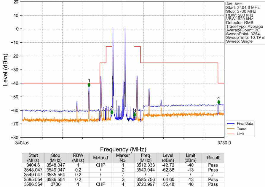
CA\_48C\_SISO\_NTNV\_CC1:20 CC2:15MHz\_CC1:16QAM CC2:16QAM\_CC1:3560 CC2:3577.1MHz\_CC1: 1@0 CC2: 1@0
