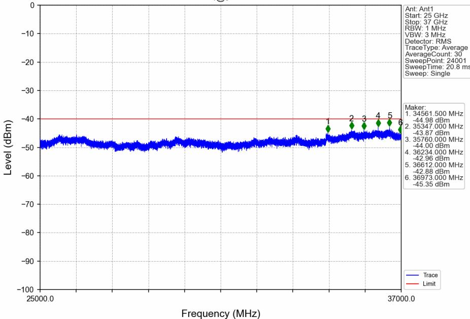
CA\_48C\_SISO\_NTNV\_CC1:20 CC2:10MHz\_CC1:16QAM CC2:16QAM\_CC1:3680.6 CC2:3695MHz\_CC1: 1@99 CC2: 1@49
