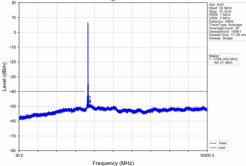
CA\_48C\_SISO\_NTNV\_CC1:20 CC2:10MHz\_CC1:16QAM CC2:16QAM\_CC1:3680.6 CC2:3695MHz\_CC1: 1@0 CC2: 1@0
