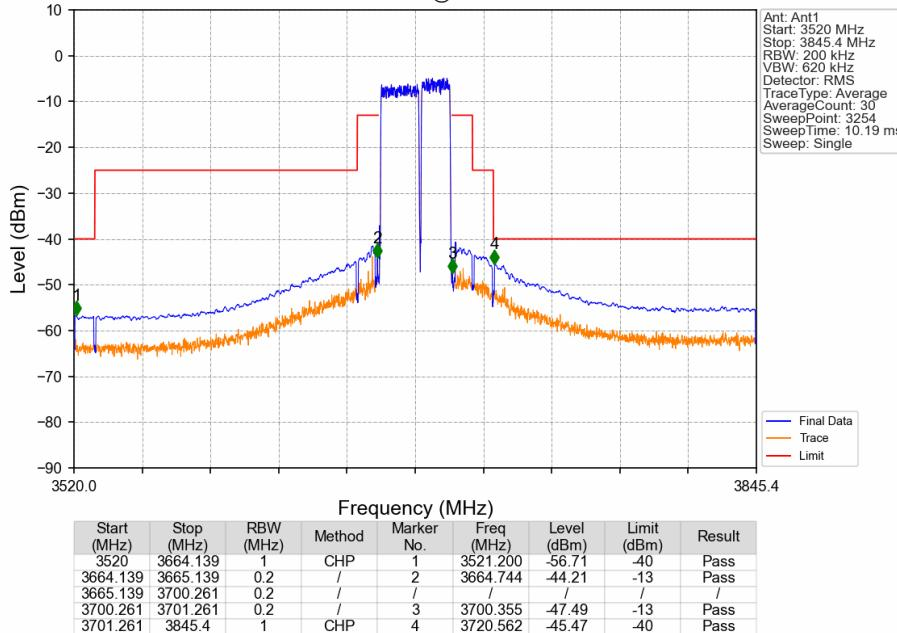
CA\_48C\_SISO\_NTNV\_CC1:20 CC2:15MHz\_CC1:16QAM CC2:16QAM\_CC1:3675.4 CC2:3692.5MHz\_CC1: 100@0
