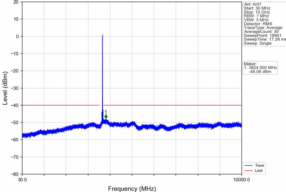
CA\_48C\_SISO\_NTNV\_CC1:20 CC2:15MHz\_CC1:16QAM CC2:16QAM\_CC1:3675.4 CC2:3692.5MHz\_CC1: 1@0
