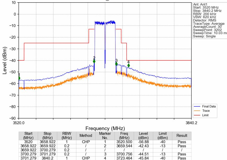
CA\_48C\_SISO\_NTNV\_CC1:20 CC2:20MHz\_CC1:QPSK CC2:QPSK\_CC1:3670.2 CC2:3690MHz\_CC1: 100@0 CC2: 100@0
