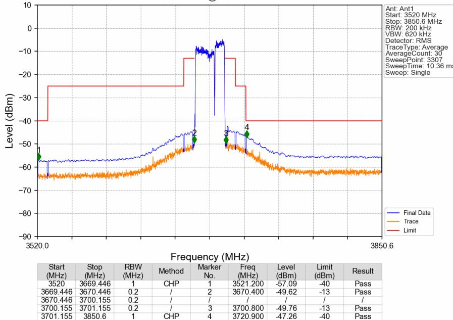
CA\_48C\_SISO\_NTNV\_CC1:20 CC2:10MHz\_CC1:QPSK CC2:QPSK\_CC1:3680.6 CC2:3695MHz\_CC1: 100@0 CC2: 50@0
