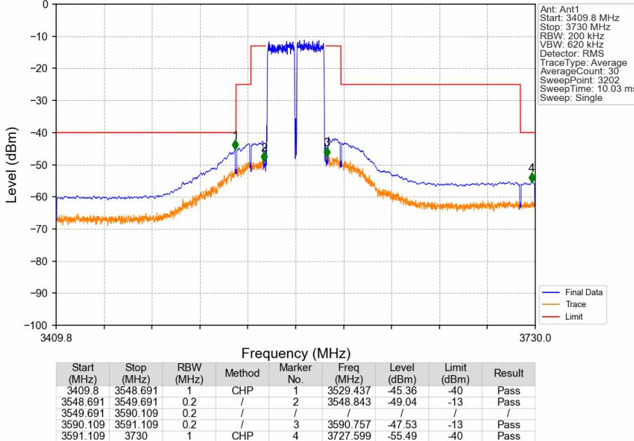
CA\_48C\_SISO\_NTNV\_CC1:20 CC2:20MHz\_CC1:QPSK CC2:QPSK\_CC1:3560 CC2:3579.8MHz\_CC1: 100@0 CC2: 100@0
