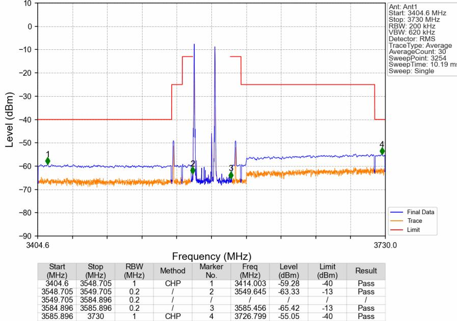
CA\_48C\_SISO\_NTNV\_CC1:20 CC2:15MHz\_CC1:QPSK CC2:QPSK\_CC1:3560 CC2:3577.1MHz\_CC1: 1@0 CC2: 1@0
