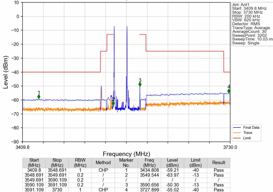
CA\_48C\_SISO\_NTNV\_CC1:20 CC2:20MHz\_CC1:QPSK CC2:QPSK\_CC1:3560 CC2:3579.8MHz\_CC1: 1@0 CC2: 1@0
