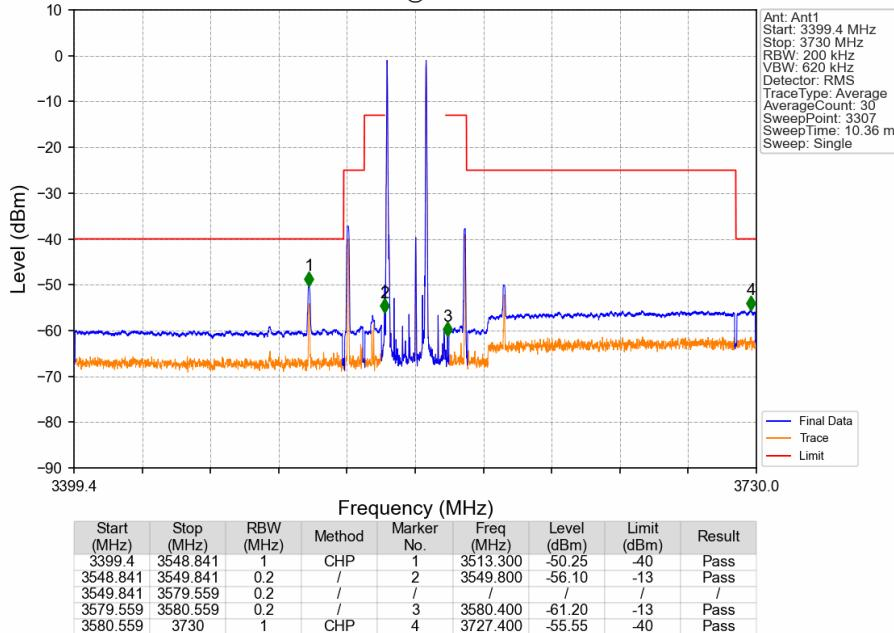
CA\_48C\_SISO\_NTNV\_CC1:20 CC2:10MHz\_CC1:16QAM CC2:16QAM\_CC1:3560 CC2:3574.4MHz\_CC1: 1@0 CC2: 1@0
