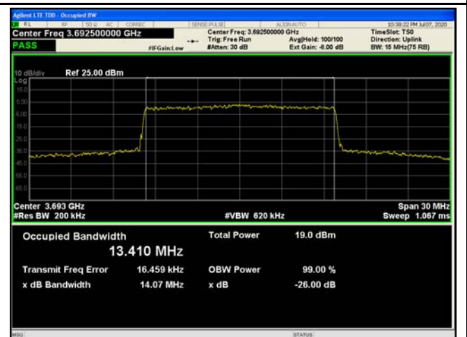
15MHz - High CH 16QAM
