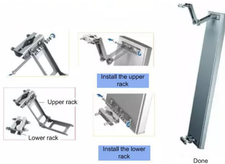
Figure 3-9 Assembling Procedure of Directional Antennas
