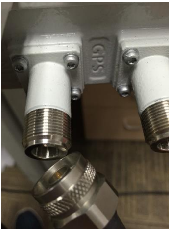
Figure 3-18 GPS Connector Connect to Base Station
