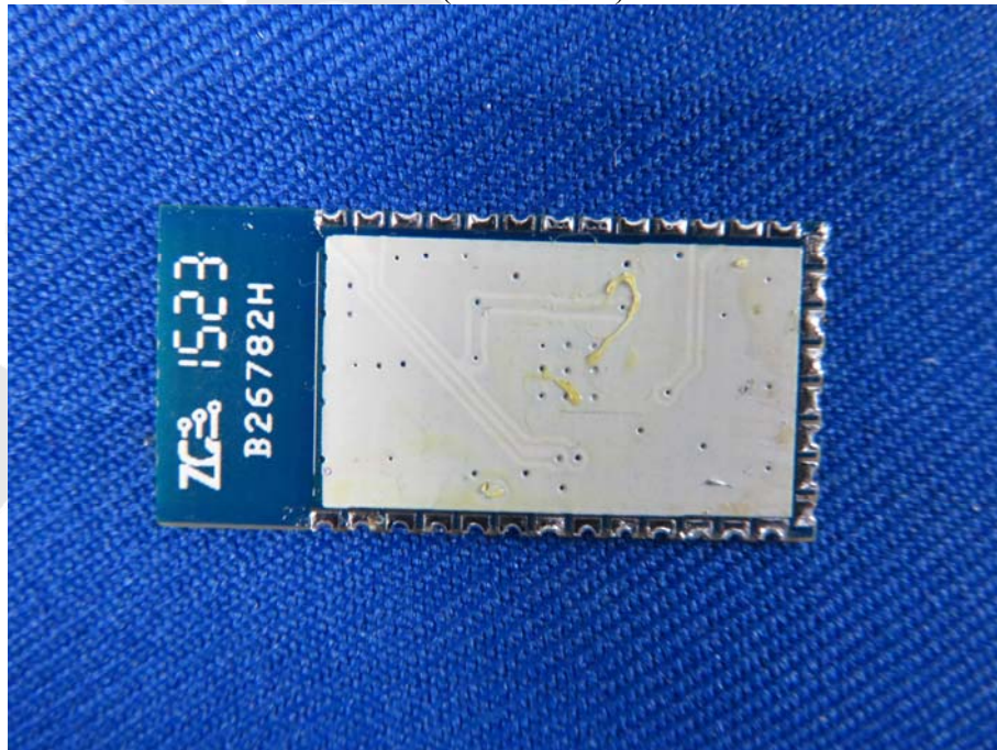
Figure 19 PCB of The EUT- Back View (BT Module)
