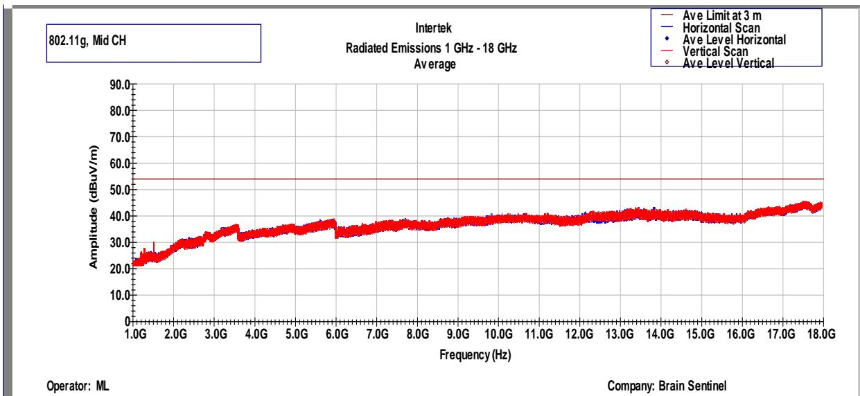
Note: Radiated emission measurements were performed up to 25GHz. No Emissions were identified when scanned from 18-25 GHz
