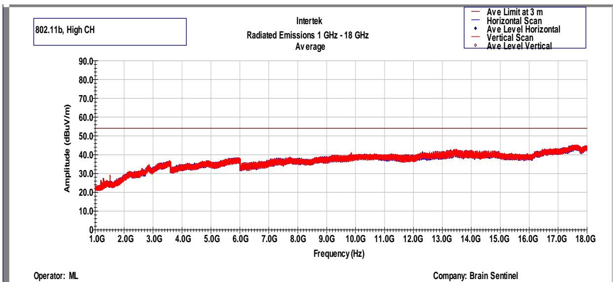
Note: Radiated emission measurements were performed up to 25GHz. No Emissions were identified when scanned from 18-25 GHz
