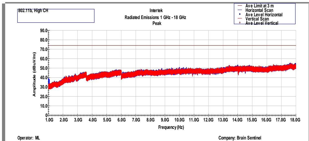
Out-of-Band Radiated Spurious Emissions (Cabinet Radiation) - 1 GHz to 18 GHz, Average
