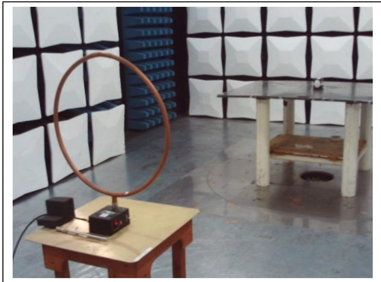
**Radiated Emissions: 30 MHz to 1000 MHz**
