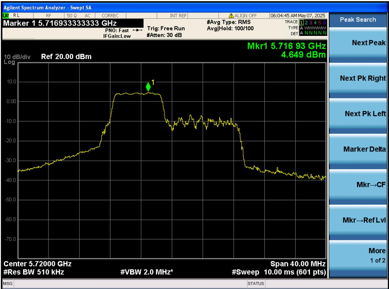
4.5. A.4-RMS Power Spectral Density (PSD)(RU106+26)
