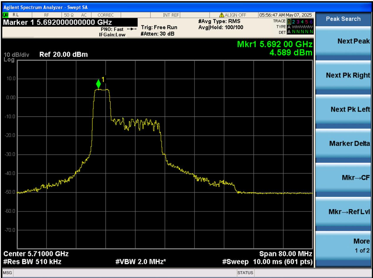
2.4. A.4-RMS Power Spectral Density (PSD)(RU242)
