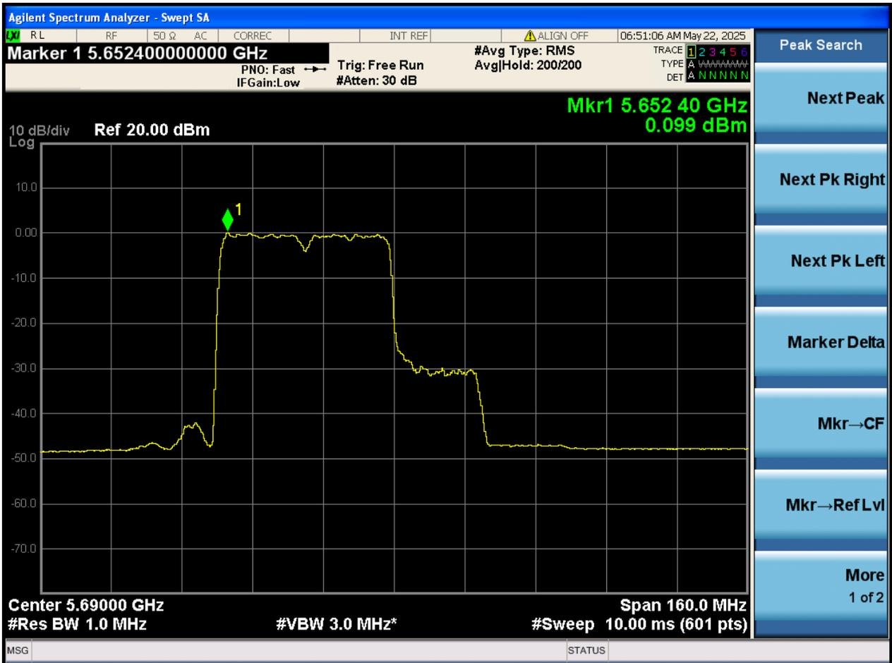
6.12. A.4-RMS Power Spectral Density (PSD)(RU52+26)
