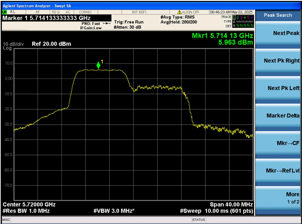
4.9. A.4-RMS Power Spectral Density (PSD)(RU52+26)
