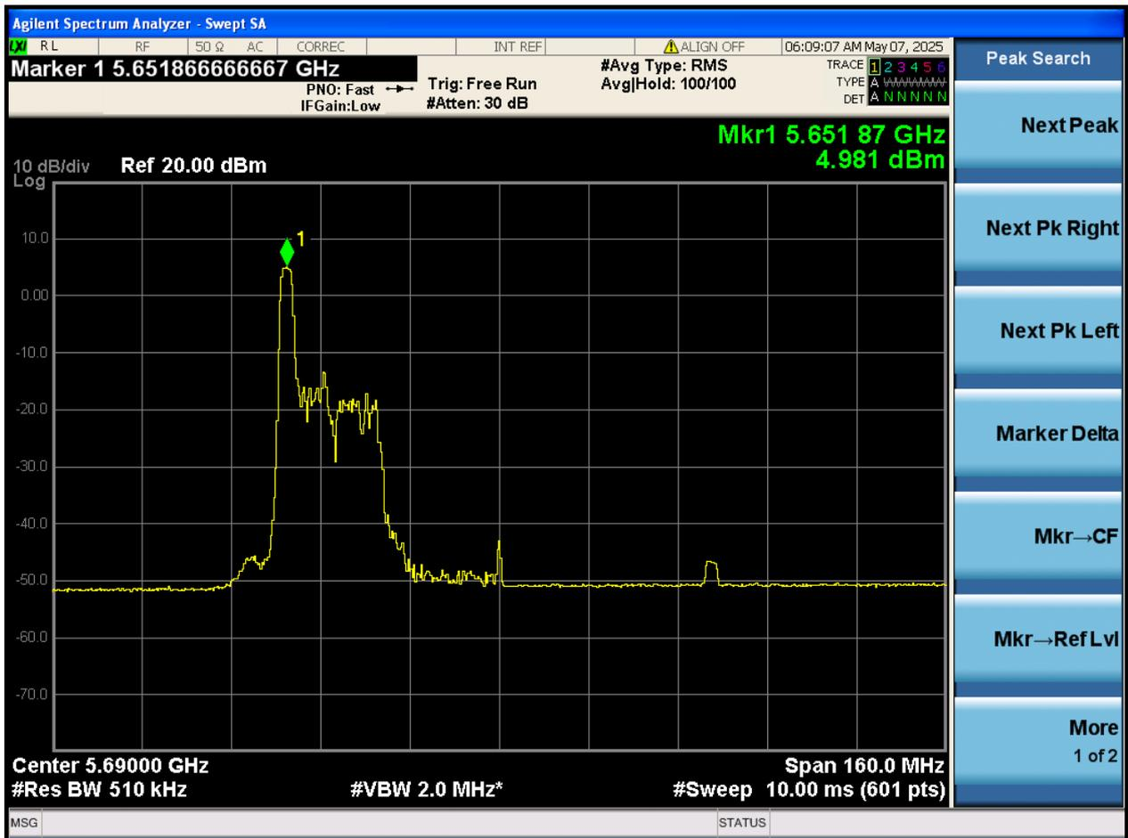
6.2. A.4-RMS Power Spectral Density (PSD)(RU52)
