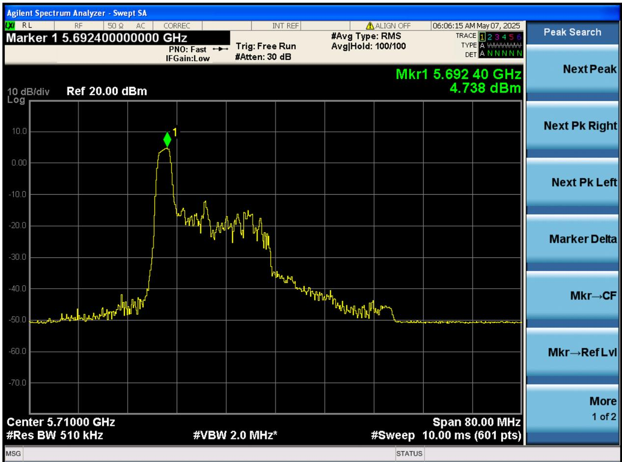
5.2. A.4-RMS Power Spectral Density (PSD)(RU52)
