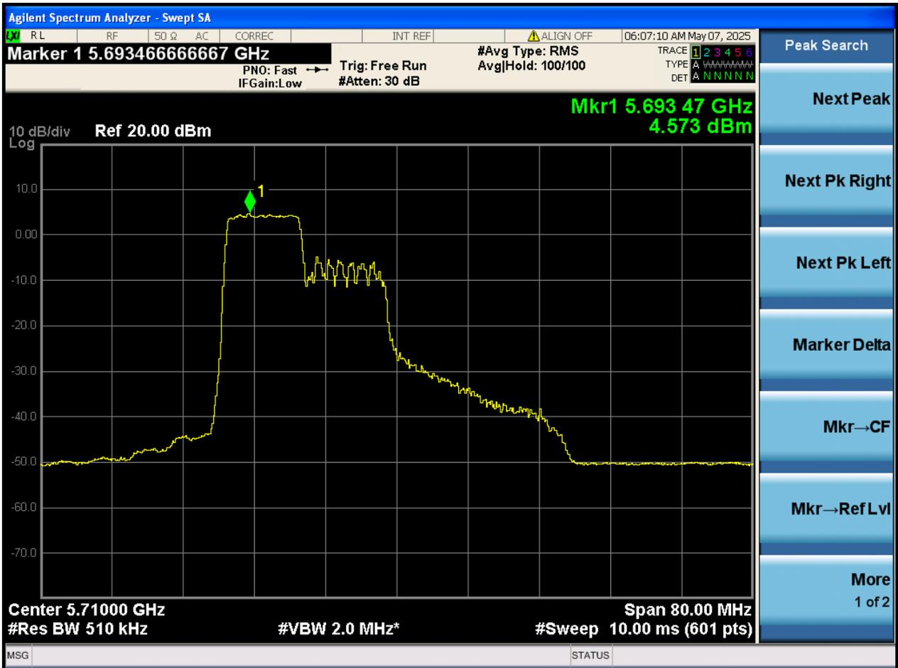
5.5. A.4-RMS Power Spectral Density (PSD)(RU52+26)
