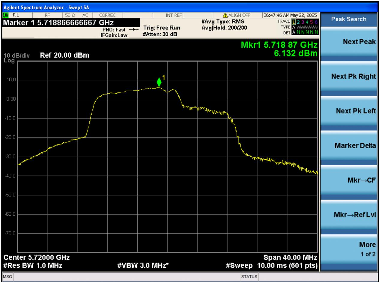
4.10. A.4-RMS Power Spectral Density (PSD)(RU106+26)
