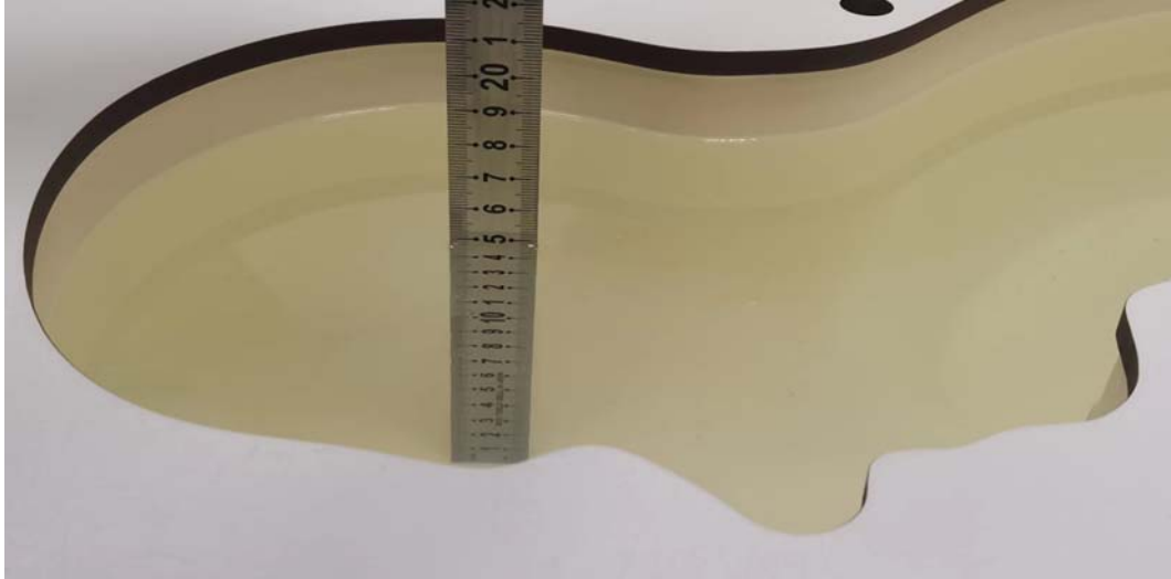
Picture 3: liquid depth in the head Phantom
