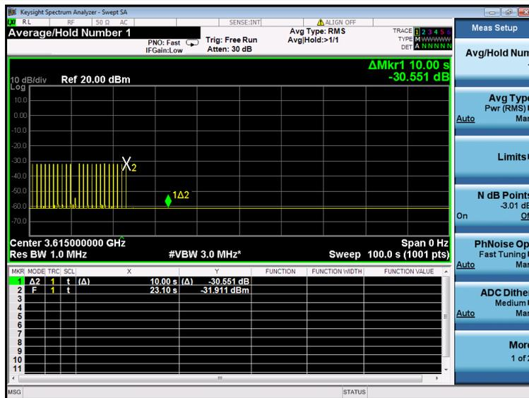
Test Band: CBSD transmit at frequency 3670-3690MHz of n48
