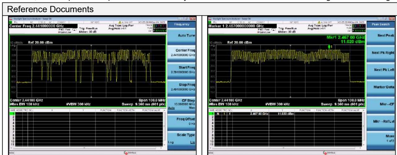
3. Channels are classified into two categories, used and unused, where used channels are part of the hopping sequence and unused channels are replaced in the hopping sequence by used channels in a pseudo-random way. Make each individual EUT meets the requirement that each of its hopping channels is used equally on average.
