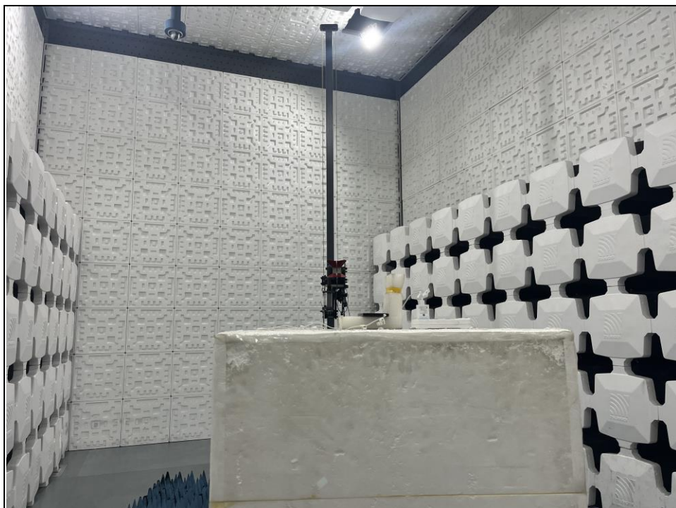
Radiated emission test: Frequency Range< 9KHz- 30MHz >
