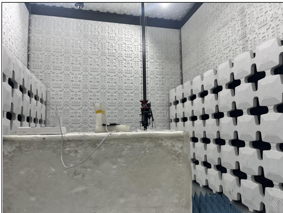
Radiated emission test: Frequency Range< Above 1GHz >
