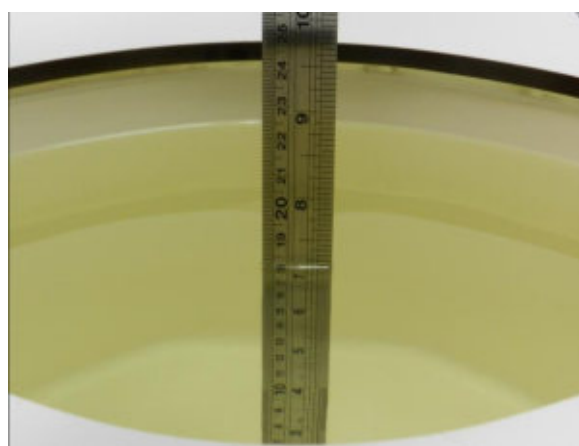
Fig 11.2 Photo of Liquid Height for Body SAR
