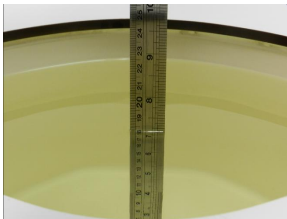
Fig 11.1 Photo of Liquid Height for Body SAR
