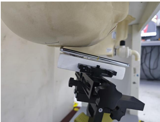
Right Tilted, Test Separation 0 mm
