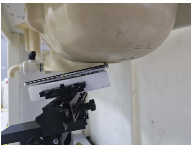
Left Tilted, Test Separation 0 mm
