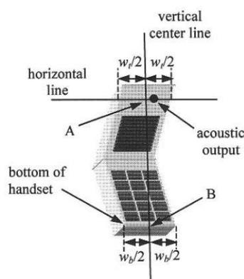
Fig 12.2.2 Handset vertical and horizontal reference lines—“clam-shell case”
