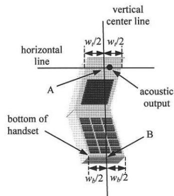
Fig 12.2.2 Handset vertical and horizontal reference lines—“clam-shell case”
