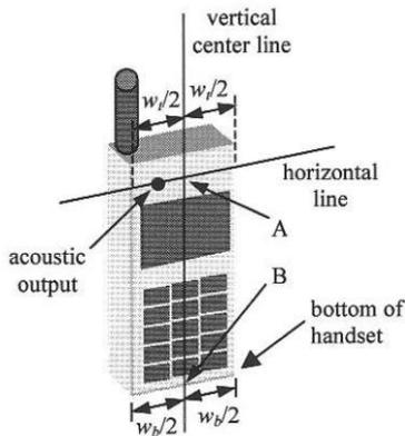
Fig 12.2.1 Handset vertical and horizontal reference lines—“fixed case”
