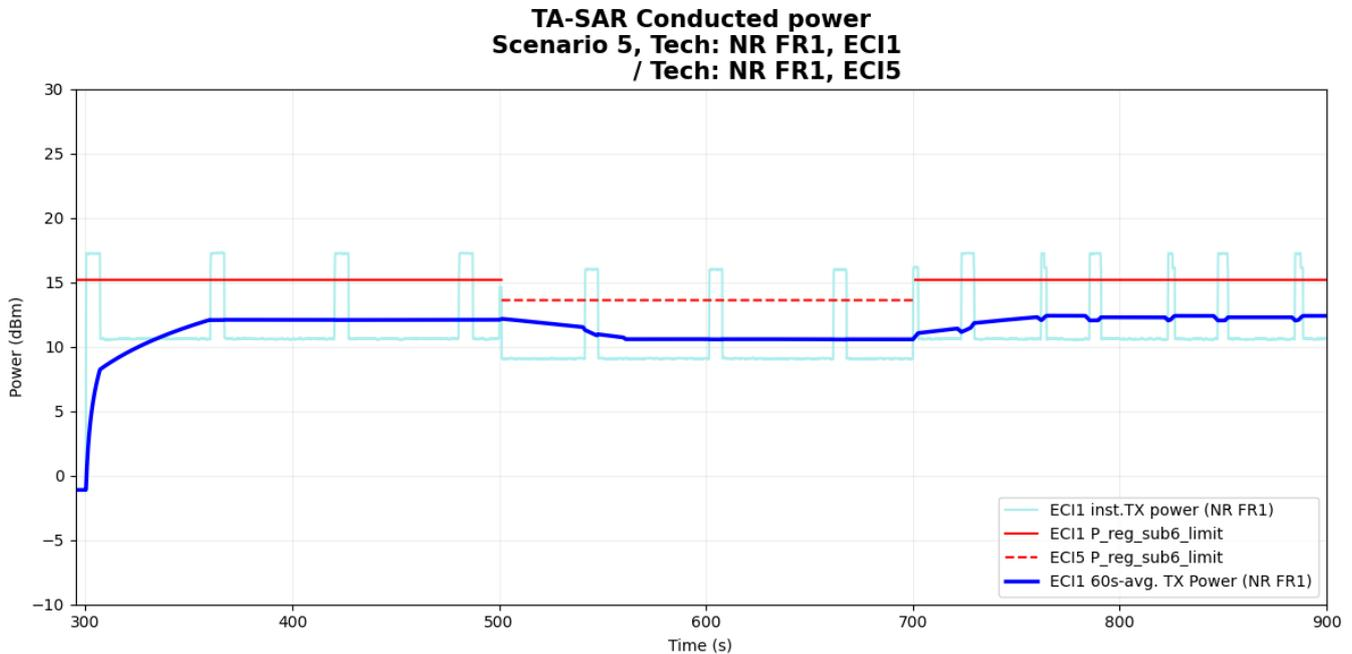
**Figure 5-45 Time-averaged conducted TX power over time for case 20 (sub6 NR ECI1, ECI5)**
