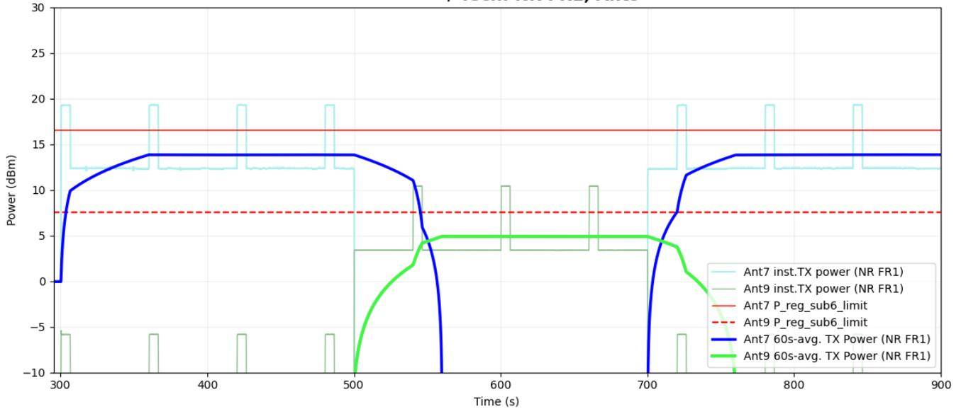
**Figure 5-47 Time-averaged conducted TX power over time for case 21 (sub6 NR n7, n9)**
