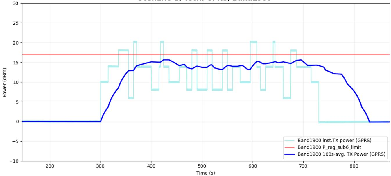
**Figure 5-39 Time-averaged conducted TX power over time for case 11 (2G GPRS 1900 2Tx)**
