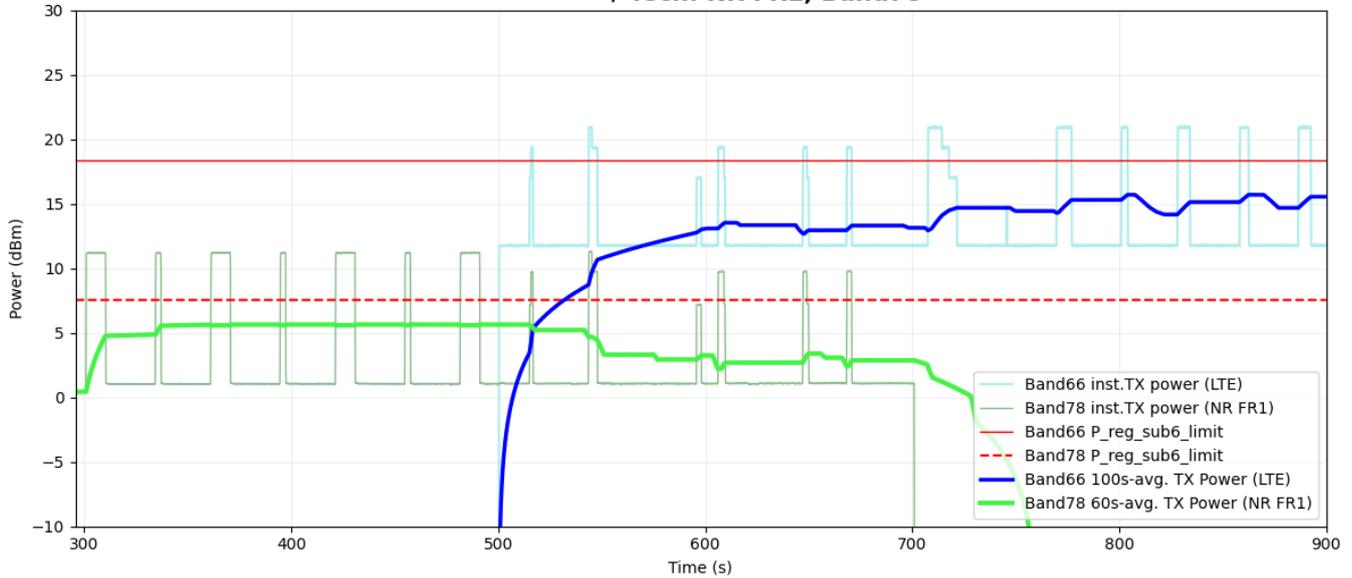
**Figure 5-55 Time-averaged conducted TX power over time for case 25 (LTE B66, sub6 NR n78)**
