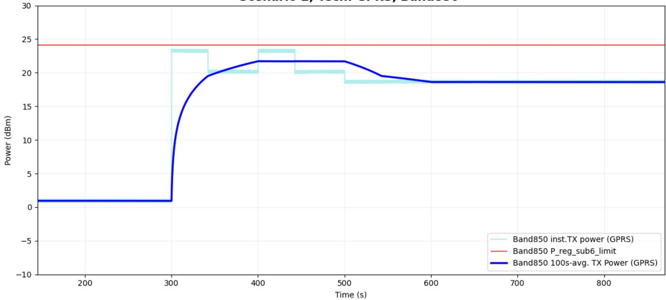
**Figure 5-33 Time-averaged conducted TX power over time for case 2 (2G GPRS 850 1TX)**
