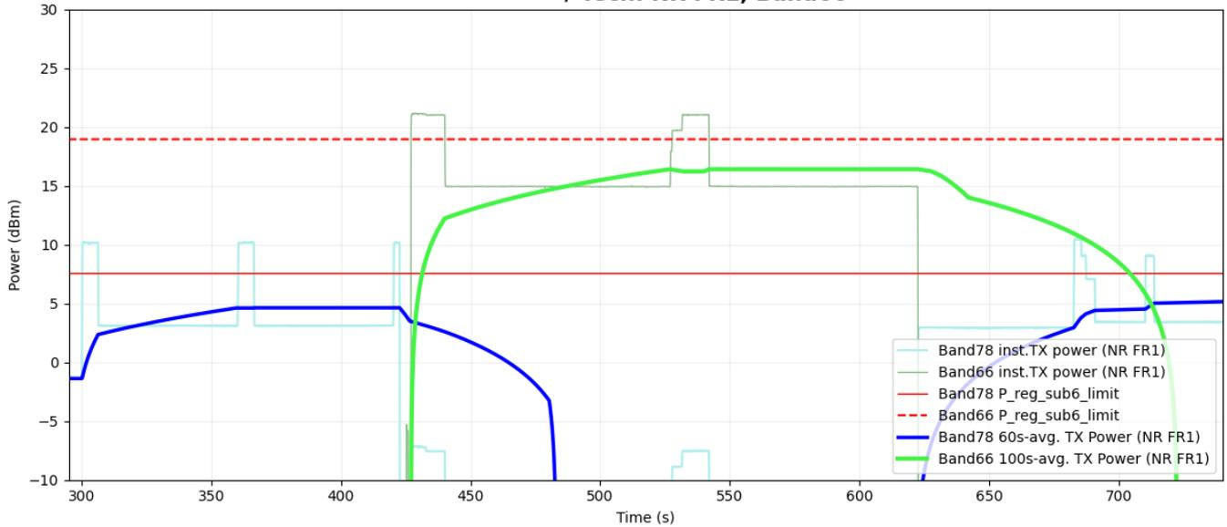
**Figure 5-49 Time-averaged conducted TX power over time for case 22 (sub6 NR n78 and n66)**
