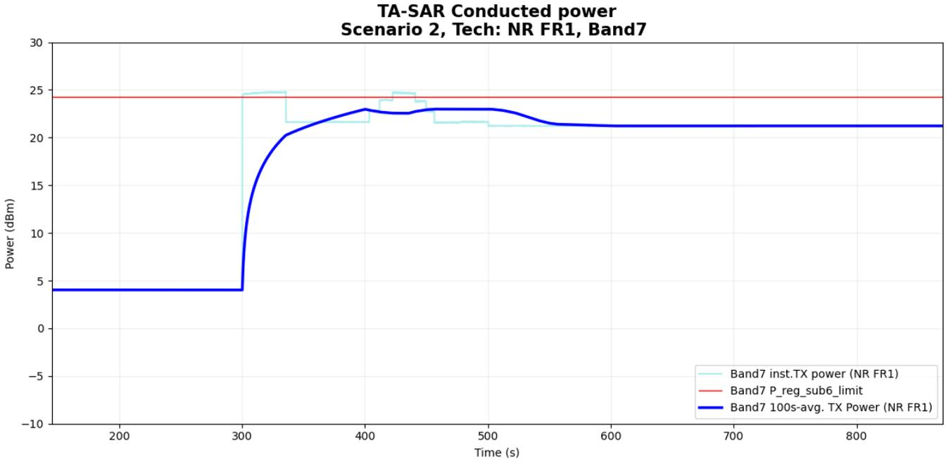
**Figure 5-9 Time-averaged conducted TX power over time for case 8 (sub6 NR n7)**
