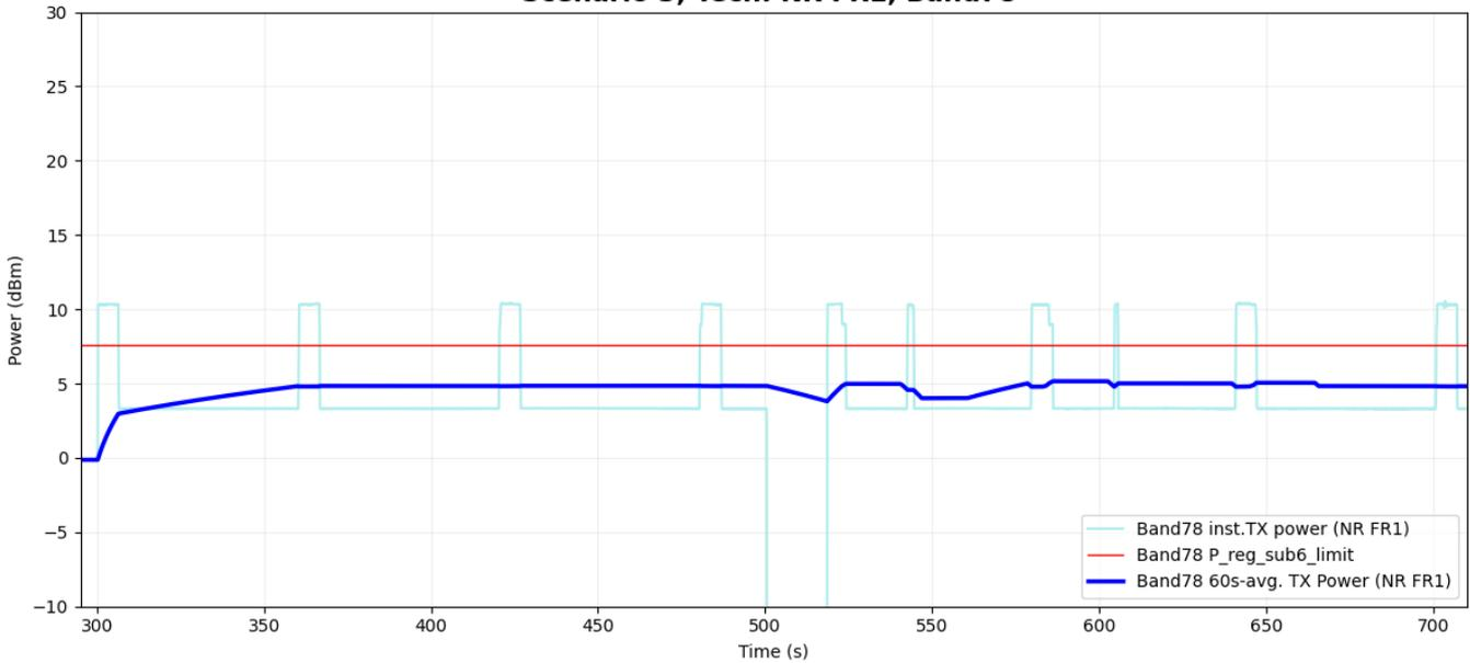
**Figure 5-41 Time-averaged conducted TX power over time for case 18 (sub6 NR n78)**
