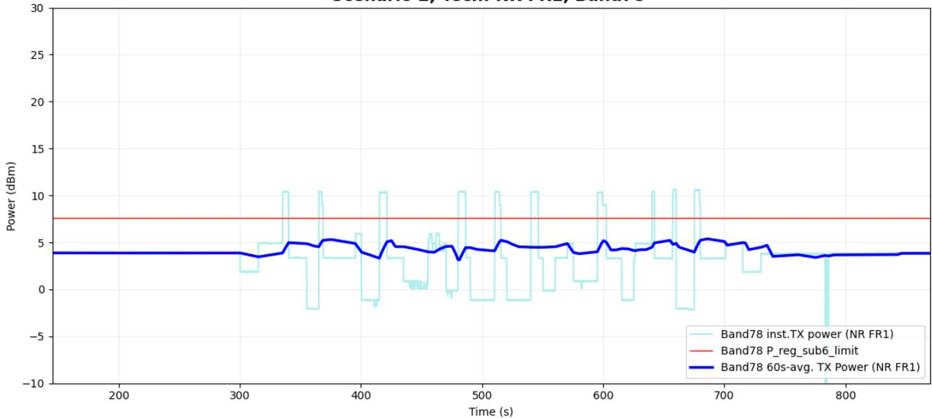
**Figure 5-15 Time-averaged conducted TX power over time for case 17 (sub6 NR n78)**
