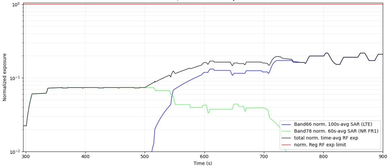
**Figure 5-56 Normalized time-averaged SAR for case 25 (LTE B66, sub6 NR n78)**
