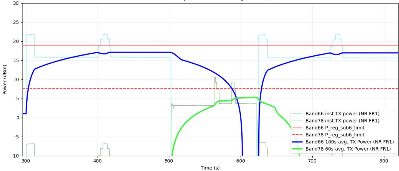
**Figure 5-51 Time-averaged conducted TX power over time for case 23 (sub6 NR n66 and n78)**
