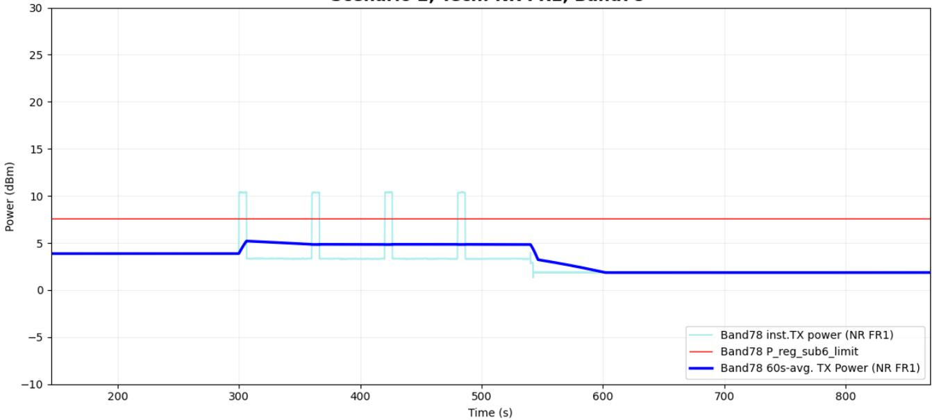
**Figure 5-11 Time-averaged conducted TX power over time for case 9 (sub6 NR n78)**
