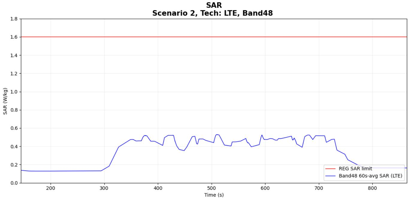
**Figure 6-9 Time-averaged SAR for case 15 in table 6-1 (LTE B48)**
