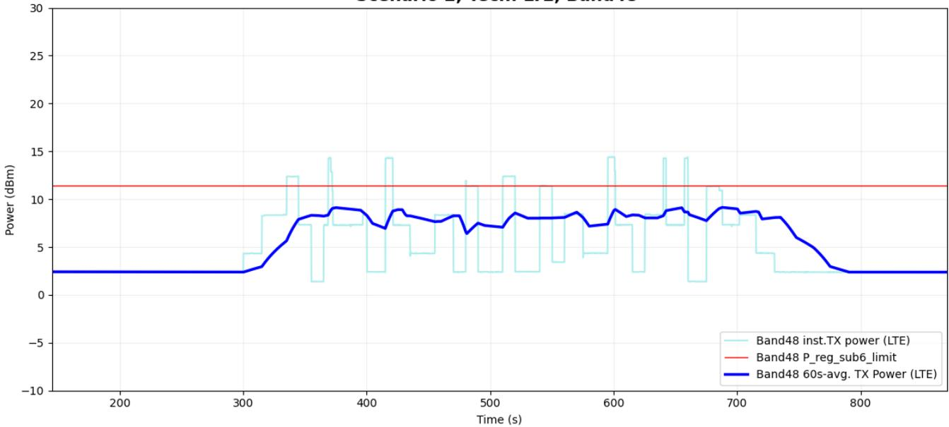
**Figure 5-23 Time-averaged conducted TX power over time for case 15 (LTE B48)**
