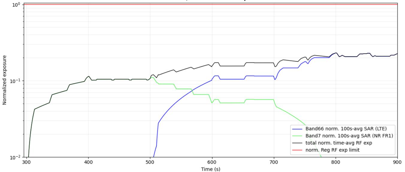
**Figure 5-54 Normalized time-averaged SAR for case 24 (LTE B66, sub6 NR n7)**
