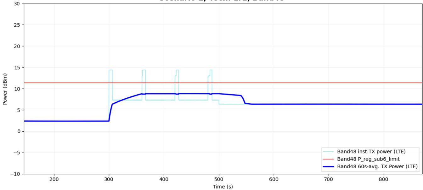
**Figure 5-19 Time-averaged conducted TX power over time for case 7 (LTE B48)**
