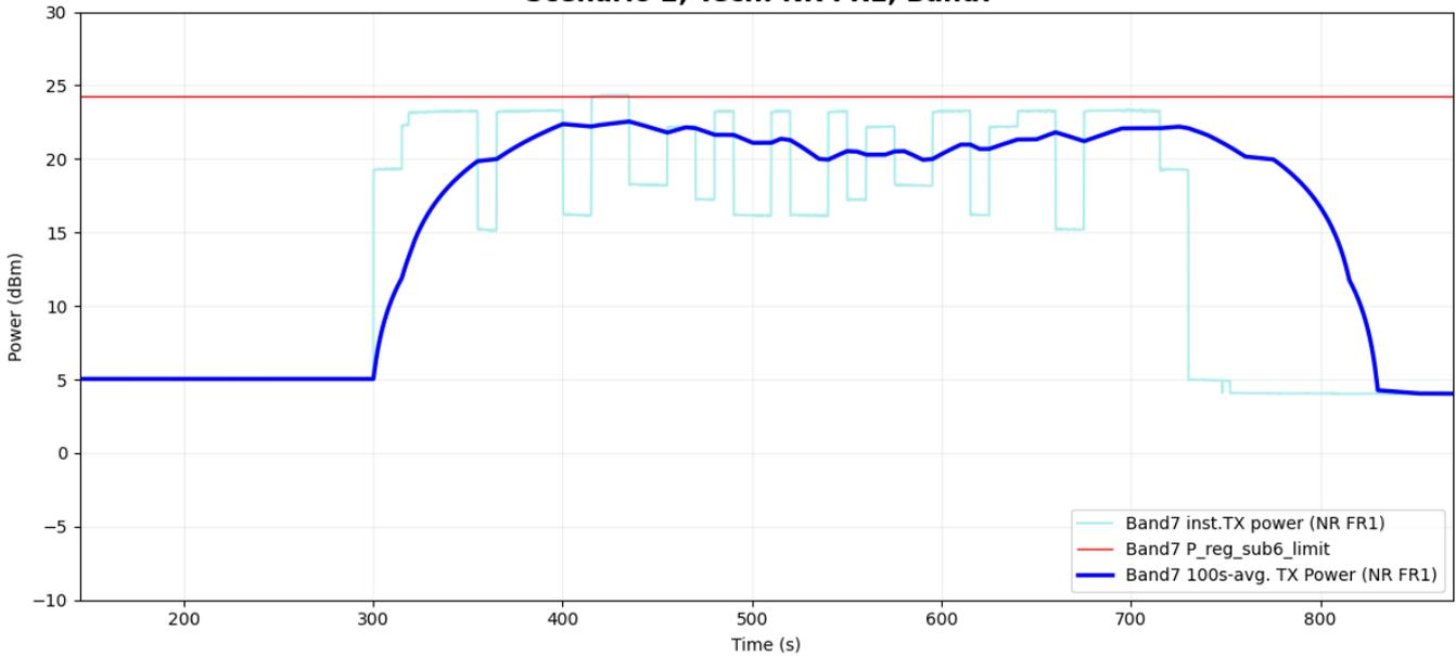
**Figure 5-13 Time-averaged conducted TX power over time for case 16 (sub6 NR n7)**
