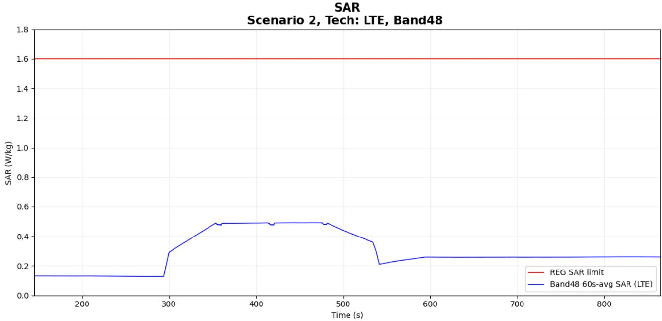
**Figure 6-7 Time-averaged SAR for case 7 in table 6-1 (LTE B48)**
