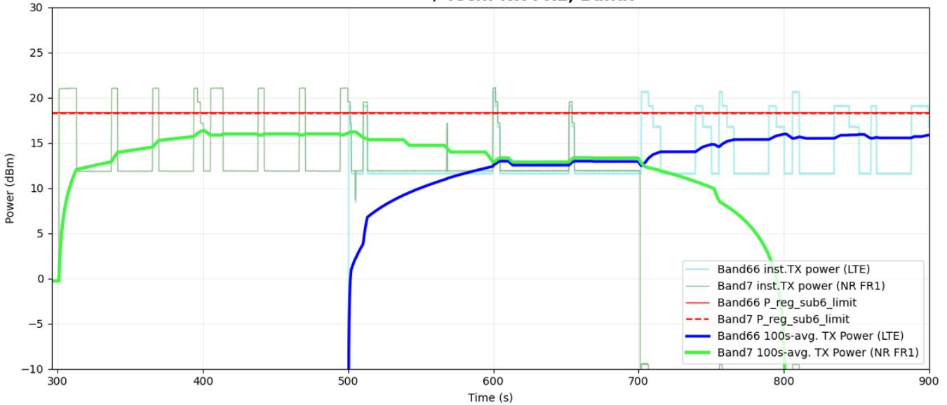
**Figure 5-53 Time-averaged conducted TX power over time for case 24 (LTE B66, sub6 NR n7)**
