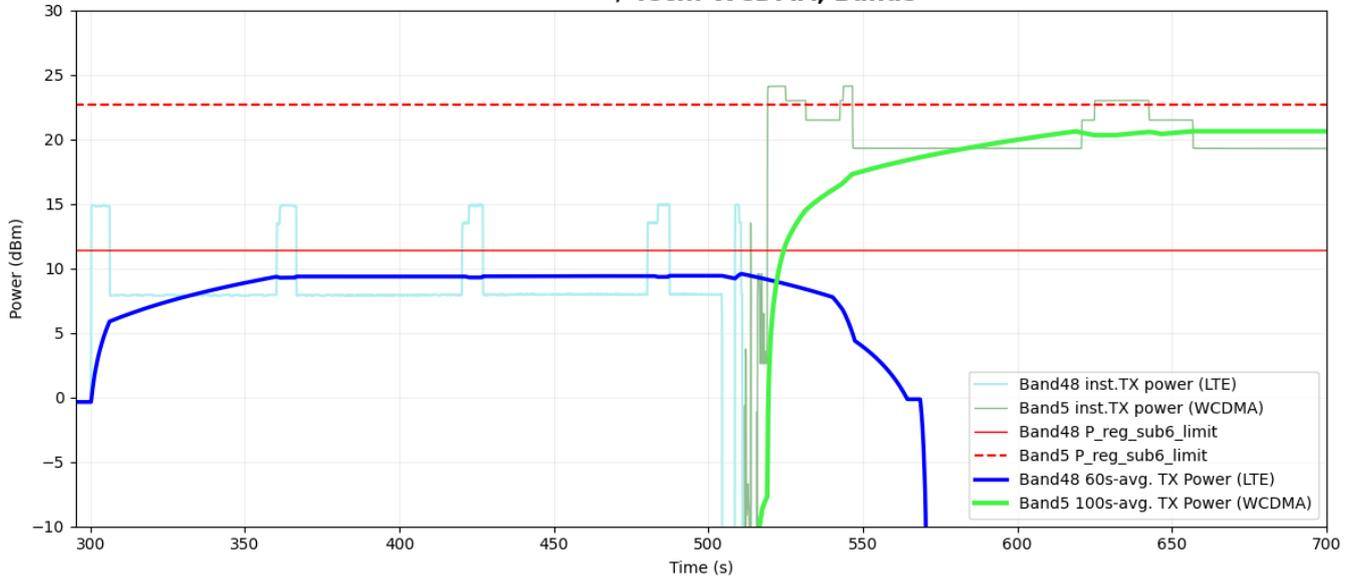
**Figure 5-43 Time-averaged conducted TX power over time for case 19 (WCDMA B5, LTE B48)**
