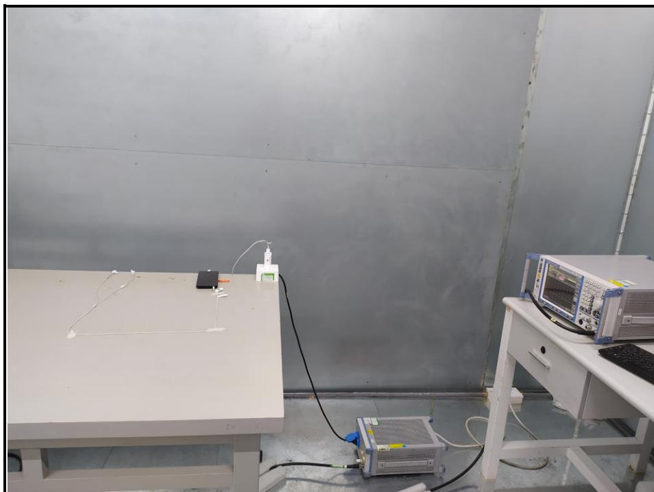
Fig. 3 Power line conducted emission setup photo
