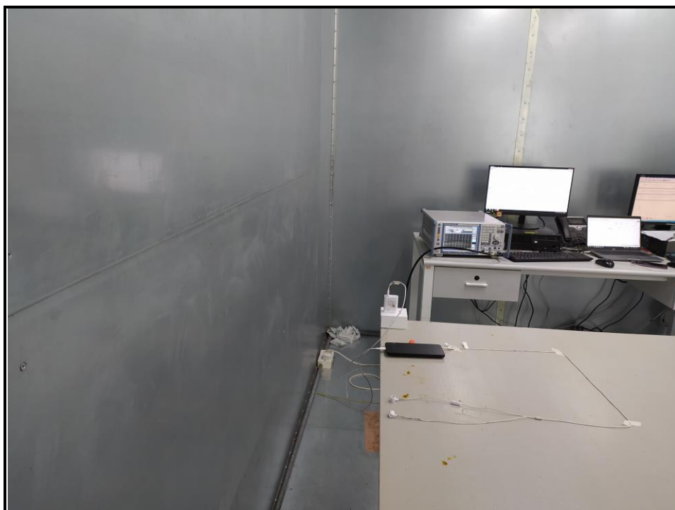
Fig. 4 Power line conducted emission setup photo
