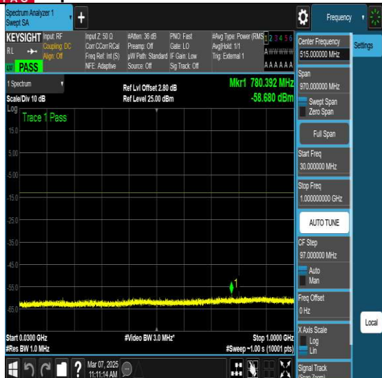
NTNV-N77-3450-3550-PC2-30-40-H-DFT-QPSK- Edge 1RB Left-Ant1-PASS
