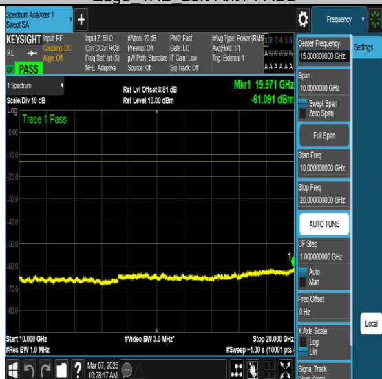
NTNV-N77-3450-3550-PC2-30-15-H-DFT-QPSK- Edge 1RB Left-Ant1-PASS
