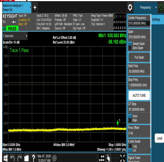
NTNV-N77-3450-3550-PC2-30-15-H-DFT-QPSK- Edge 1RB Left-Ant1-PASS
