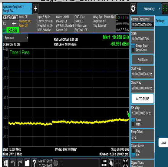
NTNV-N77-3450-3550-PC2-30-40-H-DFT-QPSK- Edge 1RB Left-Ant1-PASS
