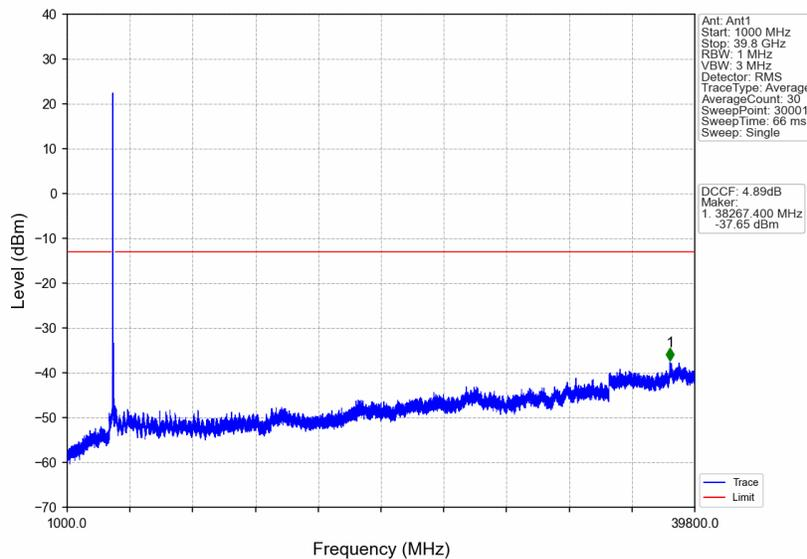
n77a\_15kHz\_SISO\_NTNV\_50MHz\_DFT-s-OFDM PI/2 BPSK\_3954.99MHz\_Edge\_1RB\_Right
