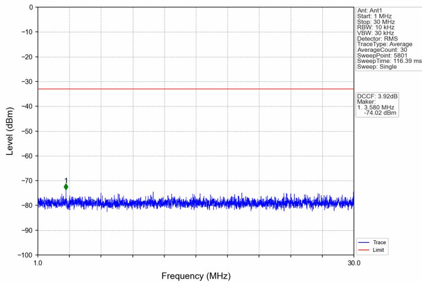
n77a\_15kHz\_SISO\_NTNV\_40MHz\_DFT-s-OFDM PI/2 BPSK\_3720MHz\_Edge\_1RB\_Left
