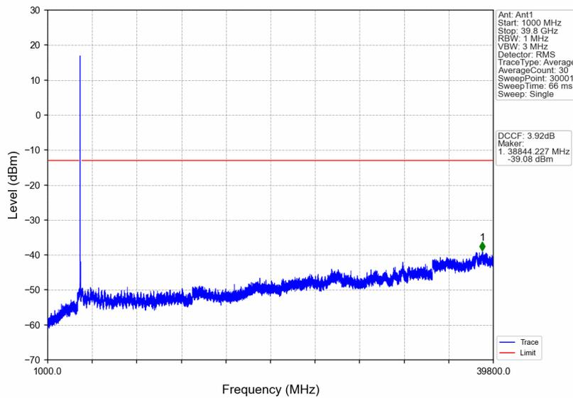
n77a\_15kHz\_SISO\_NTNV\_40MHz\_DFT-s-OFDM PI/2 BPSK\_3960MHz\_Edge\_1RB\_Right
