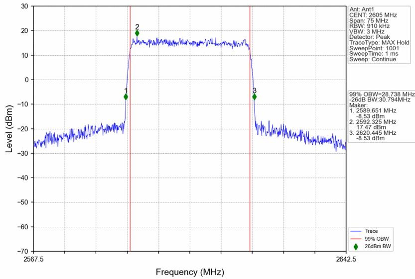
n38\_15kHz\_SISO\_NTNV\_30MHz\_CP-OFDM 64 QAM\_2585MHz\_Outer\_Full
