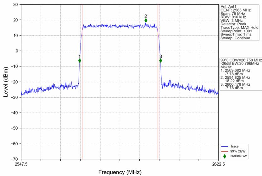
n38\_15kHz\_SISO\_NTNV\_30MHz\_DFT-s-OFDM 16 QAM\_2595MHz\_Outer\_Full
