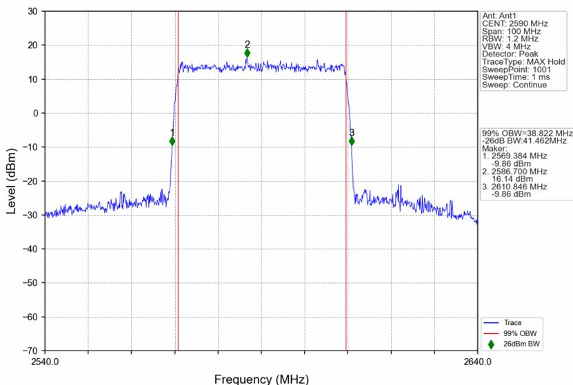
n38\_15kHz\_SISO\_NTNV\_40MHz\_DFT-s-OFDM 256 QAM\_2595MHz\_Outer\_Full
