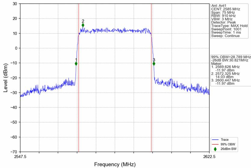
n38\_15kHz\_SISO\_NTNV\_30MHz\_CP-OFDM 256 QAM\_2595MHz\_Outer\_Full
