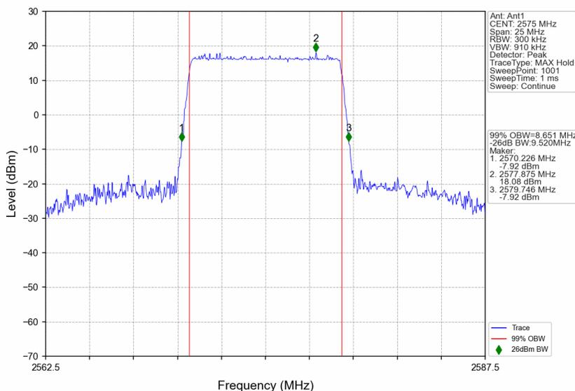
n38\_30kHz\_SISO\_NTNV\_10MHz\_DFT-s-OFDM 16 QAM\_2595MHz\_Outer\_Full
