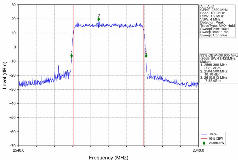
n38\_15kHz\_SISO\_NTNV\_40MHz\_CP-OFDM 16 QAM\_2595MHz\_Outer\_Full
