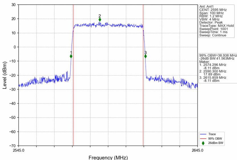
n38\_15kHz\_SISO\_NTNV\_40MHz\_DFT-s-OFDM 64 QAM\_2600MHz\_Outer\_Full
