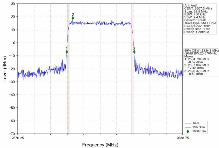
n38\_15kHz\_SISO\_NTNV\_25MHz\_CP-OFDM 64 QAM\_2582.5MHz\_Outer\_Full
