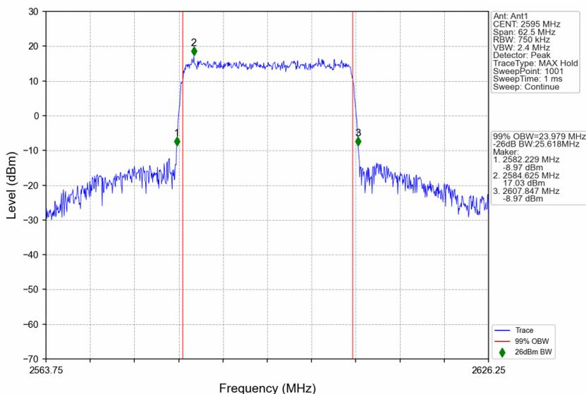
n38\_15kHz\_SISO\_NTNV\_25MHz\_CP-OFDM 64 QAM\_2607.5MHz\_Outer\_Full
