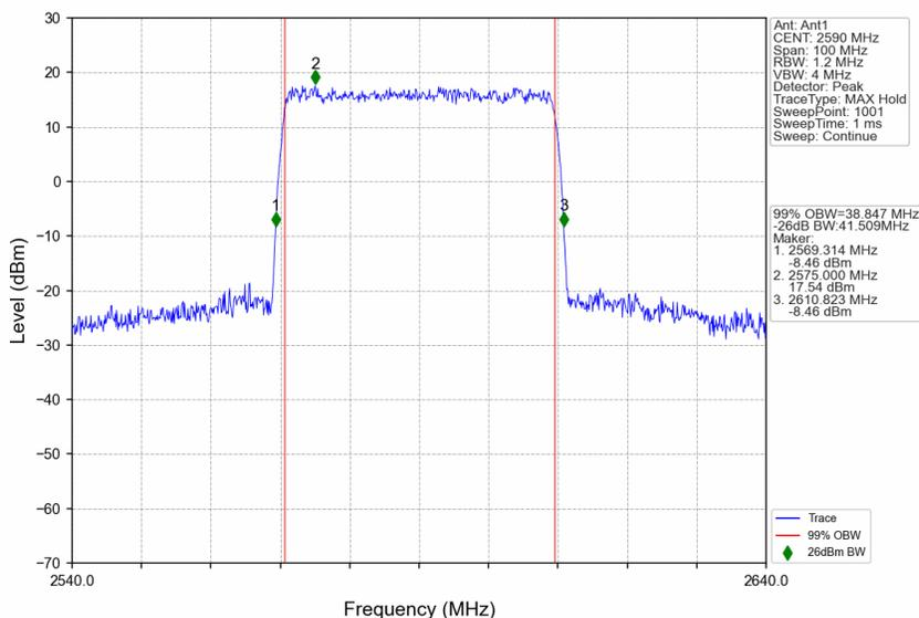
n38\_15kHz\_SISO\_NTNV\_40MHz\_DFT-s-OFDM 16 QAM\_2595MHz\_Outer\_Full
