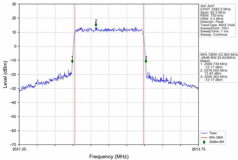
n38\_15kHz\_SISO\_NTNV\_25MHz\_CP-OFDM 256 QAM\_2595MHz\_Outer\_Full
