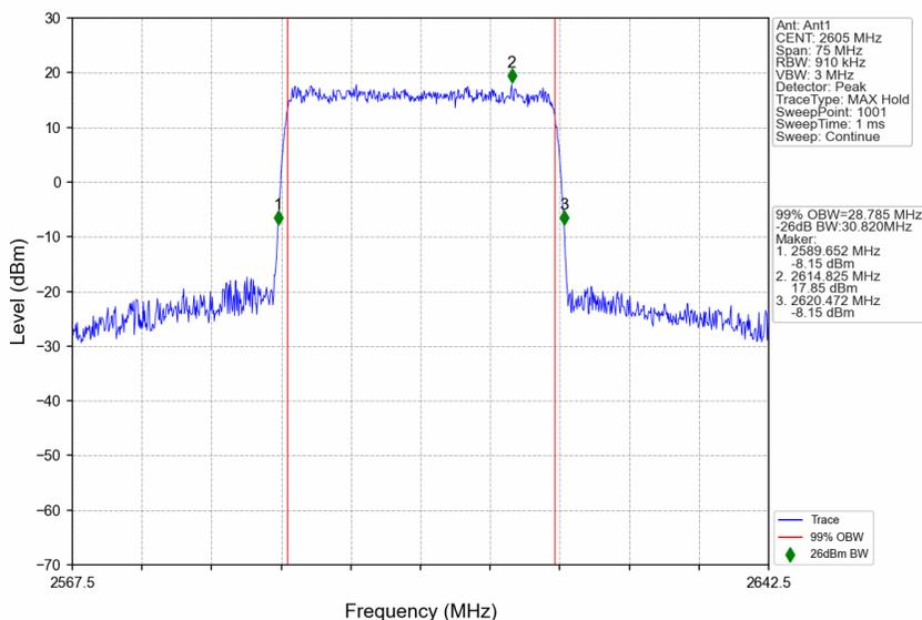
n38\_15kHz\_SISO\_NTNV\_30MHz\_DFT-s-OFDM 64 QAM\_2585MHz\_Outer\_Full
