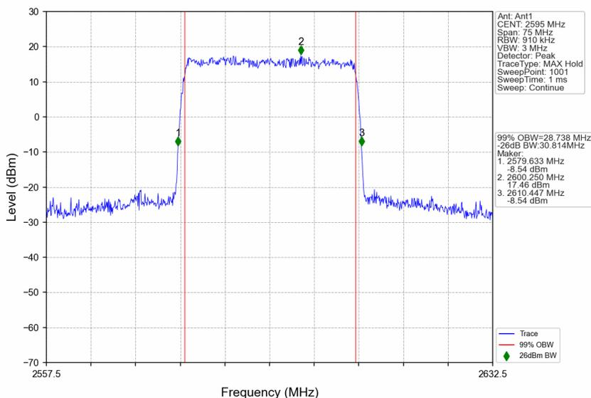
n38\_15kHz\_SISO\_NTNV\_30MHz\_DFT-s-OFDM 64 QAM\_2605MHz\_Outer\_Full
