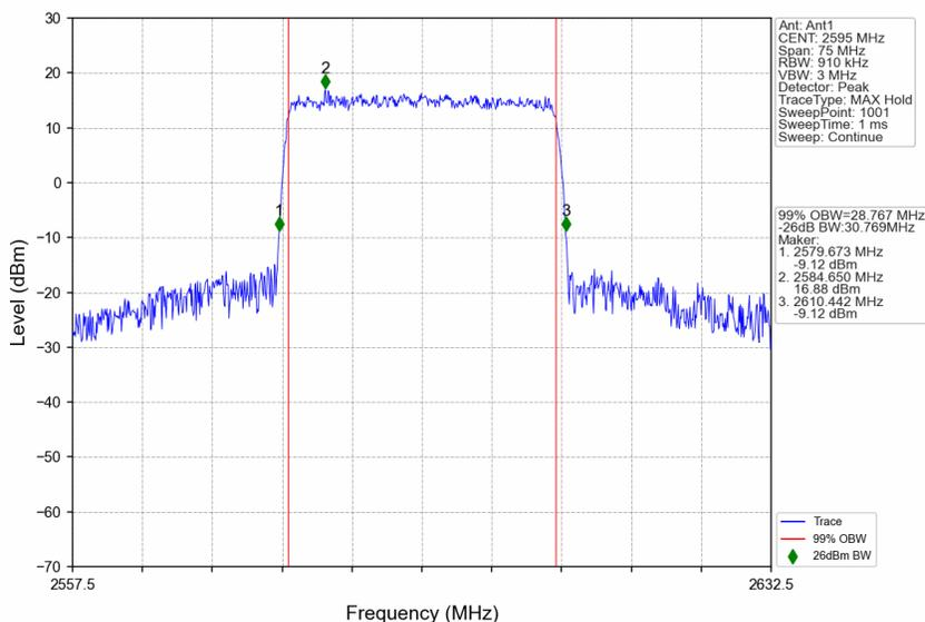
n38\_15kHz\_SISO\_NTNV\_30MHz\_CP-OFDM 64 QAM\_2605MHz\_Outer\_Full
