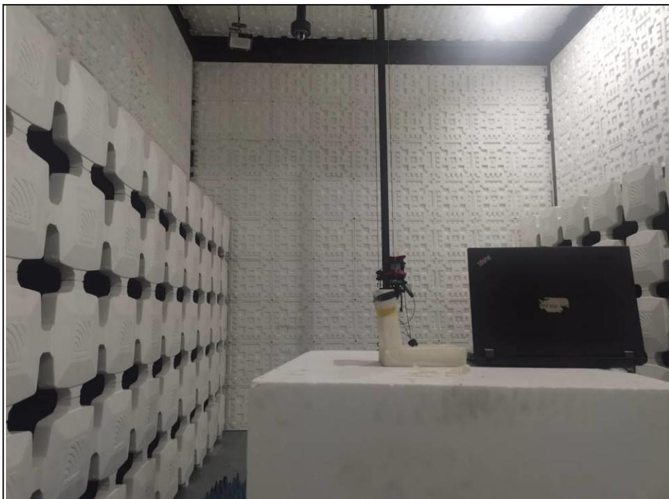
Radiated emission test: Frequency Range < 9KHz- 30MHz >
