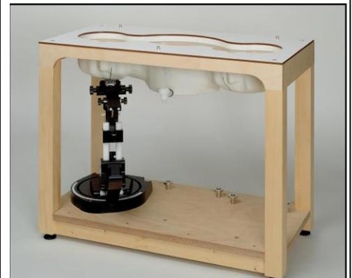
The shell corresponds to the specifications of the Specific Anthropomorphic Mannequin (SAM) phantom defined in IEEE 1528 and IEC 62209-1. It enables the dosimetric evaluation of left and right hand phone usage as well as body mounted usage at the flat phantom region. A cover prevents evaporation of the liquid. Reference markings on the phantom allow the complete setup of all predefined phantom positions and measurement grids by teaching three points with the robot.
