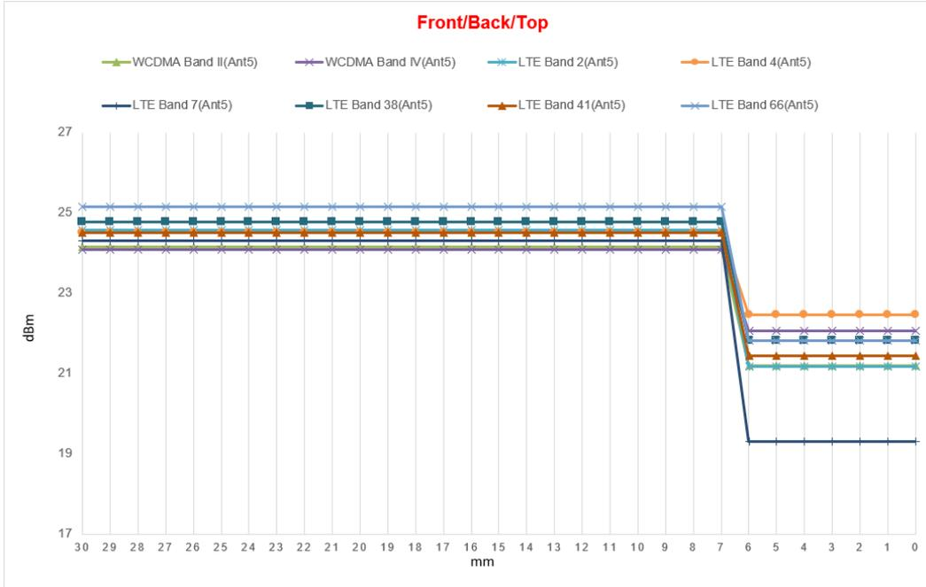
● DUT Moving Away(Release) from the Phantom
