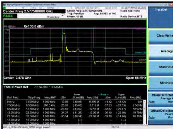
LTE Band 38 64QAM 15MHz CH-High, 1 RB
