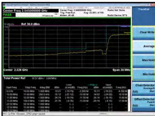
LTE Band 41 64QAM 20MHz CH-High, 100%RB
