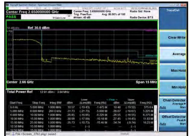
LTE Band 41 16QAM 15MHz CH-Low, 1 RB
