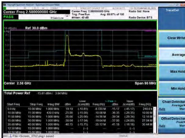
LTE Band 38 64QAM 20MHz CH-High, 1 RB
