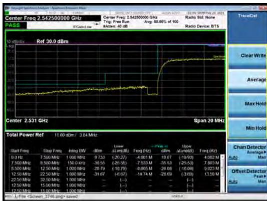
LTE Band 41 64QAM 15MHz CH-High, 100%RB
