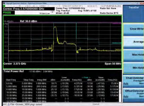
LTE Band 38 64QAM 10MHz CH-High, 1 RB
