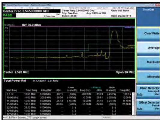
LTE Band 41 64QAM 20MHz CH-High, RB 1
