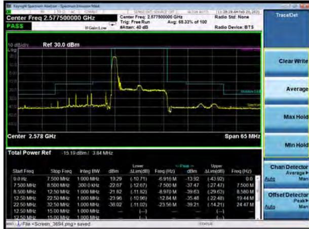
LTE Band 38 16QAM 15MHz CH-High, 1 RB
