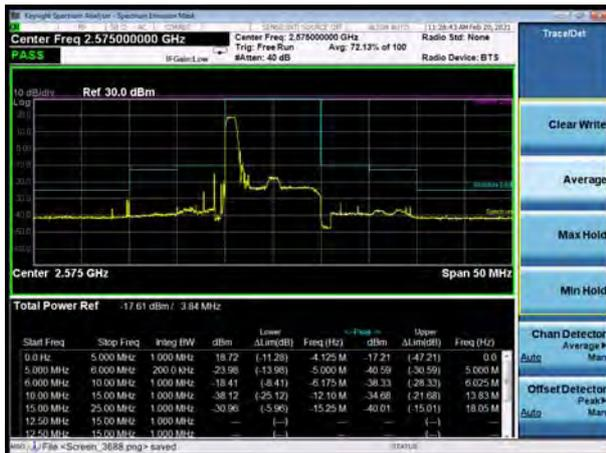
LTE Band 38 16QAM 10MHz CH-High, 1 RB
