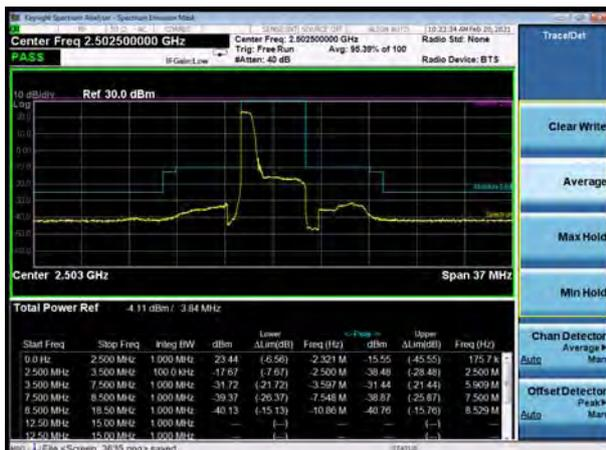
LTE Band 7 64QAM 5MHz CH-High, 1 RB
