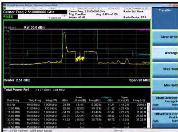
LTE Band 7 64QAM 20MHz CH-High, 1 RB
