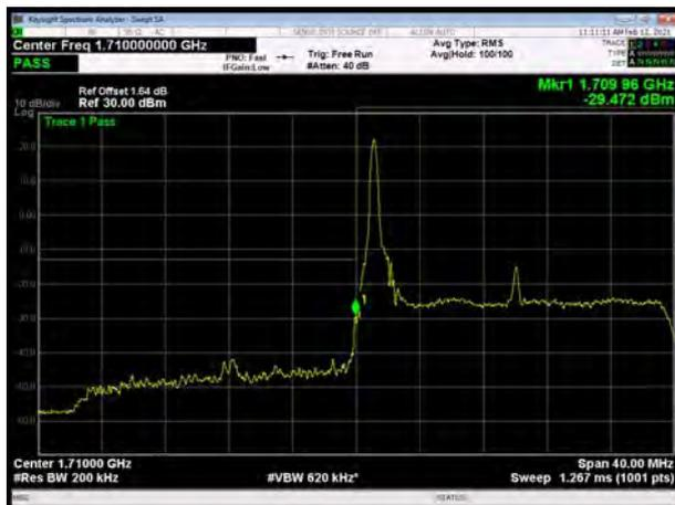
LTE Band 4 16QAM 20MHz CH-High, 1 RB
