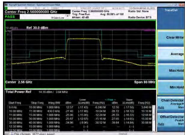
LTE Band 7 64QAM 5MHz CH-Low, 1 RB
