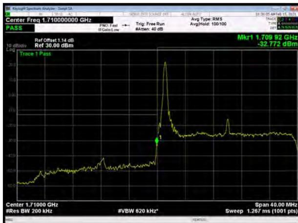
LTE Band 4 64QAM 20MHz CH-High, 1 RB
