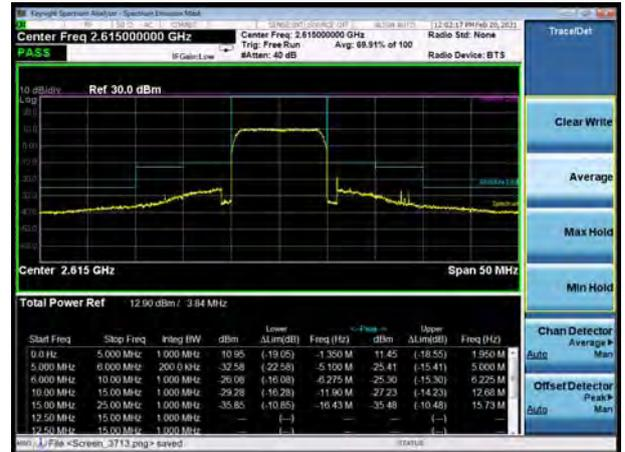
LTE Band 38 16QAM 15MHz CH-Low, 1 RB
