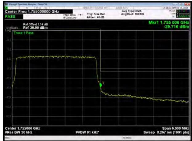
LTE Band 4 64QAM 5MHz CH-Low, 1 RB
