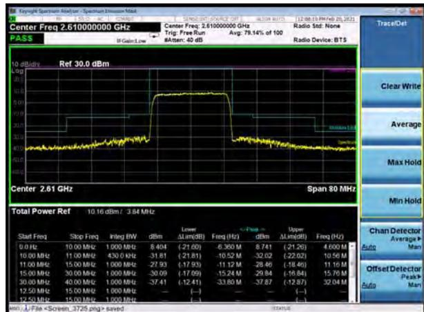
LTE Band 38 64QAM 5MHz CH-Low, 1 RB
