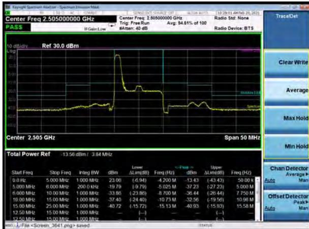
LTE Band 7 64QAM 10MHz CH-High, 1 RB
