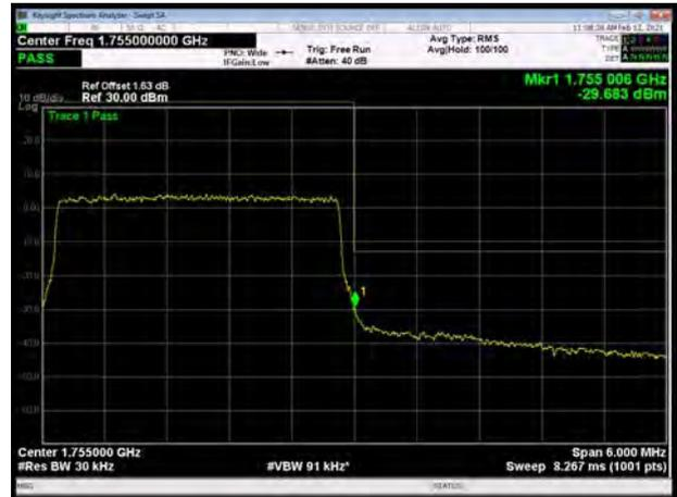
LTE Band 4 16QAM 5MHz CH-Low, 1 RB
