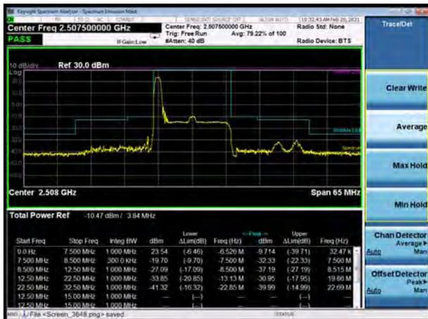
LTE Band 7 64QAM 15MHz CH-High, 1 RB
