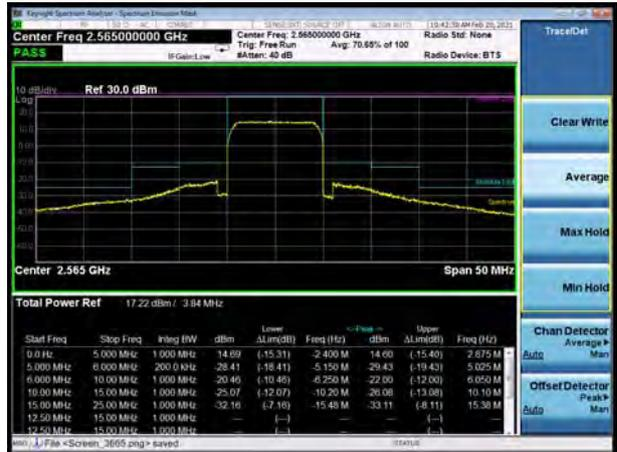
LTE Band 7 16QAM 15MHz CH-Low, 1 RB
