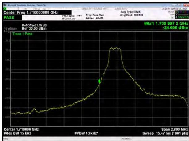
LTE Band 4 64QAM 1.4MHz CH-High, 1 RB
