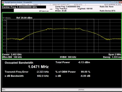
BLE (2M) Carrier frequency (MHz): 2402
