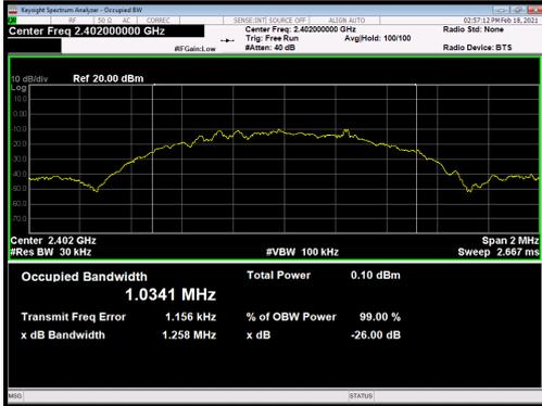
BLE (2M) Carrier frequency (MHz): 2402
