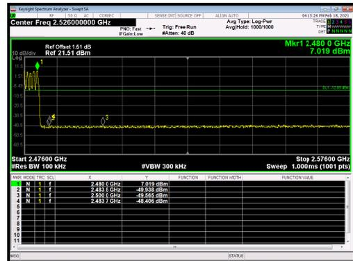
BT 2DH5 CH0, Carrier frequency (MHz): 2402
