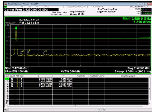
BT 2DH5 CH0, Carrier frequency (MHz): 2402
