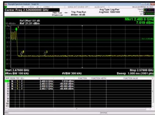
BT 2DH5 CH0, Carrier frequency (MHz): 2402
