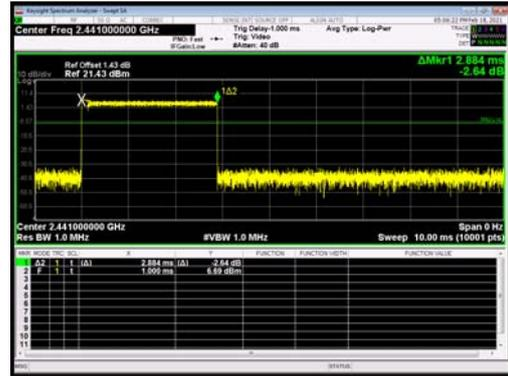
BT 3DH5 CH78, Carrier frequency (MHz): 2480
