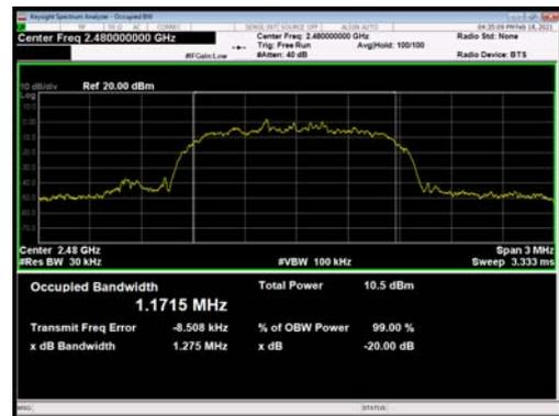
BT 3DH5 CH0, Carrier frequency (MHz): 2402
