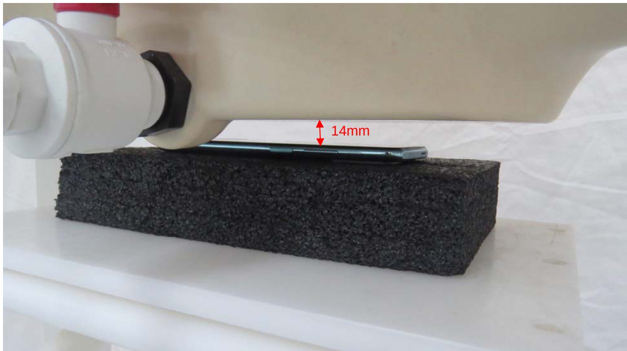
Picture 14: Front Side, the distance from handset to the bottom of the Phantom is 14mm
