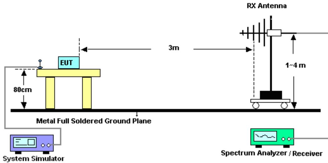
For radiated test above 1GHz
