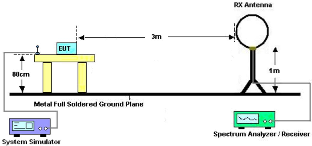
For radiated emissions from 30MHz to 1GHz
