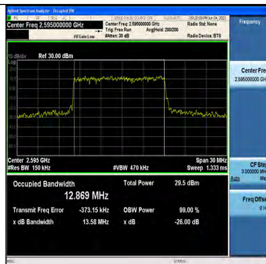
NTNV-N38-30kHz-15MHz-DFT-64QAM- Mid-Outer Full-----PASS
