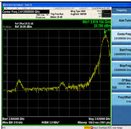
NTNV-N38-30kHz-15MHz-DFT-QPSK- High-Edge_1RB_Right-----2604-2620----- see graph-PASS
