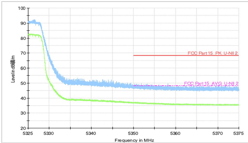
**Fig.20 Band Edges (EUT4, 802.11n-HT40, 5310MHz)**
