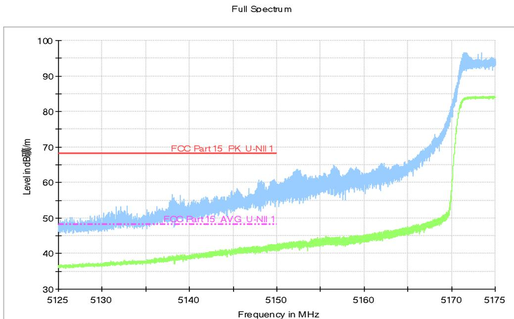
**Fig.27 Band Edges (EUT43, 802.11ax-HT40, 5190MHz)**
