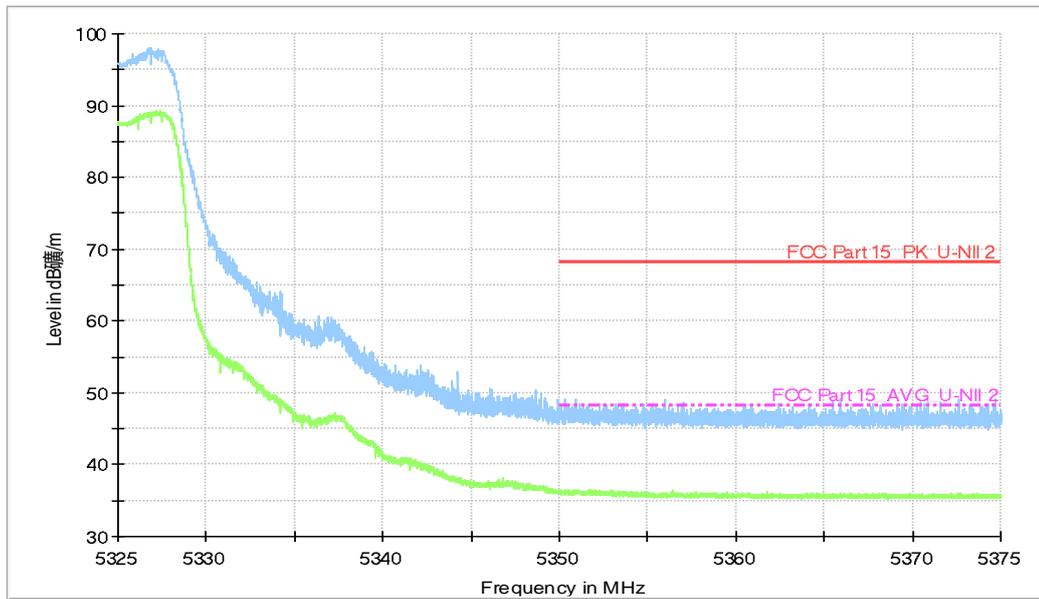
**Fig.4 Band Edges (EUT4, 802.11a, 5320MHz)**
