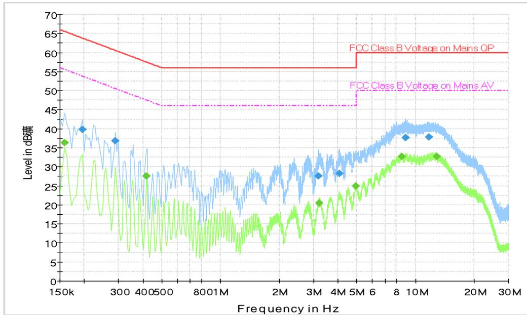
**Fig.37 Conducted Emission(802.11a EUT4(M2001J2G)+AE1+AE3+AE6, Ch40, TX)**
