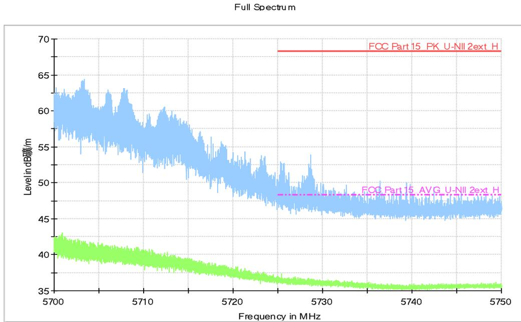
**Fig.30 Band Edges (EUT43, 802.11ax-HT40, 5670MHz)**
