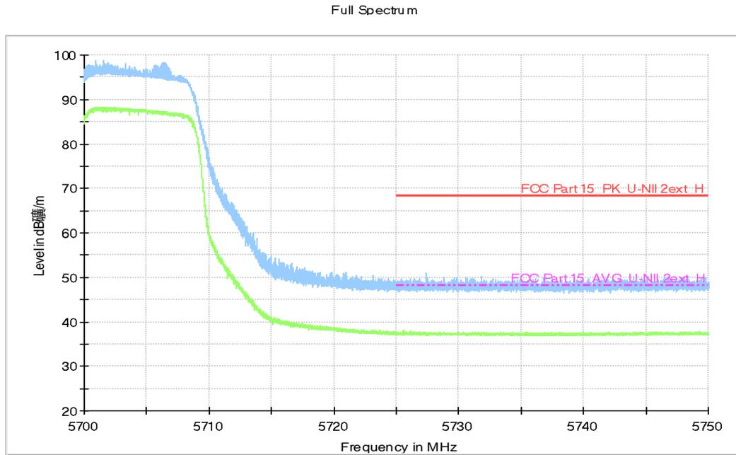
**Fig.10 Band Edges (EUT4, 802.11n-HT20, 5700MHz)**
