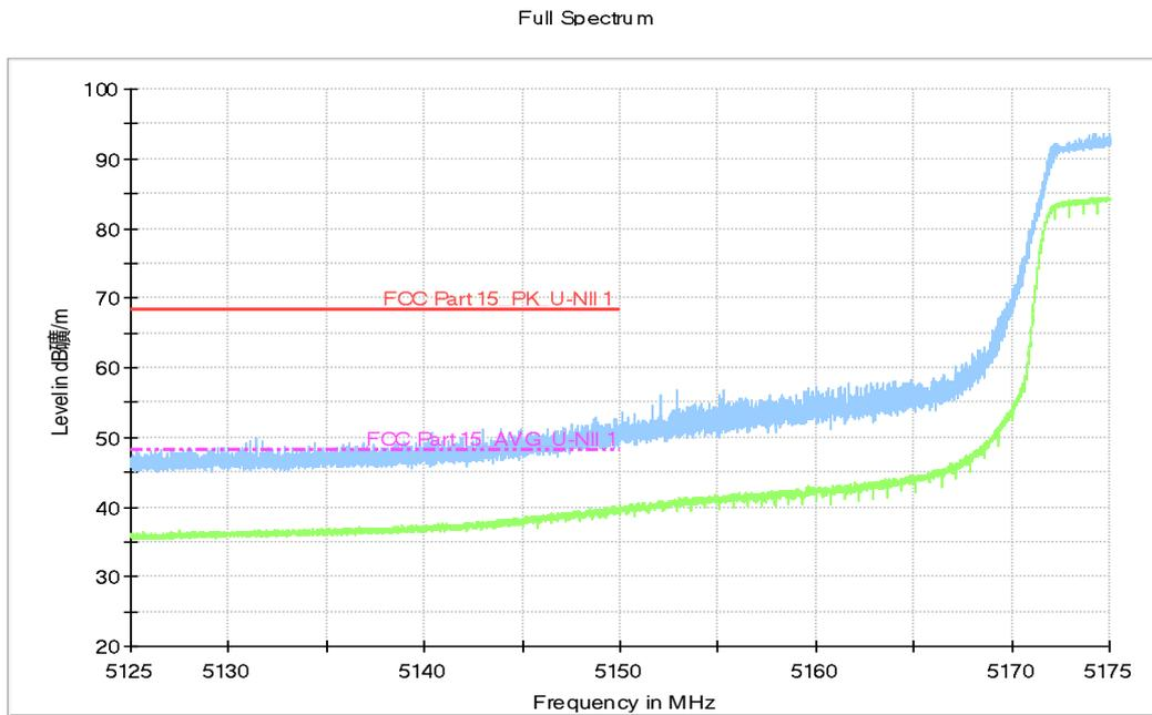
**Fig.19 Band Edges (EUT4, 802.11n-HT40, 5190MHz)**
