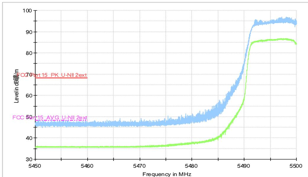
**Fig.13 Band Edges (EUT4, 802.11ac-HT20, 5500MHz)**
