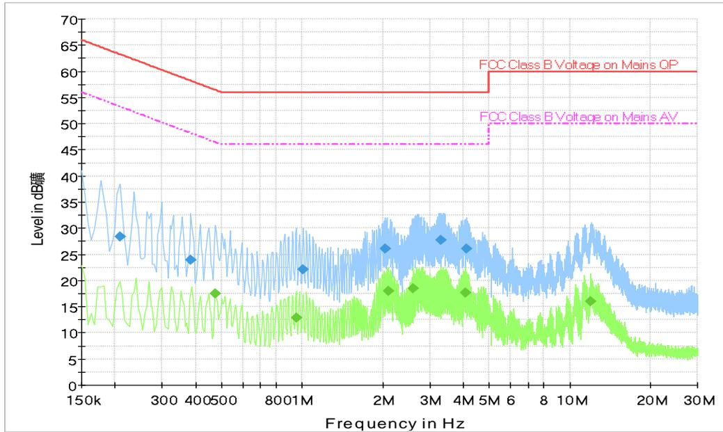
**Fig.40 Conducted Emission( 802.11a EUT43(M2001J1G)+AE11+AE13+AE16, IDLE)**
