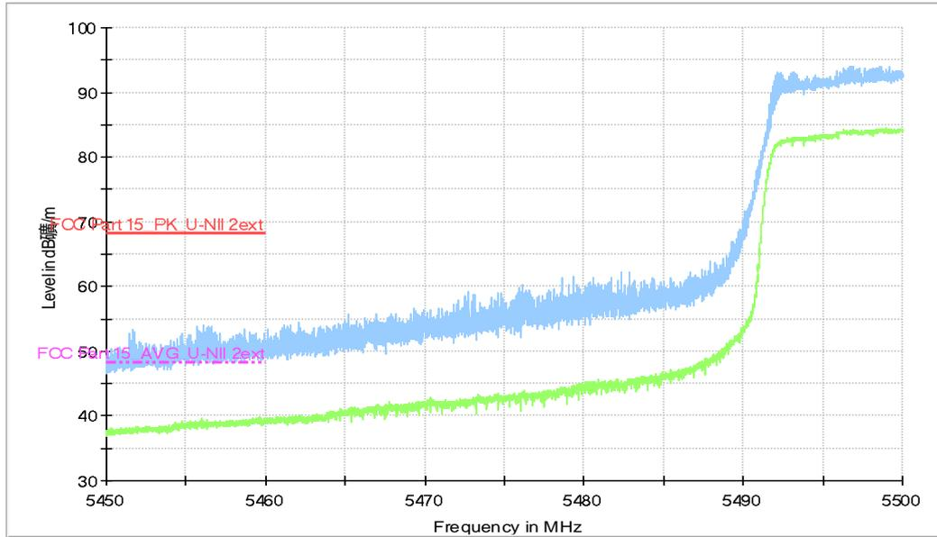
**Fig.22 Band Edges (EUT4, 802.11n-HT40, 5670MHz)**
