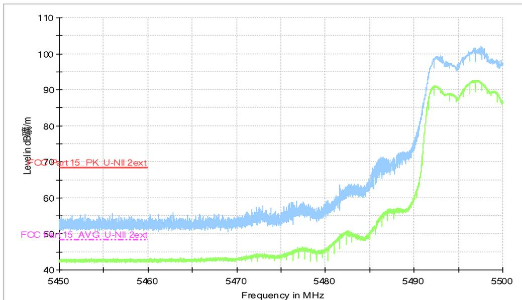
**Fig.5 Band Edges (EUT4, 802.11a, 5500MHz)**
