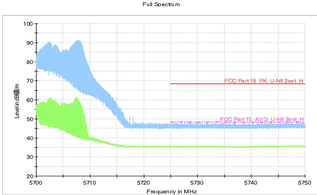
**Fig.18 Band Edges (EUT43, 802.11ax-HT20, 5700MHz)**
