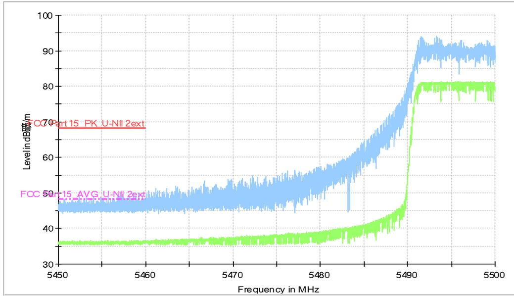
**Fig.36 Band Edges (EUT43, 802.11ax-HT80, 5530MHz)**
