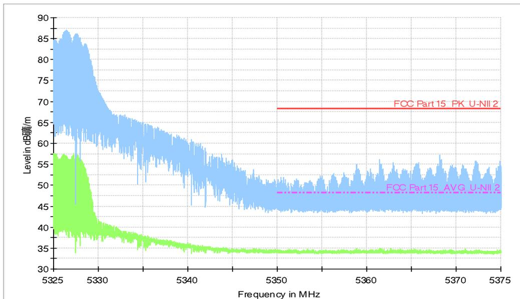
**Fig.35 Band Edges (EUT43, 802.11ax-HT80, 5290MHz)**
