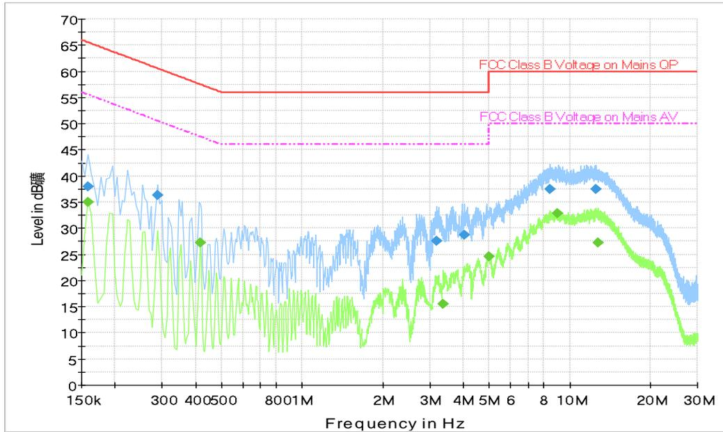
**Fig.38 Conducted Emission( 802.11a EUT4(M2001J2G)+AE1+AE3+AE6, IDLE)**
