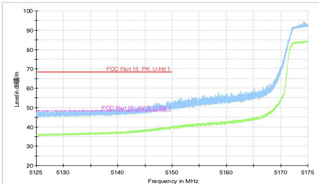
**Fig.23 Band Edges (EUT4, 802.11ac-HT40, 5190MHz)**
