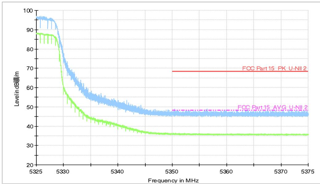
**Fig.12 Band Edges (EUT4, 802.11ac-HT20, 5320MHz)**
