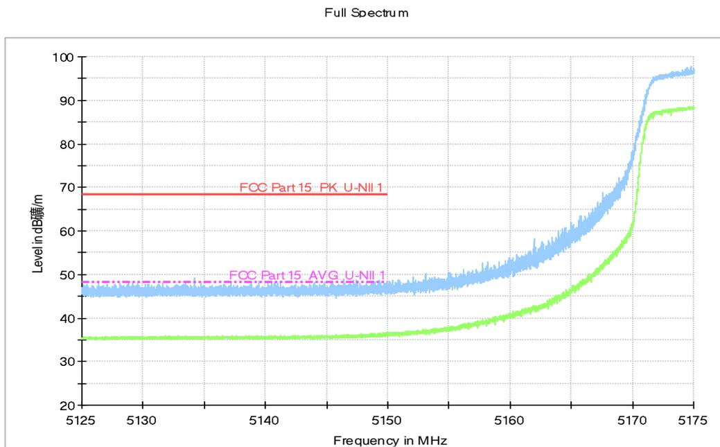
**Fig.11 Band Edges (EUT4, 802.11ac-HT20, 5180MHz)**
