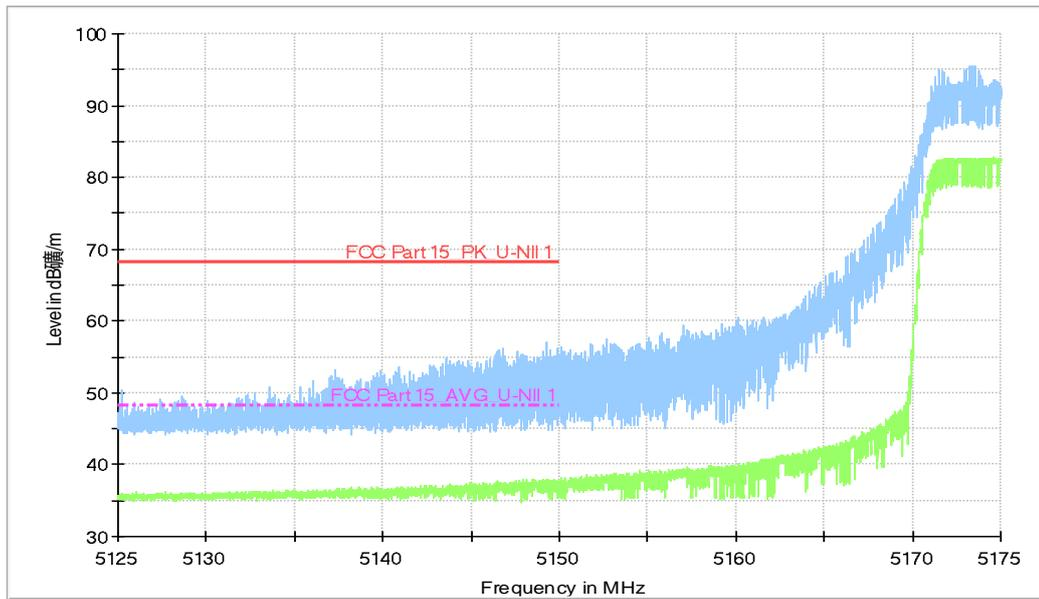
**Fig.34 Band Edges (EUT43, 802.11ax-HT80, 5210MHz)**
