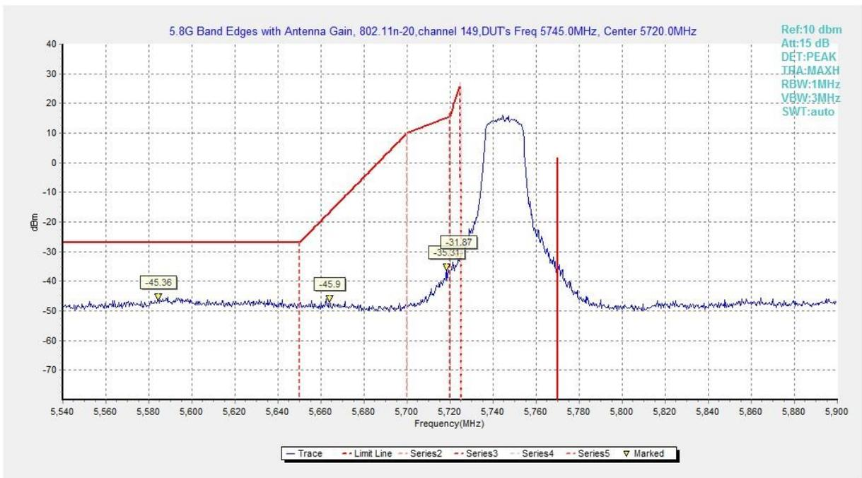
Fig. 141 Band Edges (802.11n-HT20, 5745MHz)
