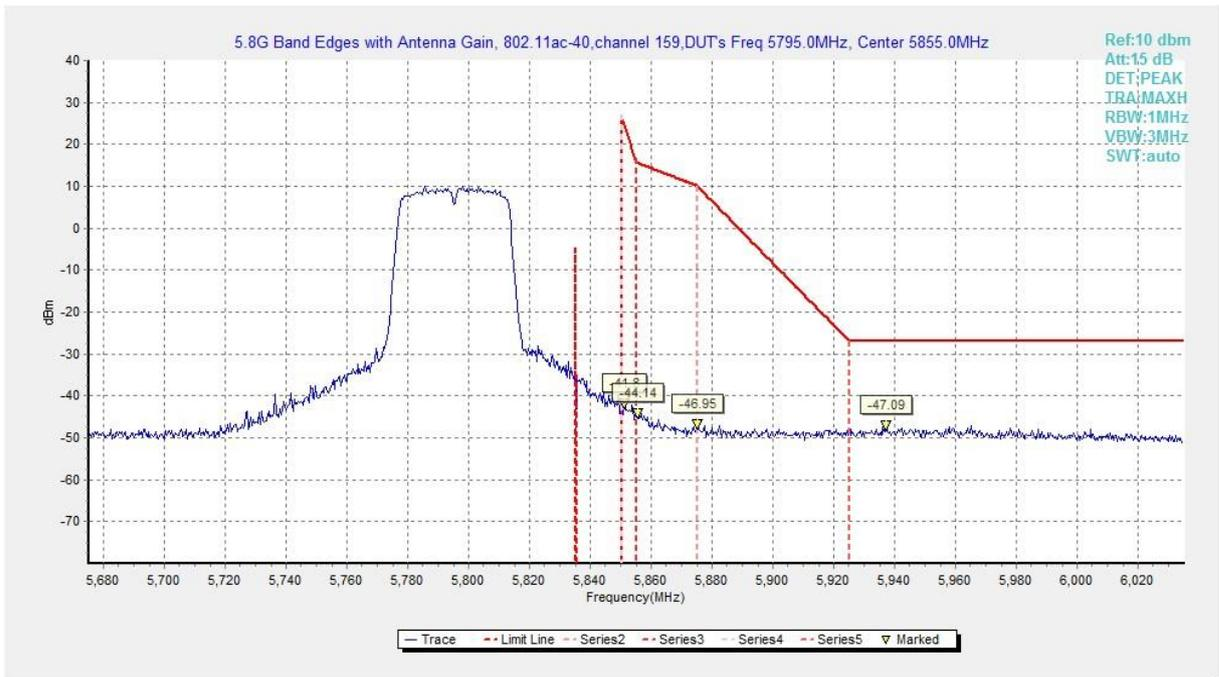
**Fig. 170 Band Edges (802.11ac-HT40, 5795MHz)**
