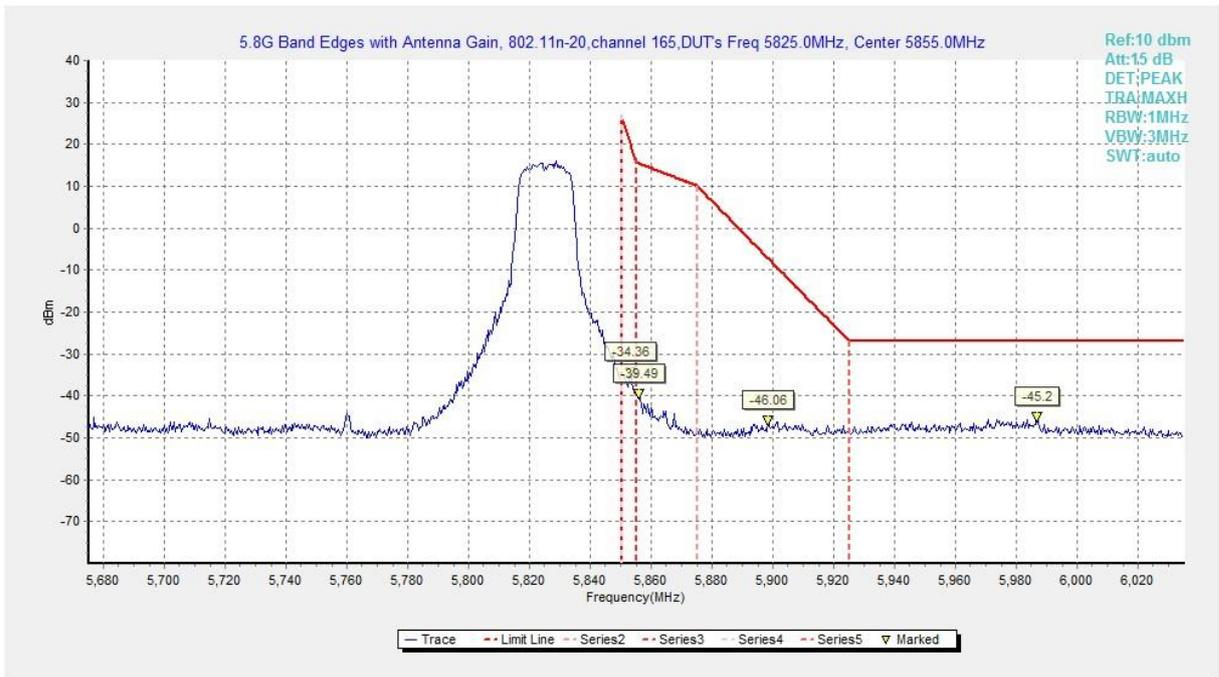
**Fig. 142 Band Edges (802.11n-HT20, 5805MHz)**
