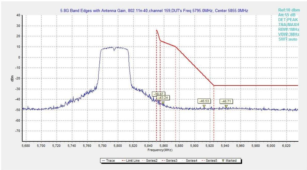
**Fig. 168 Band Edges (802.11n-HT40, 5795MHz)**
