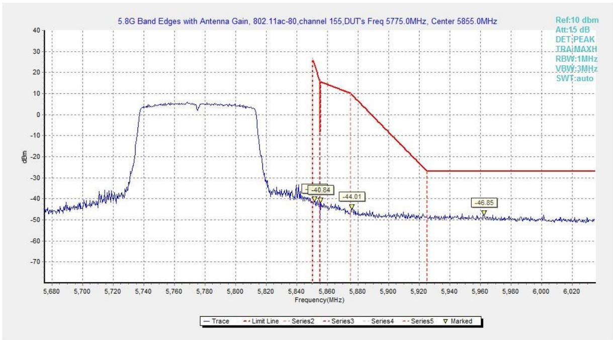
Fig. 172 Band Edges (802.11ac-HT80, 5775MHz)
