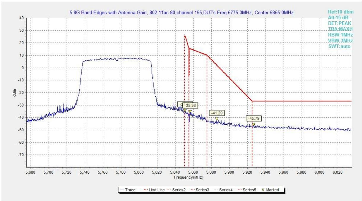
**Fig. 150 Band Edges (802.11ac-HT80, 5775MHz)**
