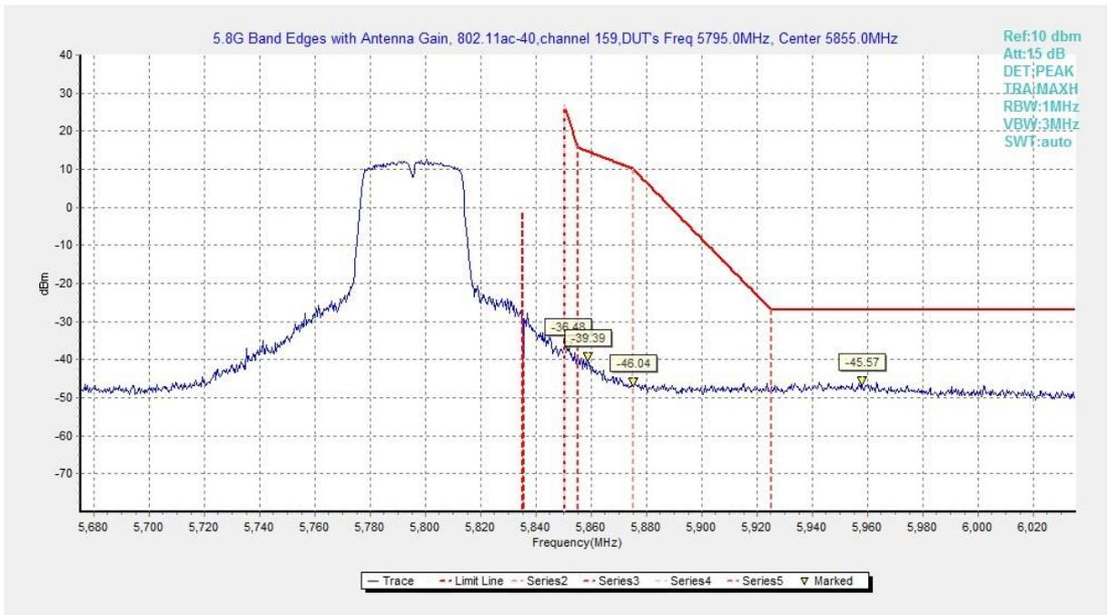
**Fig. 148 Band Edges (802.11ac-HT40, 5795MHz)**
