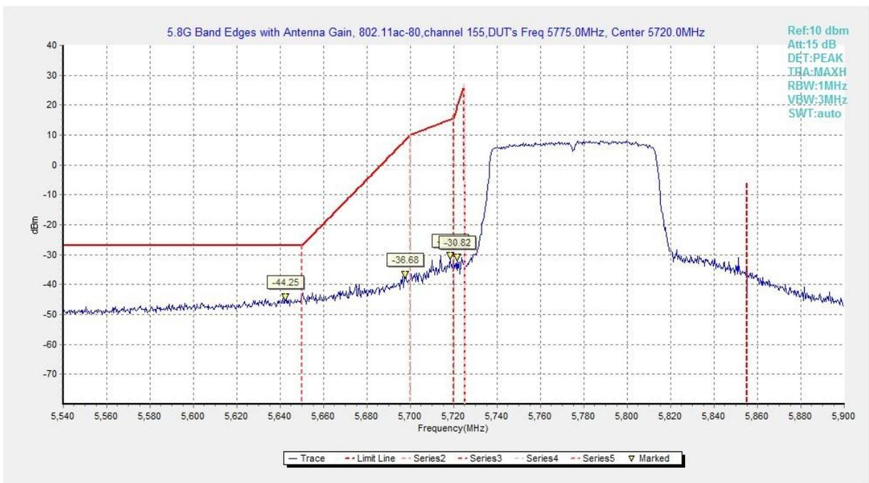
**Fig. 149 Band Edges (802.11ac-HT80, 5775MHz)**
