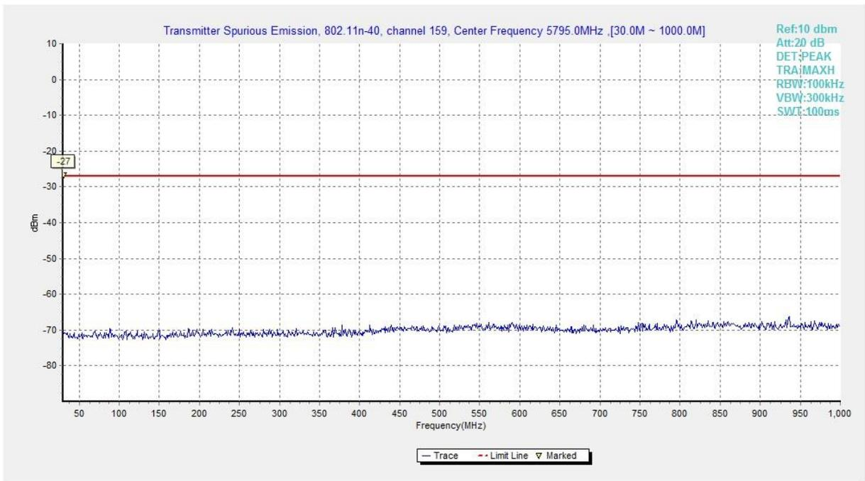
**Fig. 43 Conducted Spurious Emission (802.11n-HT40, Ch159, 30 MHz-1 GHz)**
