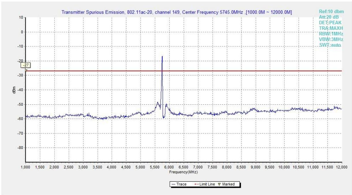
**Fig. 28 Conducted Spurious Emission (802.11ac-HT20, Ch149, 1 GHz -12 GHz)**
