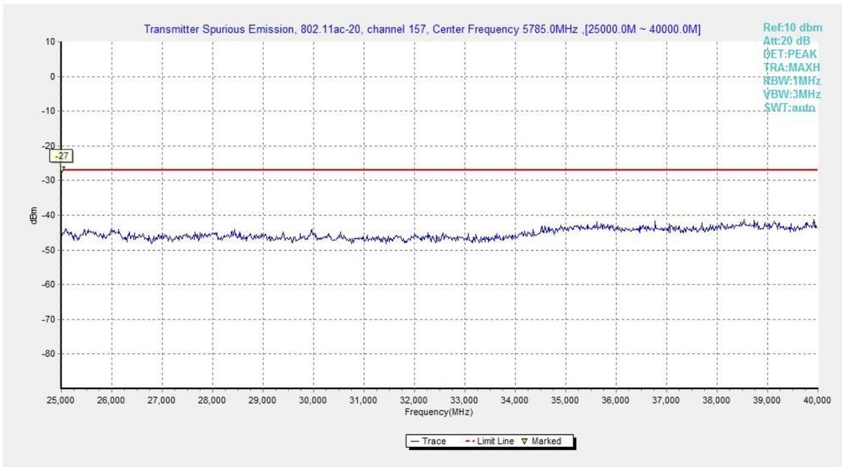
**Fig. 34 Conducted Spurious Emission (802.11ac-HT20, Ch157, 25 GHz-40 GHz)**
