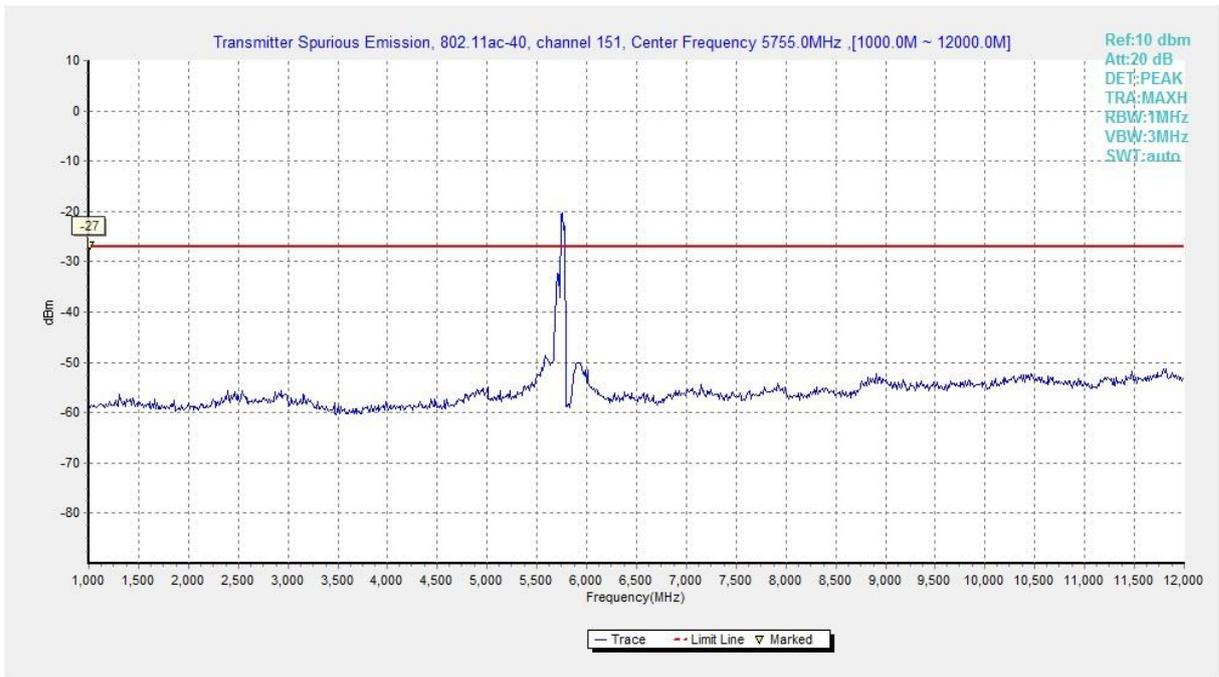
**Fig. 48 Conducted Spurious Emission (802.11ac-HT40, Ch151, 1 GHz -12 GHz)**
