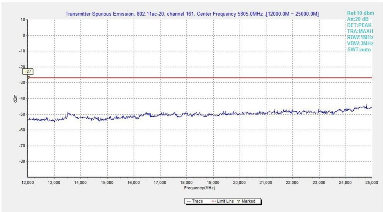
**Fig. 37 Conducted Spurious Emission (802.11ac-HT20, Ch161, 12 GHz-25 GHz)**
