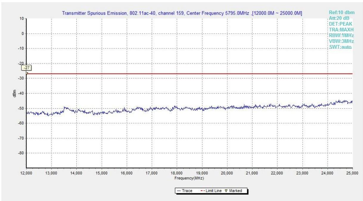
**Fig. 53 Conducted Spurious Emission (802.11ac-HT40, Ch159, 12 GHz-25 GHz)**
