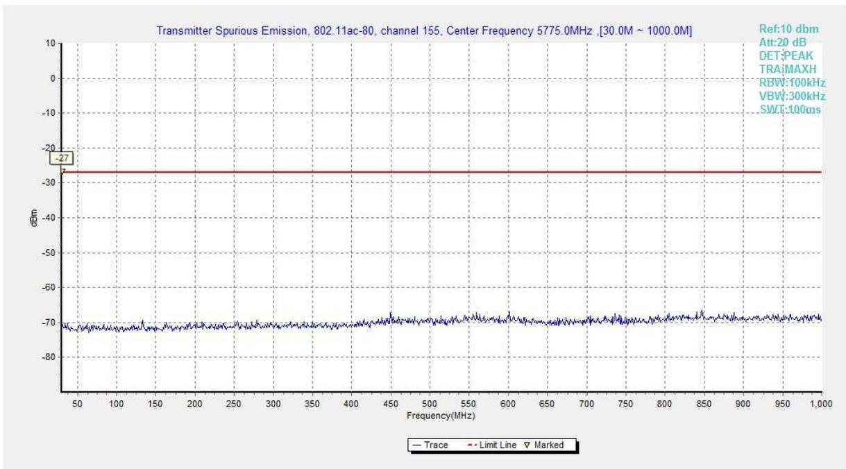
**Fig. 55 Conducted Spurious Emission (802.11ac-HT80, Ch155, 30 MHz-1 GHz)**
