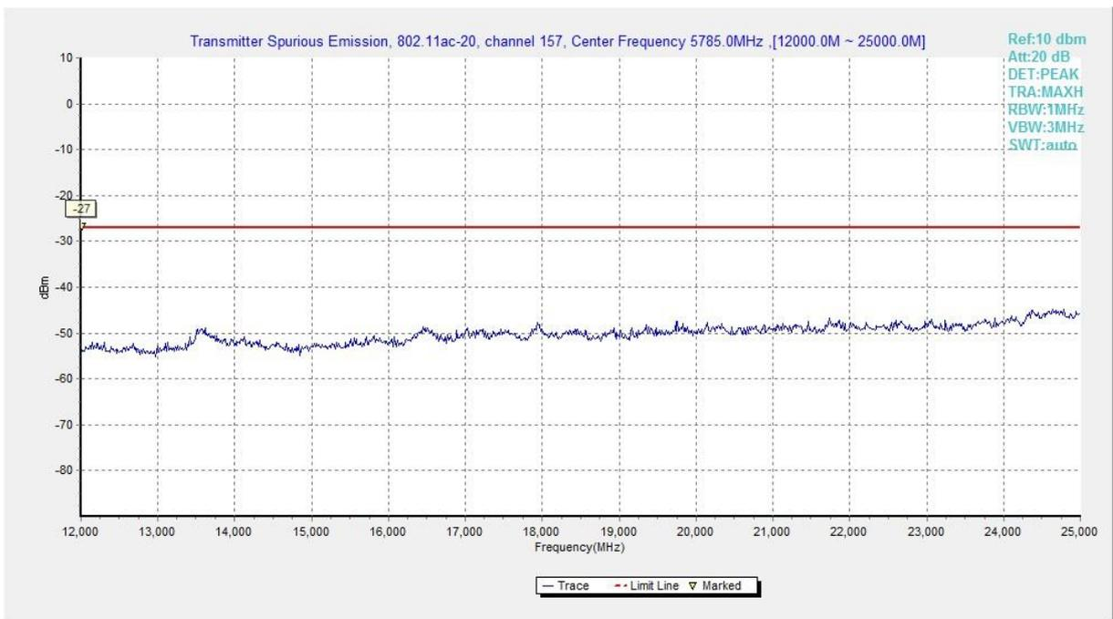
**Fig. 33 Conducted Spurious Emission (802.11ac-HT20, Ch157, 12 GHz-25 GHz)**
