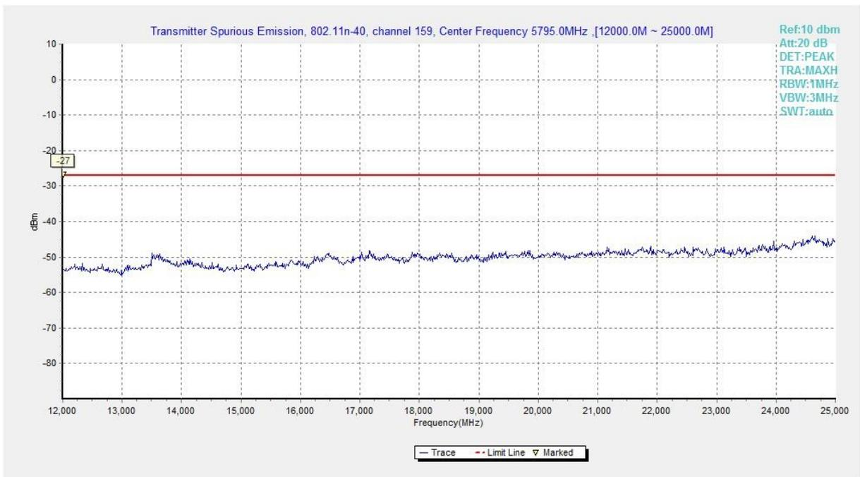
**Fig. 45 Conducted Spurious Emission (802.11n-HT40, Ch159, 12 GHz-25 GHz)**
