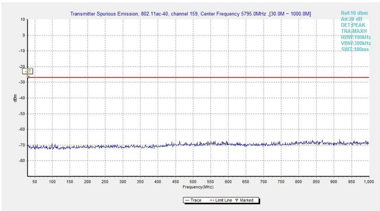
**Fig. 51 Conducted Spurious Emission (802.11ac-HT40, Ch159, 30 MHz-1 GHz)**
