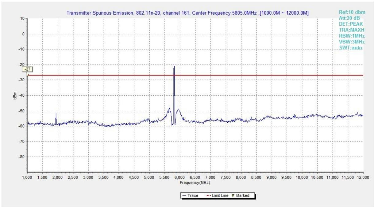
**Fig. 24 Conducted Spurious Emission (802.11n-HT20, Ch161, 1 GHz -12 GHz)**
