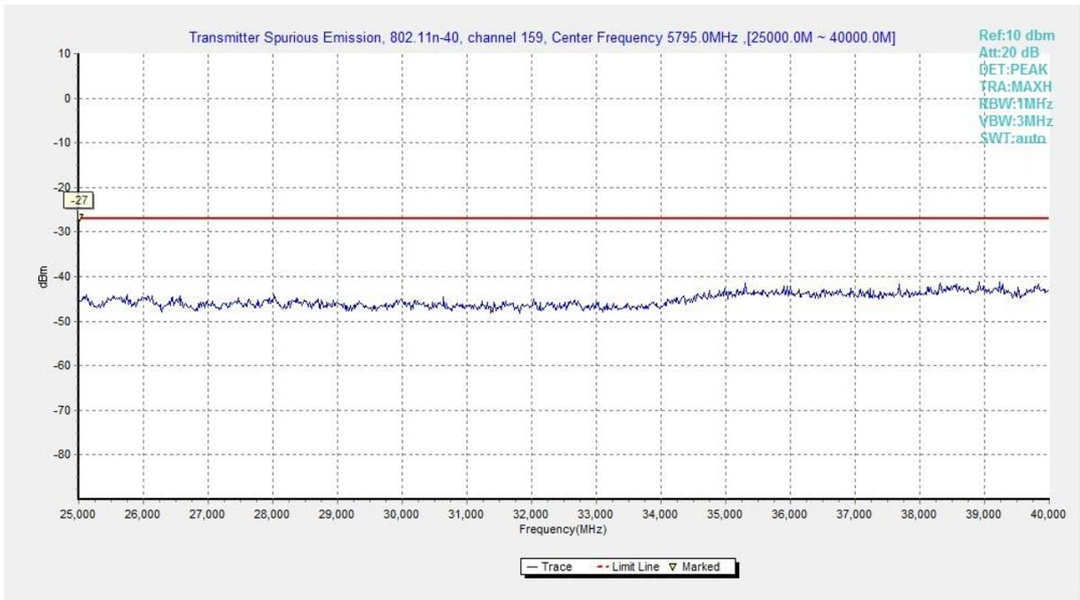
**Fig. 46 Conducted Spurious Emission (802.11n-HT40, Ch159, 25 GHz-40 GHz)**
