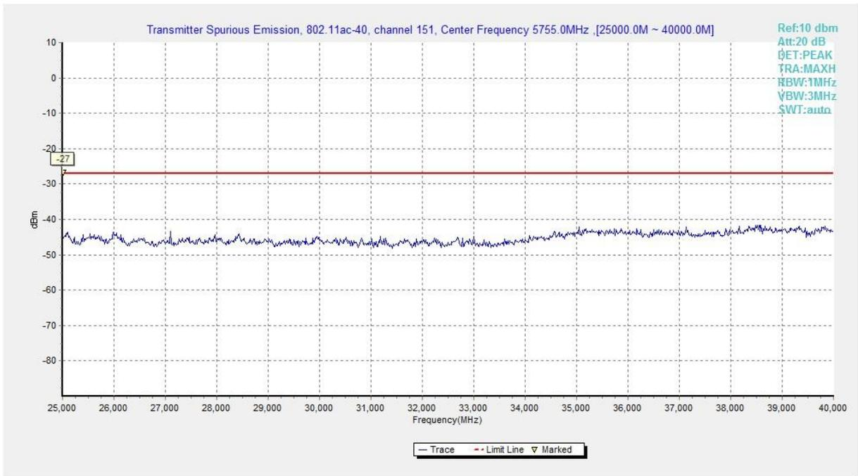
**Fig. 50 Conducted Spurious Emission (802.11ac-HT40, Ch151, 25 GHz-40 GHz)**
