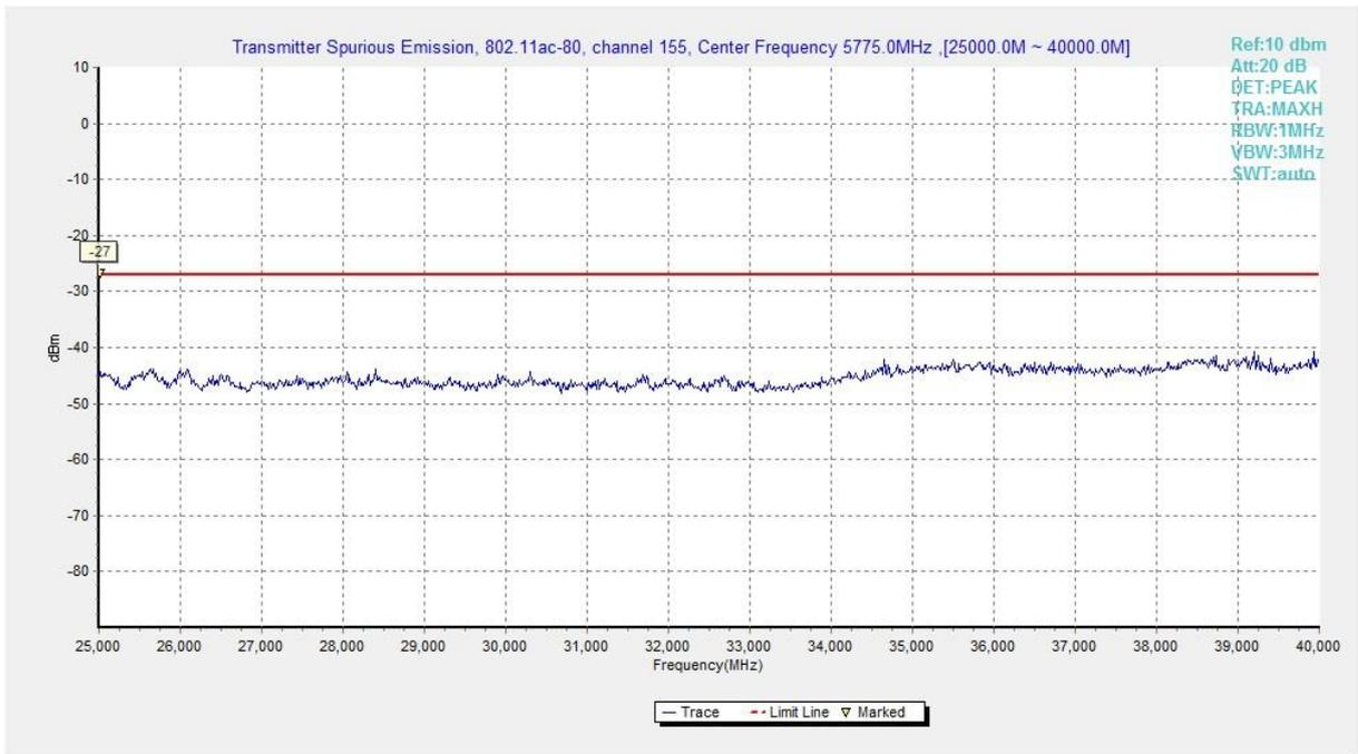
**Fig. 58 Conducted Spurious Emission (802.11ac-HT80, Ch155, 25 GHz-40 GHz)**
