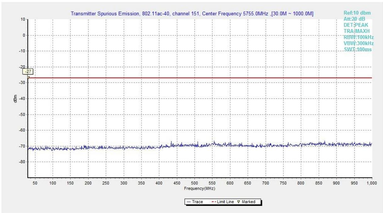
**Fig. 47 Conducted Spurious Emission (802.11ac-HT40, Ch151, 30 MHz-1 GHz)**
