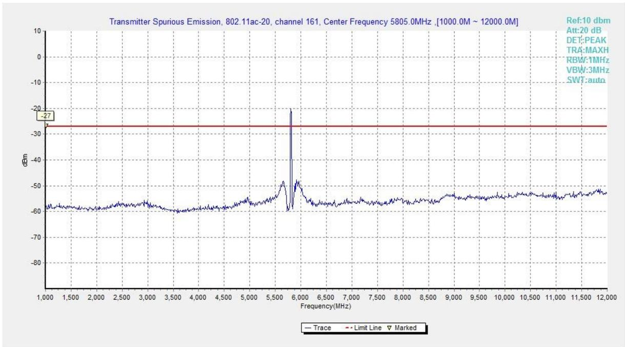
**Fig. 36 Conducted Spurious Emission (802.11ac-HT20, Ch161, 1 GHz -12 GHz)**
