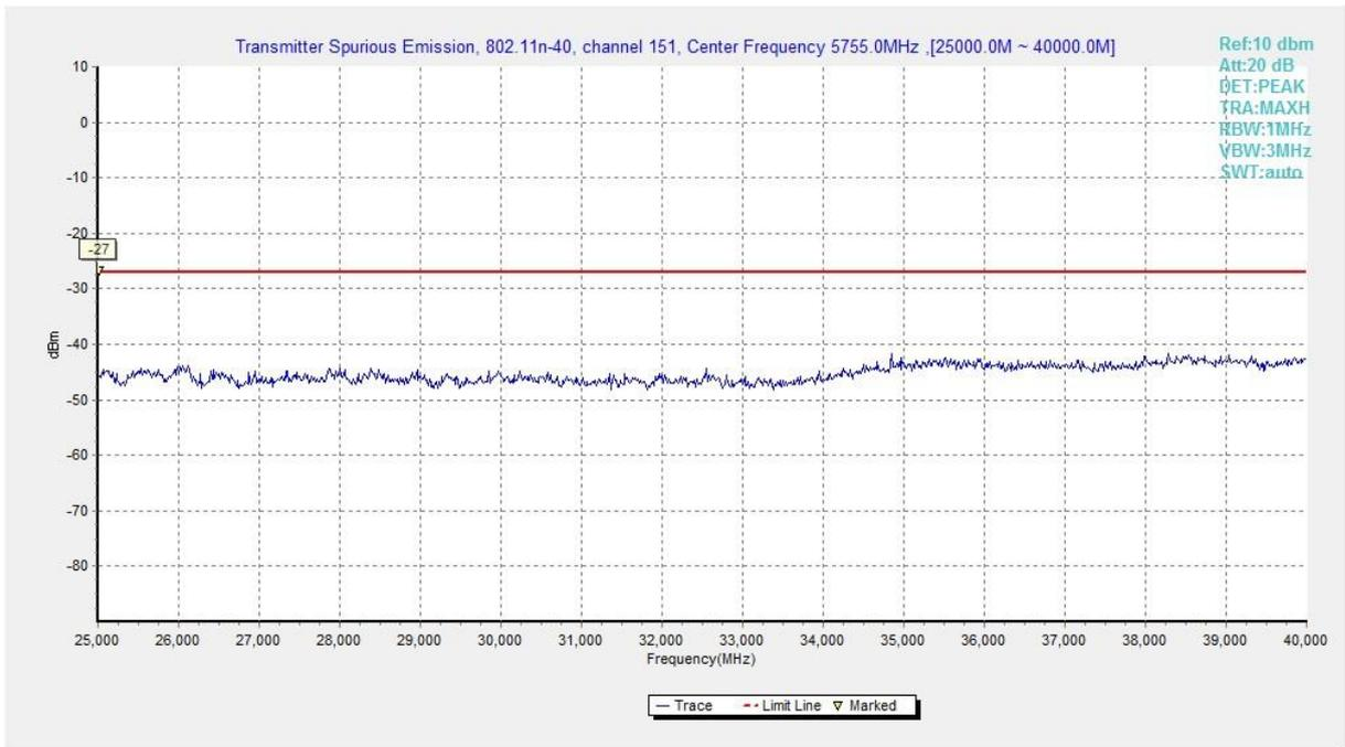
**Fig. 42 Conducted Spurious Emission (802.11n-HT40, Ch151, 25 GHz-40 GHz)**
