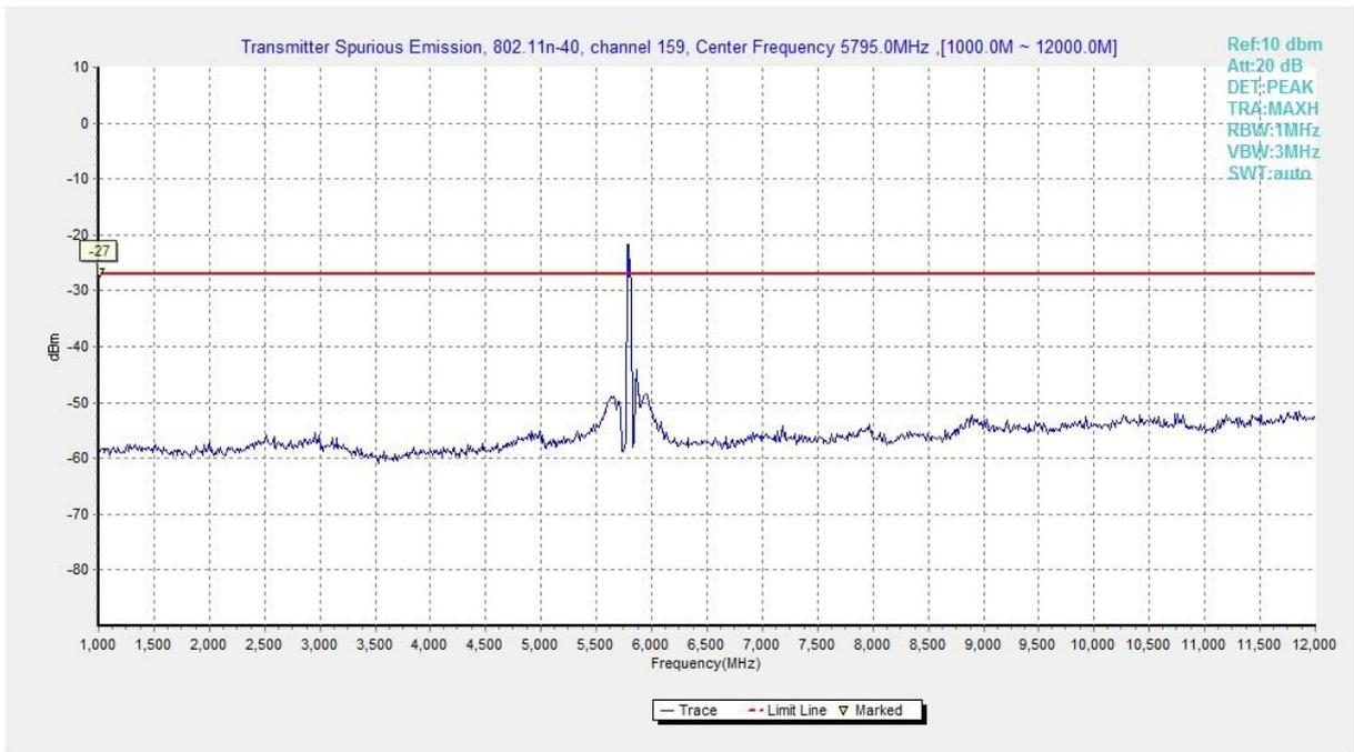
**Fig. 44 Conducted Spurious Emission (802.11n-HT40, Ch159, 1 GHz -12 GHz)**
