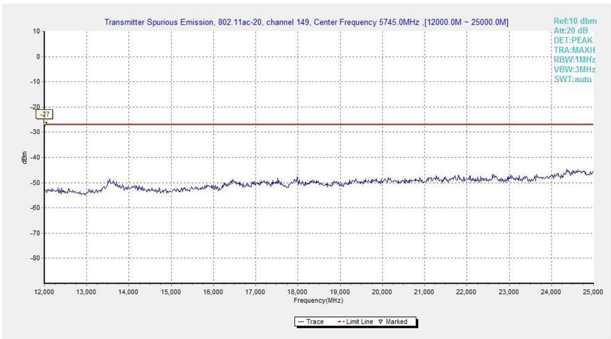
**Fig. 29 Conducted Spurious Emission (802.11ac-HT20, Ch149, 12 GHz-25 GHz)**
