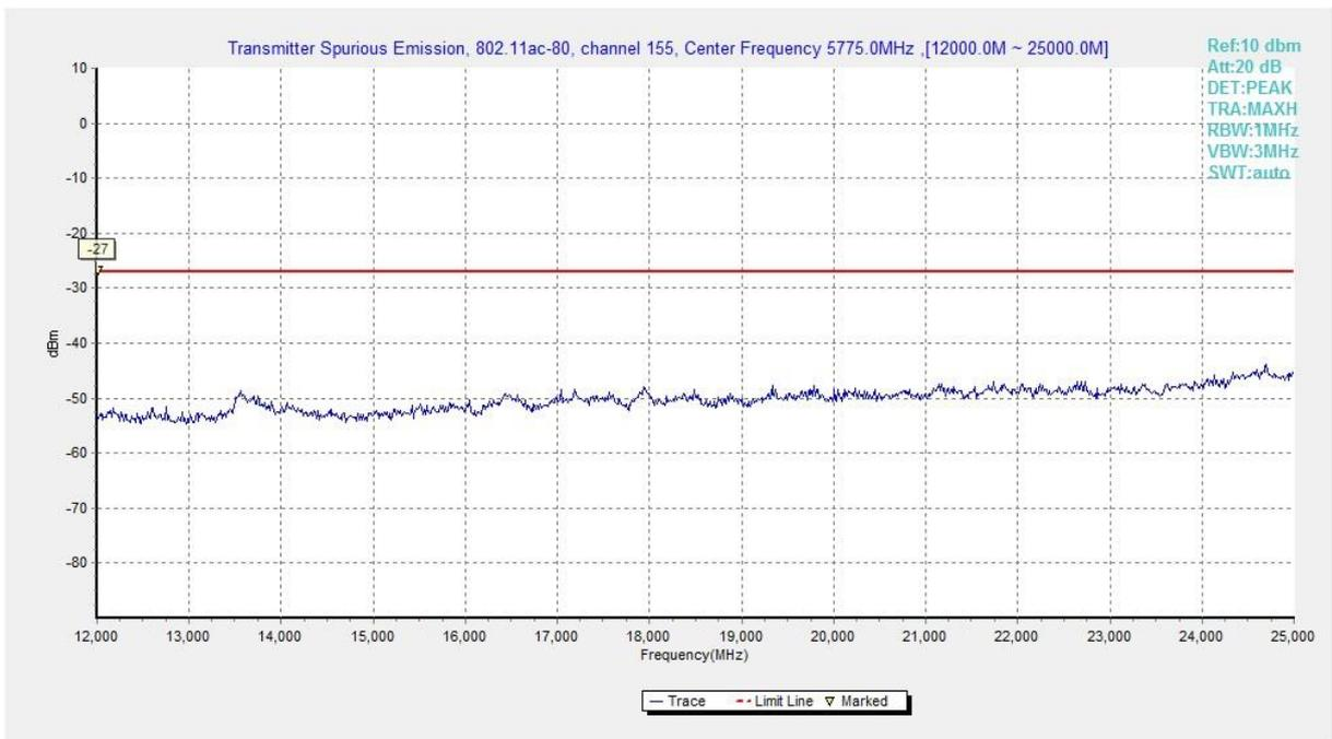
**Fig. 57 Conducted Spurious Emission (802.11ac-HT80, Ch155, 12 GHz-25 GHz)**
