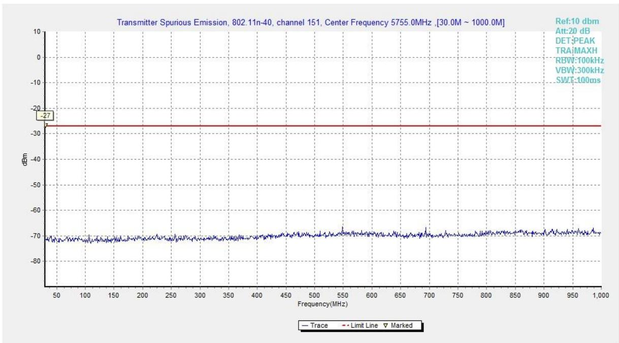
**Fig. 39 Conducted Spurious Emission (802.11n-HT40, Ch151, 30 MHz-1 GHz)**
