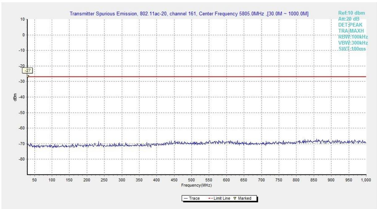
**Fig. 35 Conducted Spurious Emission (802.11ac-HT20, Ch161, 30 MHz-1 GHz)**
