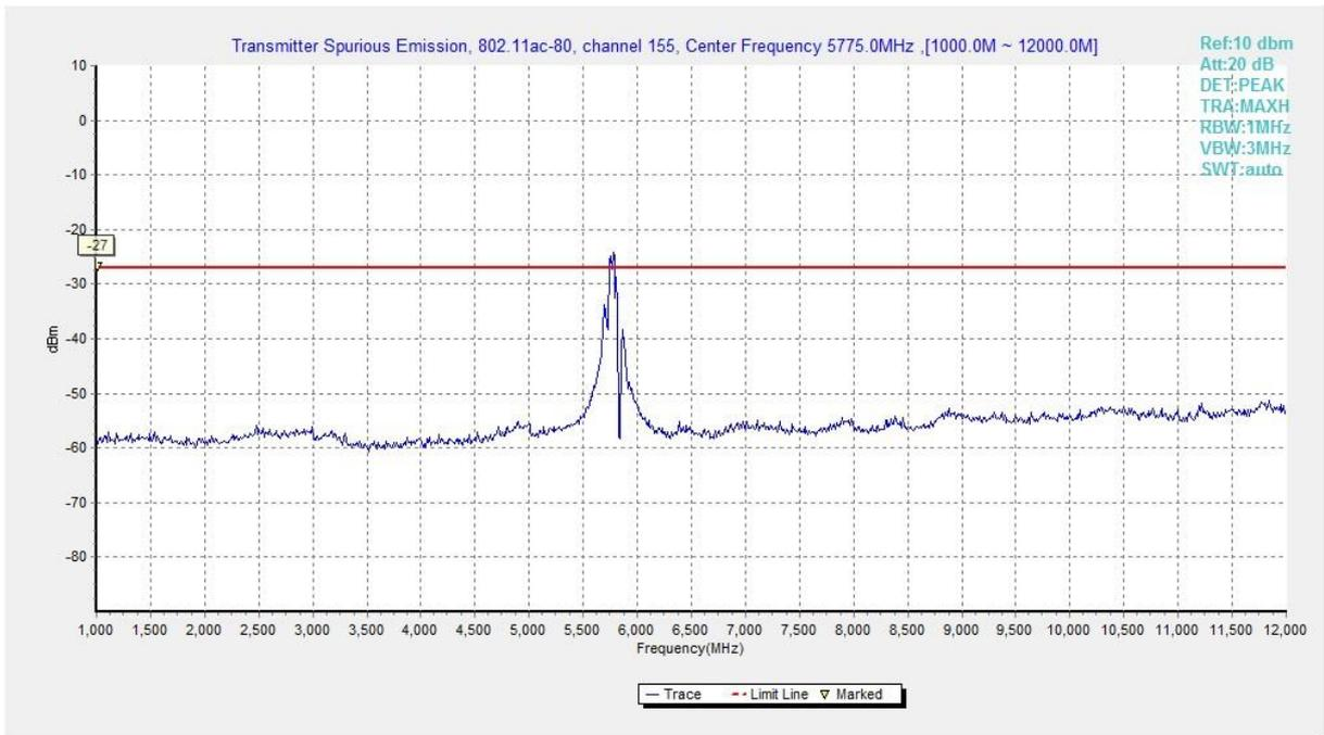
**Fig. 56 Conducted Spurious Emission (802.11ac-HT80, Ch155, 1 GHz -12 GHz)**
