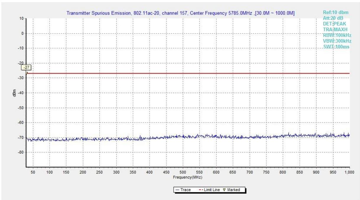
**Fig. 31 Conducted Spurious Emission (802.11ac-HT20, Ch157, 30 MHz-1 GHz)**
