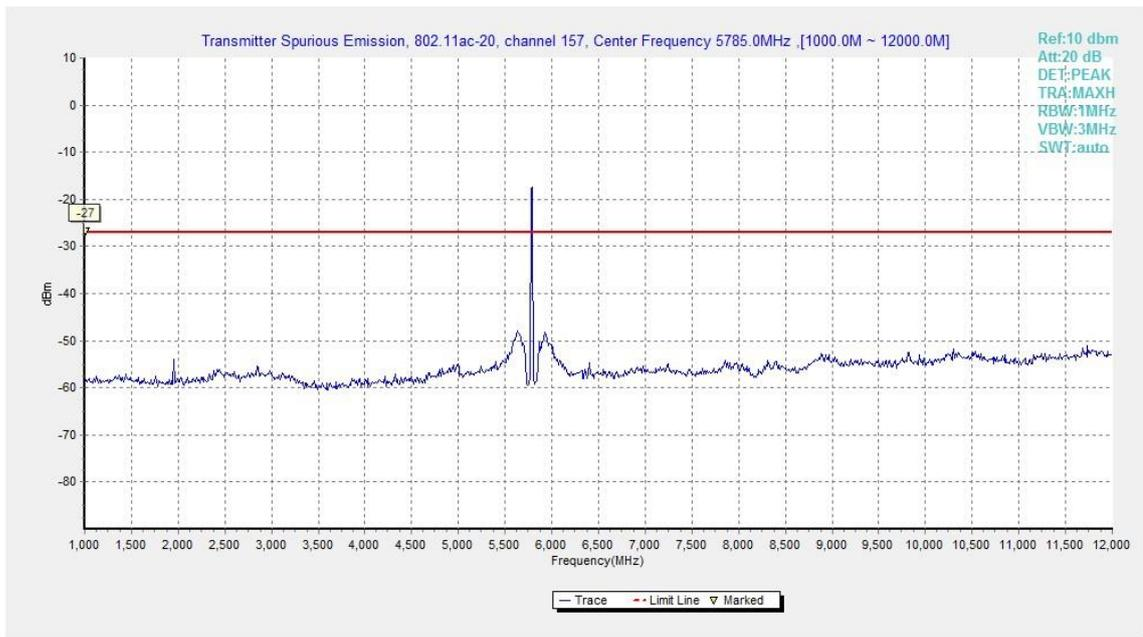
**Fig. 32 Conducted Spurious Emission (802.11ac-HT20, Ch157, 1 GHz -12 GHz)**
