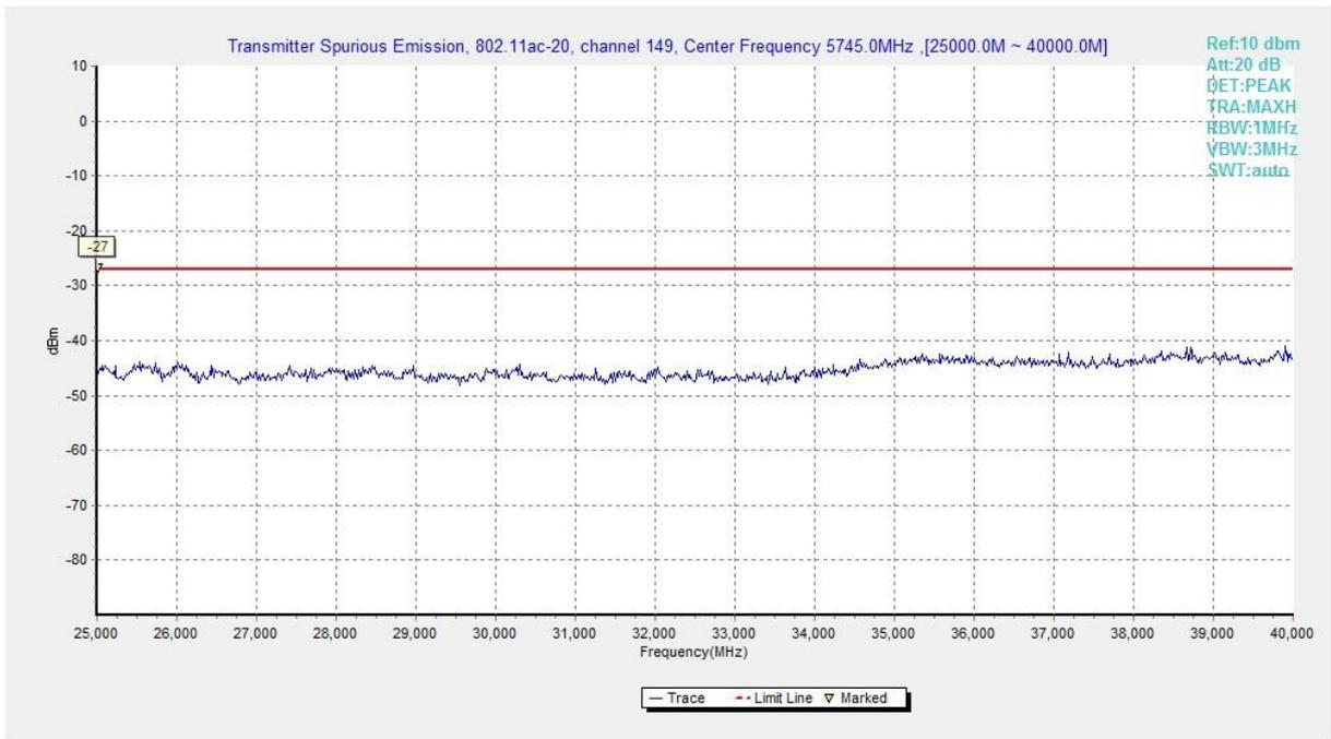
**Fig. 30 Conducted Spurious Emission (802.11ac-HT20, Ch149, 25 GHz-40 GHz)**
