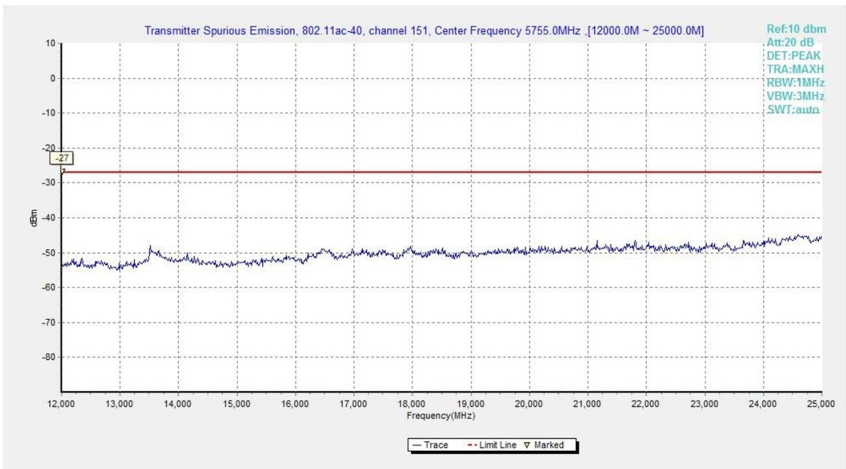
**Fig. 49 Conducted Spurious Emission (802.11ac-HT40, Ch151, 12 GHz-25 GHz)**
