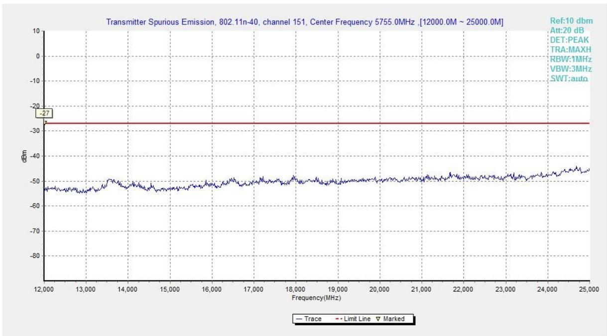
**Fig. 41 Conducted Spurious Emission (802.11n-HT40, Ch151, 12 GHz-25 GHz)**
