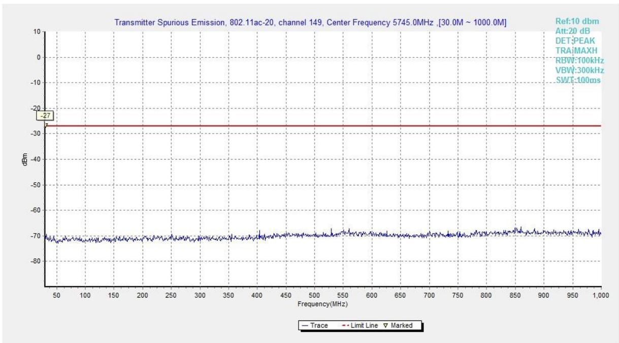
**Fig. 27 Conducted Spurious Emission (802.11ac-HT20, Ch149, 30 MHz-1 GHz)**
