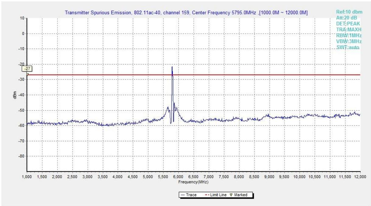
**Fig. 52 Conducted Spurious Emission (802.11ac-HT40, Ch159, 1 GHz -12 GHz)**
