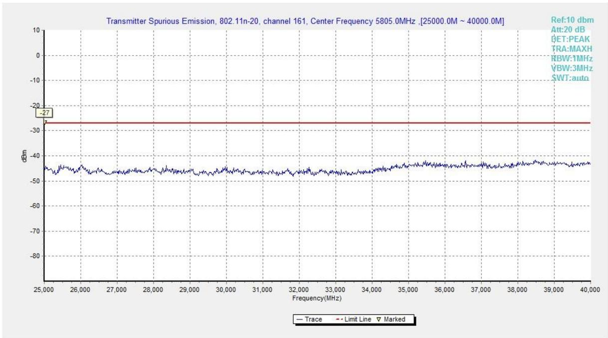
**Fig. 26 Conducted Spurious Emission (802.11n-HT20, Ch161, 25 GHz-40 GHz)**
