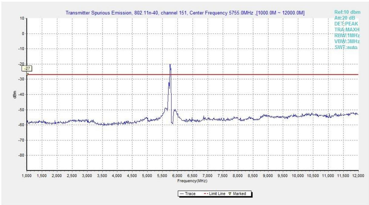
**Fig. 40 Conducted Spurious Emission (802.11n-HT40, Ch151, 1 GHz -12 GHz)**
