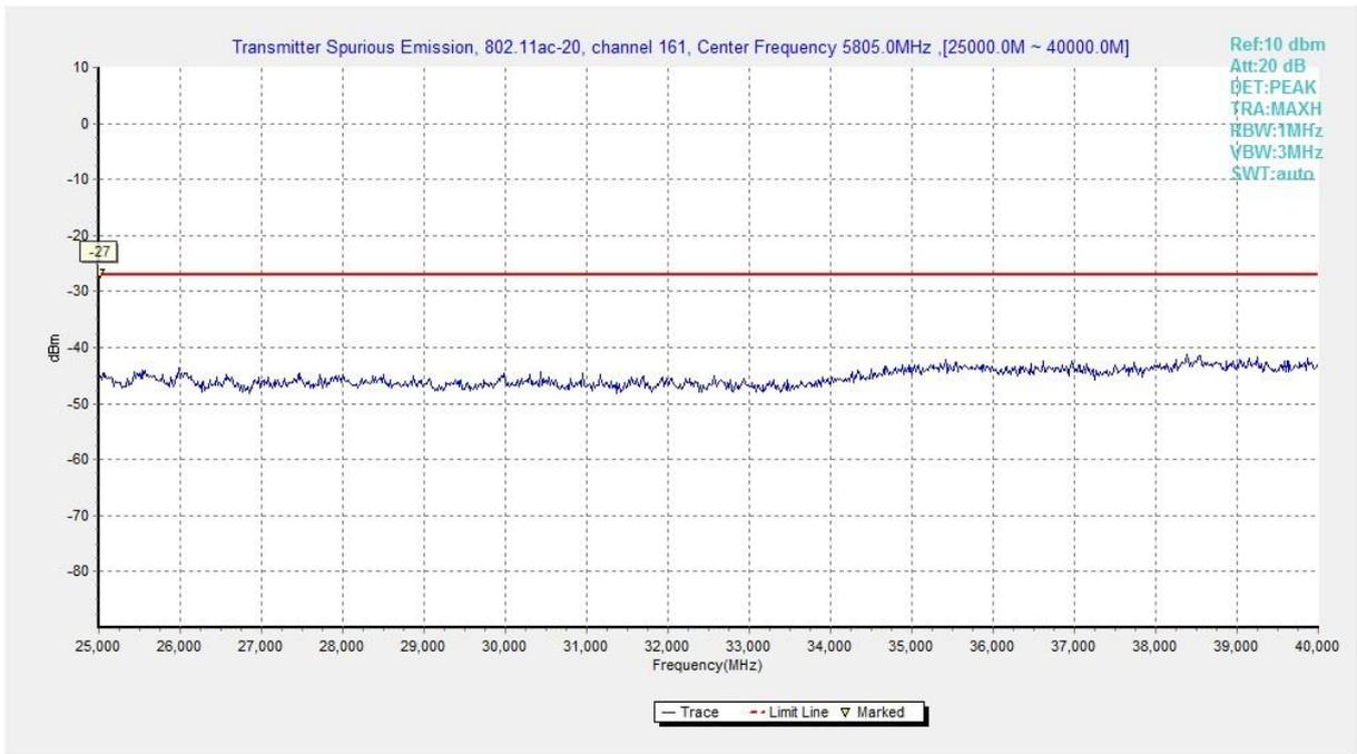
**Fig. 38 Conducted Spurious Emission (802.11ac-HT20, Ch161, 25 GHz-40 GHz)**
