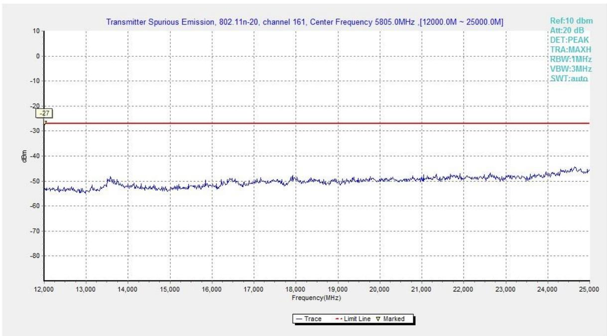
**Fig. 25 Conducted Spurious Emission (802.11n-HT20, Ch161, 12 GHz-25 GHz)**
