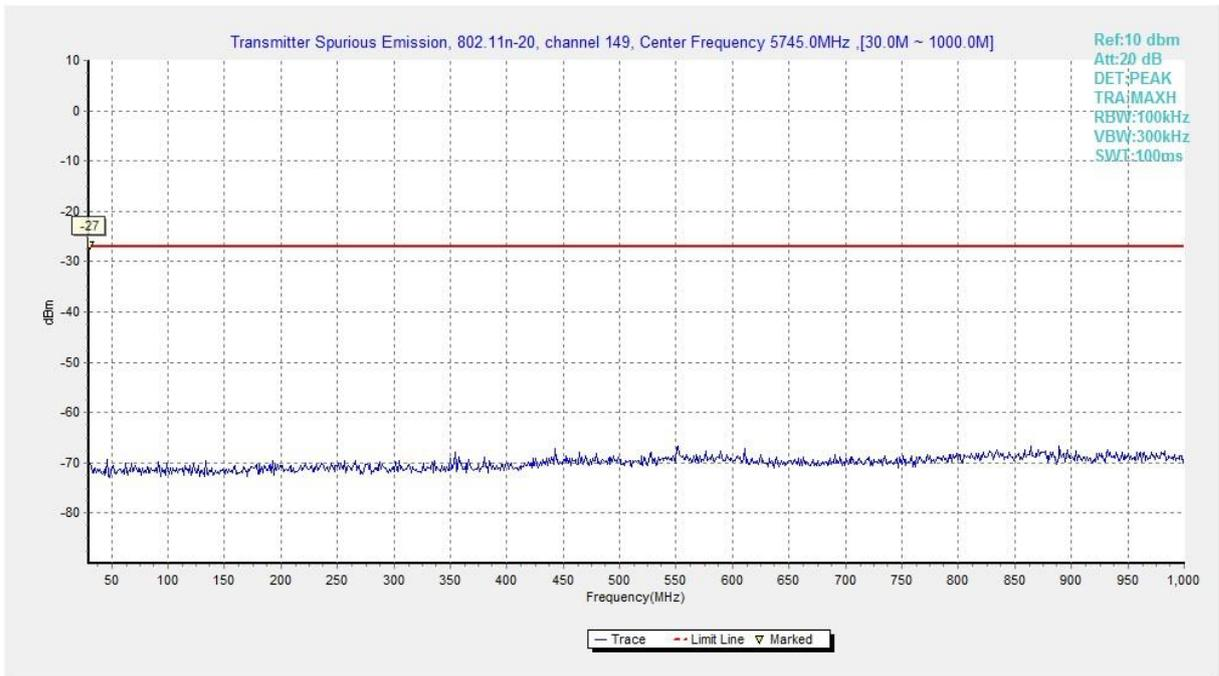
**Fig. 15 Conducted Spurious Emission (802.11n-HT20, Ch149, 30 MHz-1 GHz)**
