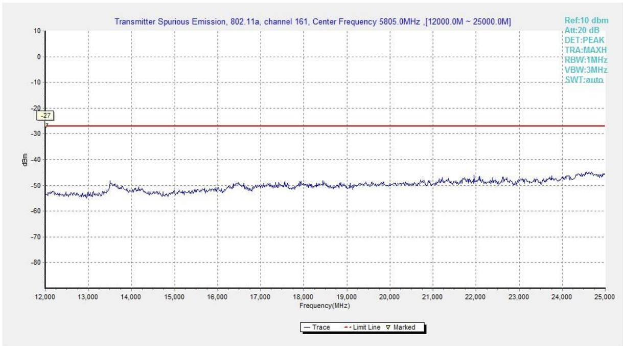
**Fig. 13 Conducted Spurious Emission (802.11a, Ch161, 12 GHz-25 GHz)**
