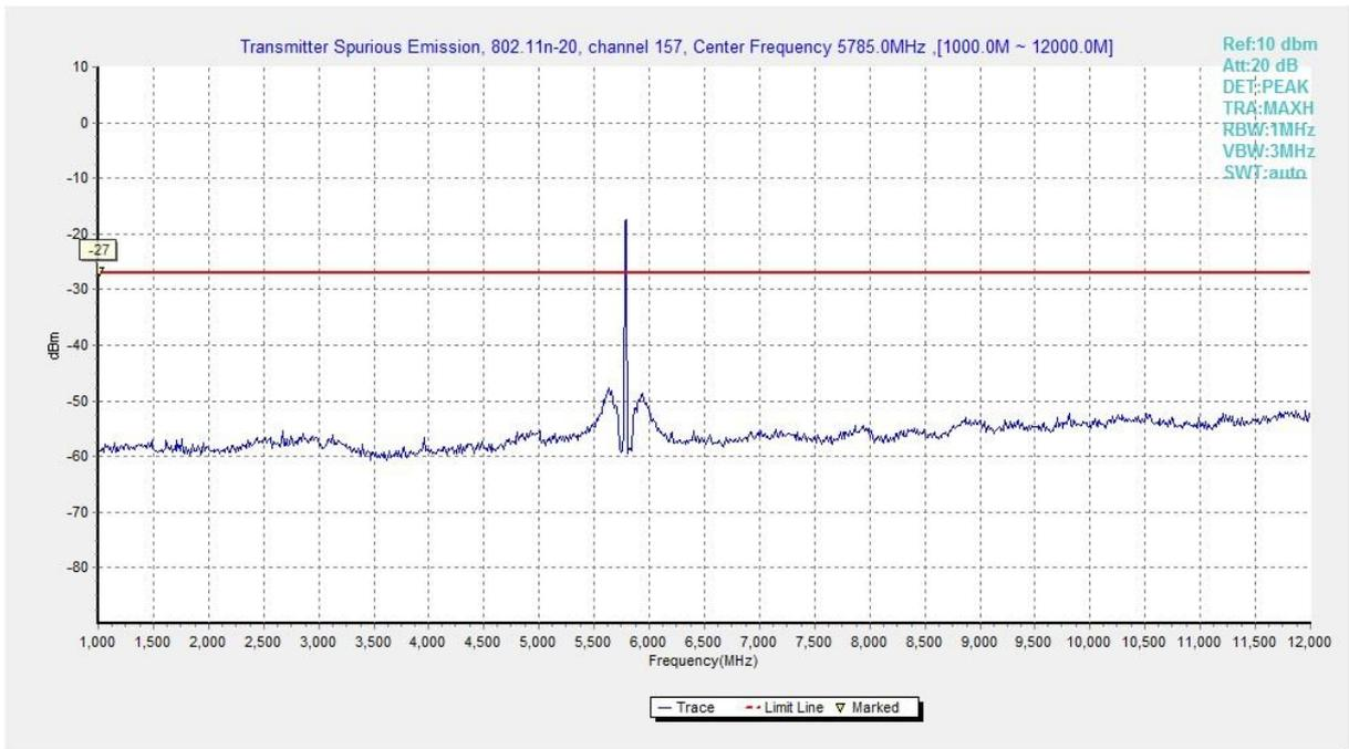
**Fig. 20 Conducted Spurious Emission (802.11n-HT20, Ch157, 1 GHz -12 GHz)**
