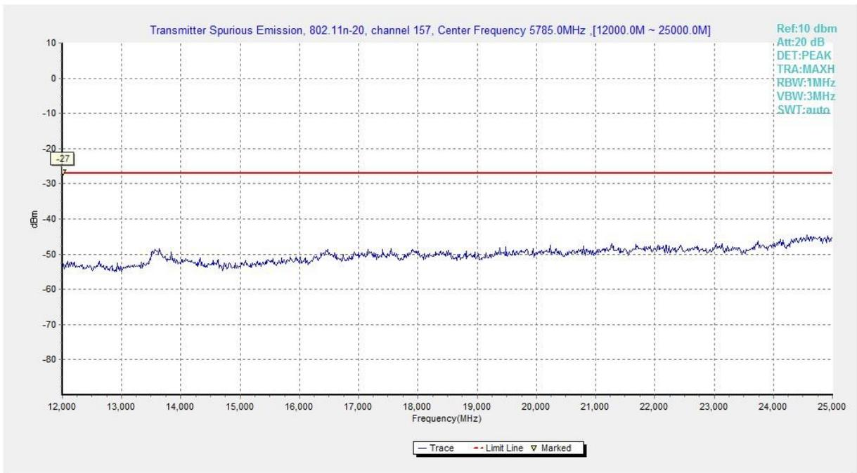
**Fig. 21 Conducted Spurious Emission (802.11n-HT20, Ch157, 12 GHz-25 GHz)**
