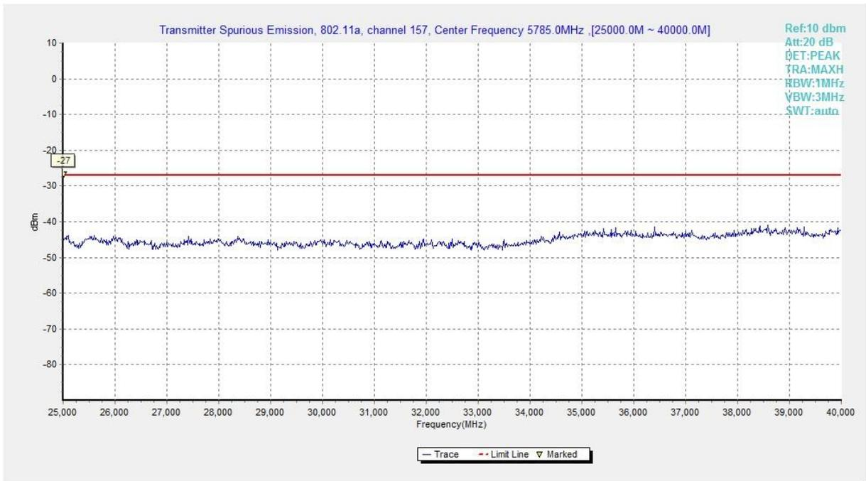
**Fig. 10 Conducted Spurious Emission (802.11a, Ch157, 25 GHz-40 GHz)**
