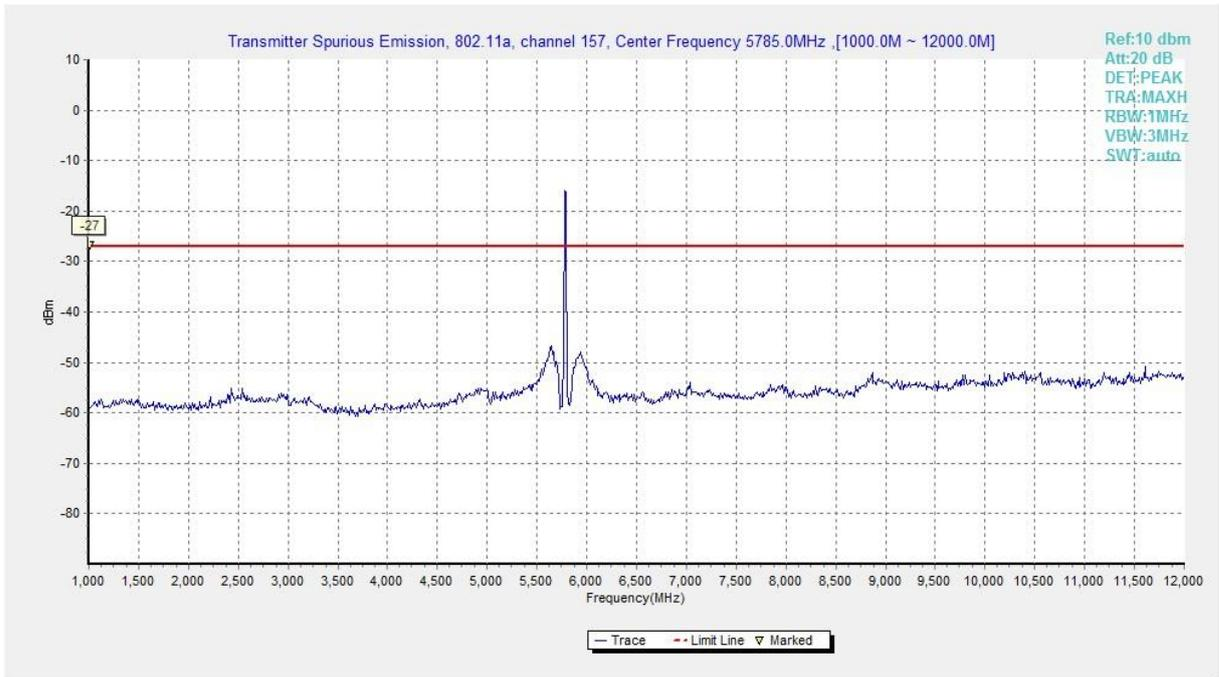
**Fig. 8 Conducted Spurious Emission (802.11a, Ch157, 1 GHz -12 GHz)**
