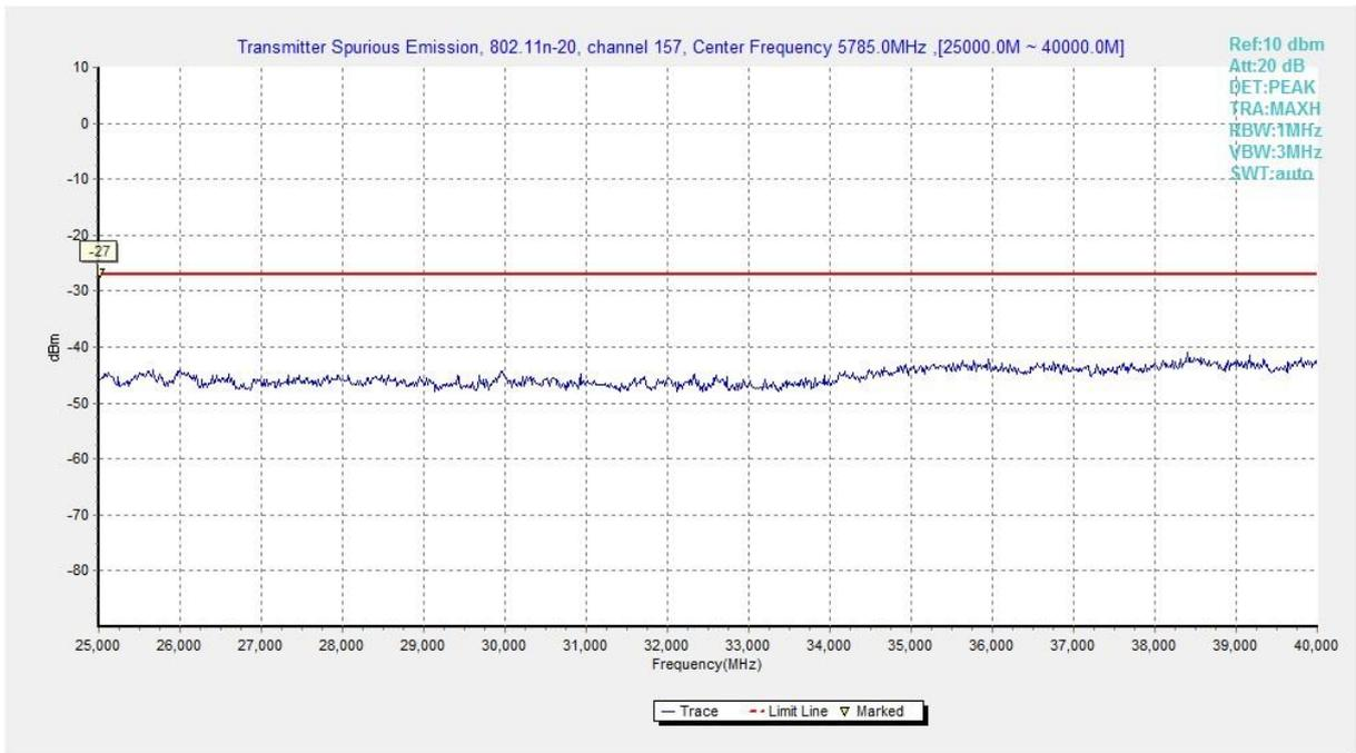
**Fig. 22 Conducted Spurious Emission (802.11n-HT20, Ch157, 25 GHz-40 GHz)**
