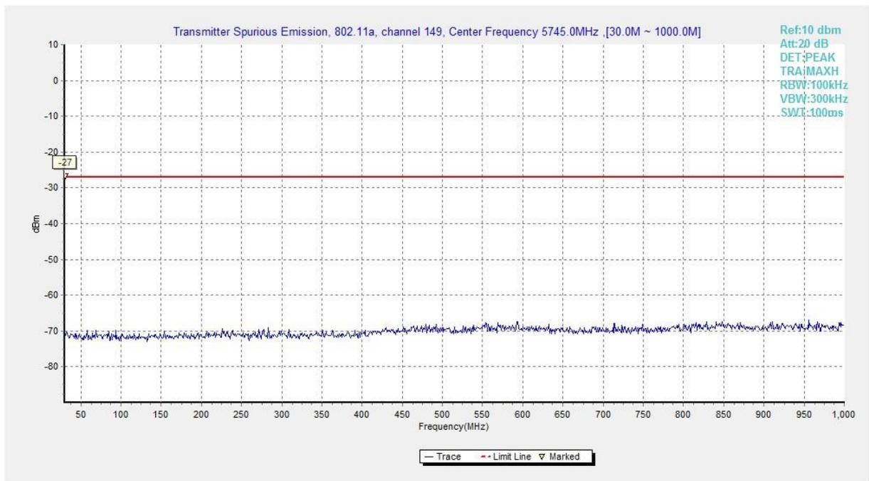
**Fig. 3 Conducted Spurious Emission (802.11a, Ch149, 30 MHz-1 GHz)**
