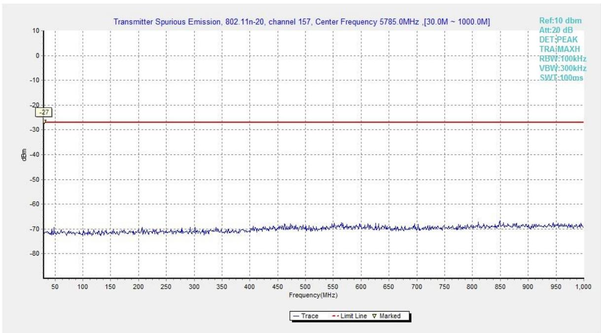
**Fig. 19 Conducted Spurious Emission (802.11n-HT20, Ch157, 30 MHz-1 GHz)**
