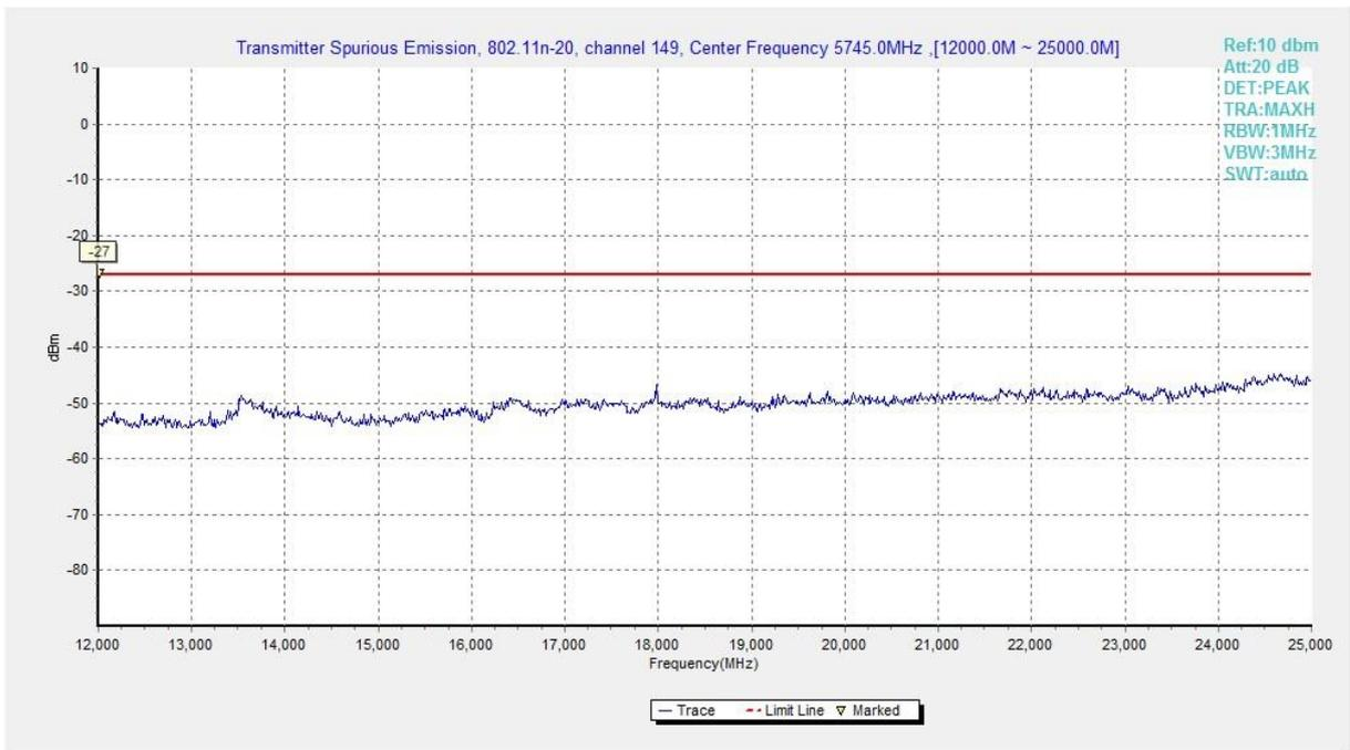
**Fig. 17 Conducted Spurious Emission (802.11n-HT20, Ch149, 12 GHz-25 GHz)**
