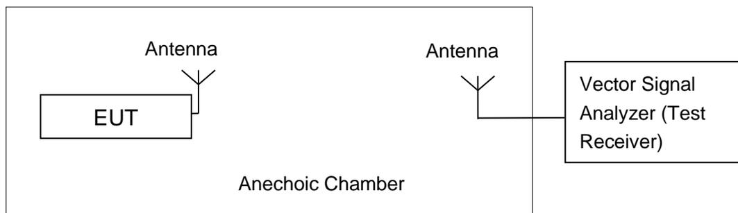
The measurement is made according to ANSI C63.10.
