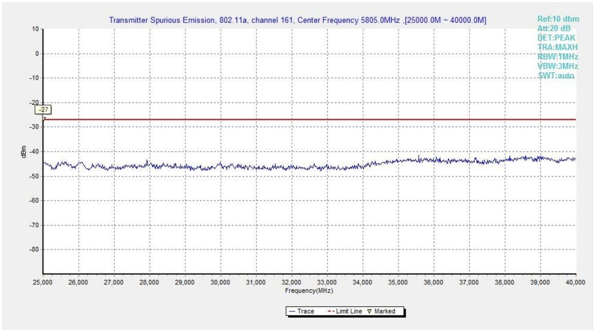
**Fig. 14 Conducted Spurious Emission (802.11a, Ch161, 25 GHz-40 GHz)**
