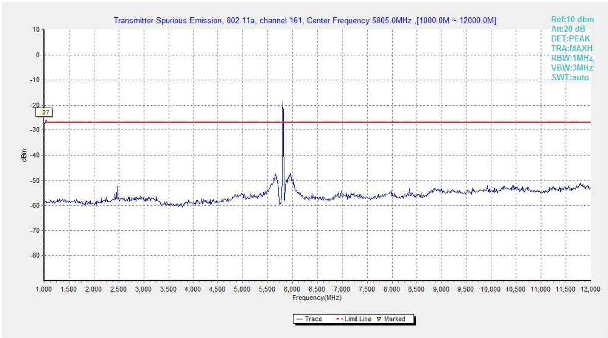
**Fig. 12 Conducted Spurious Emission (802.11a, Ch161, 1 GHz -12 GHz)**
