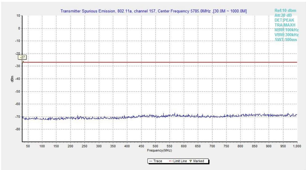
**Fig. 7 Conducted Spurious Emission (802.11a, Ch157, 30 MHz-1 GHz)**
