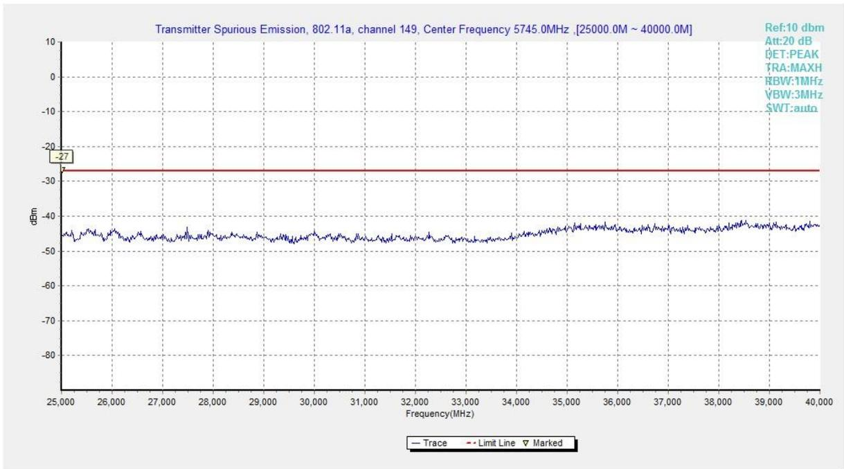
**Fig. 6 Conducted Spurious Emission (802.11a, Ch149, 25 GHz-40 GHz)**
