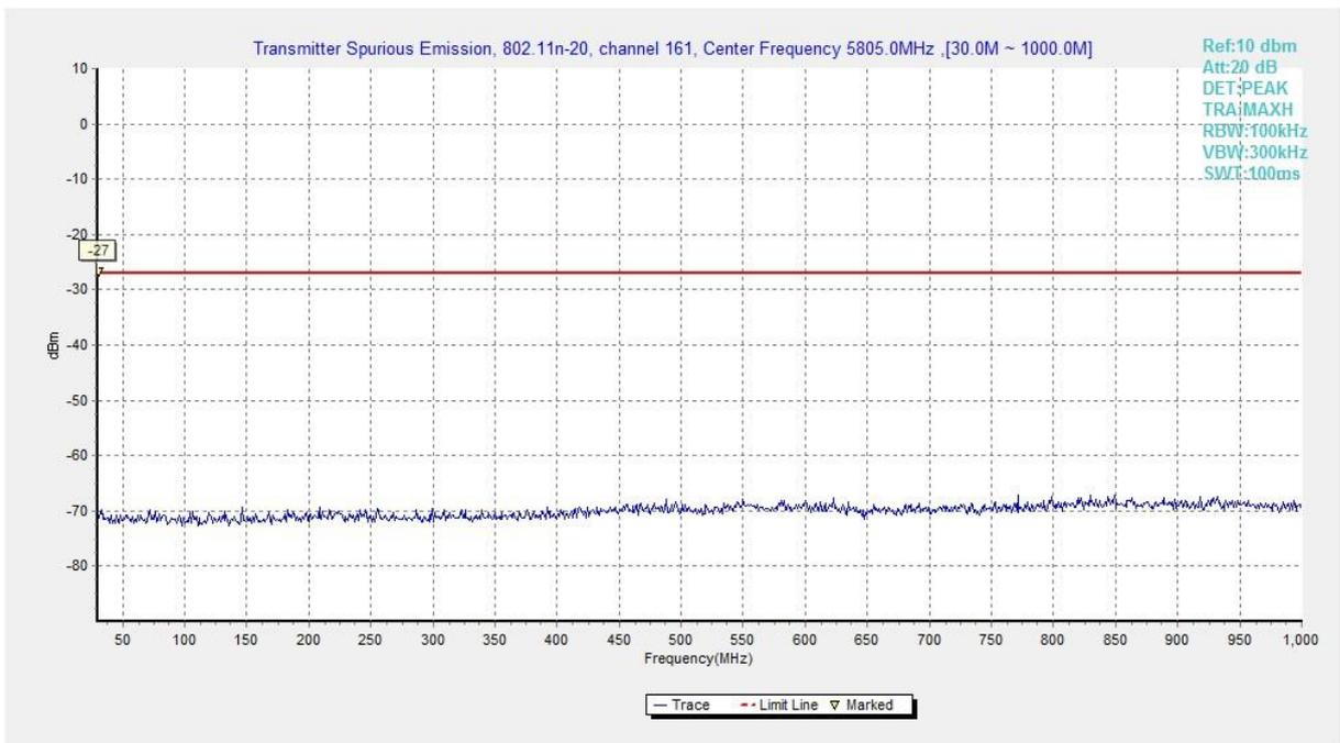
**Fig. 23 Conducted Spurious Emission (802.11n-HT20, Ch161, 30 MHz-1 GHz)**
