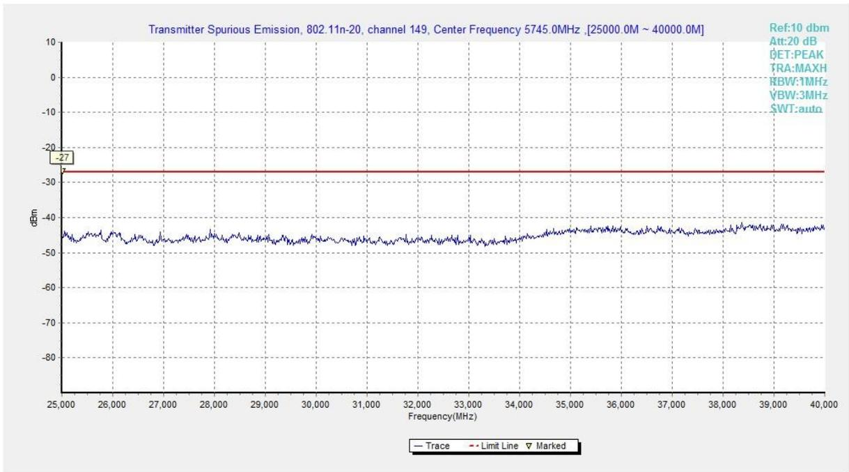
**Fig. 18 Conducted Spurious Emission (802.11n-HT20, Ch149, 25 GHz-40 GHz)**
