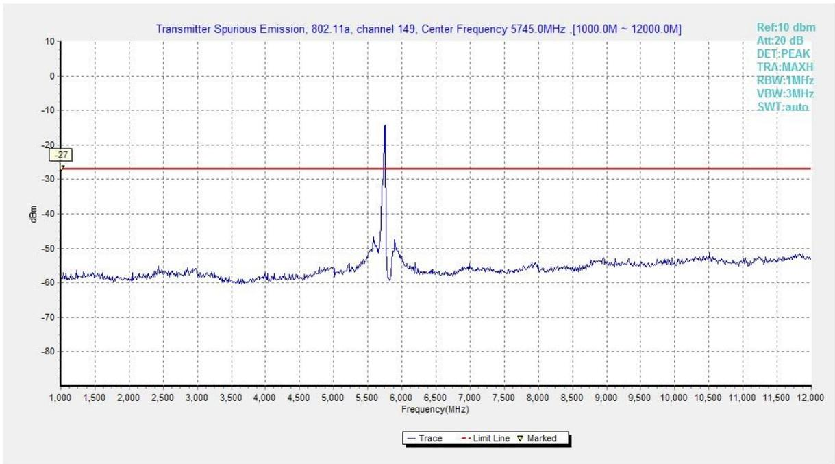
**Fig. 4 Conducted Spurious Emission (802.11a, Ch149, 1 GHz -12 GHz)**
