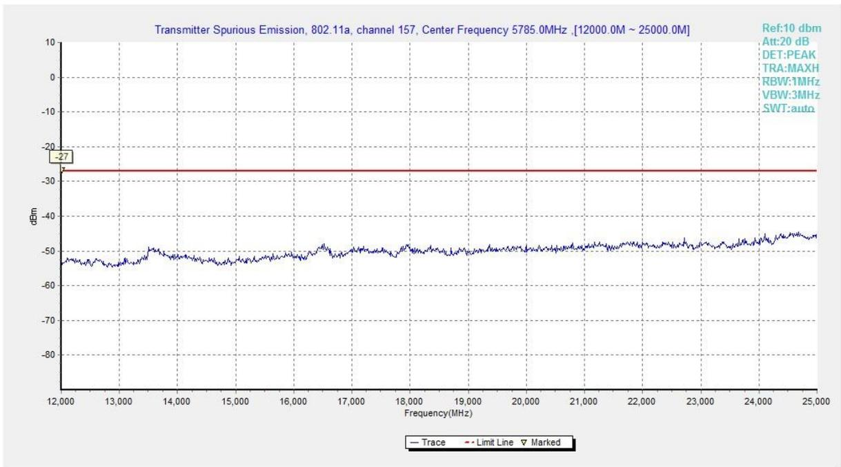
**Fig. 9 Conducted Spurious Emission (802.11a, Ch157, 12 GHz-25 GHz)**
