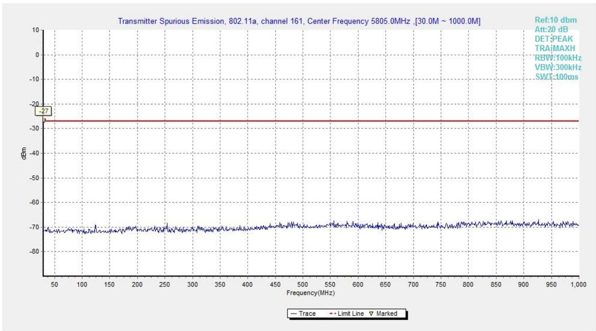
**Fig. 11 Conducted Spurious Emission (802.11a, Ch161, 30 MHz-1 GHz)**
