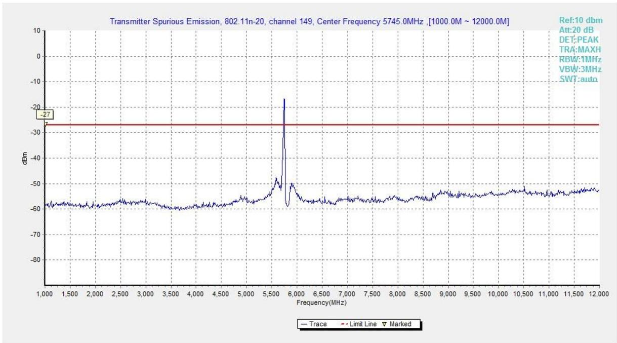
**Fig. 16 Conducted Spurious Emission (802.11n-HT20, Ch149, 1 GHz -12 GHz)**
