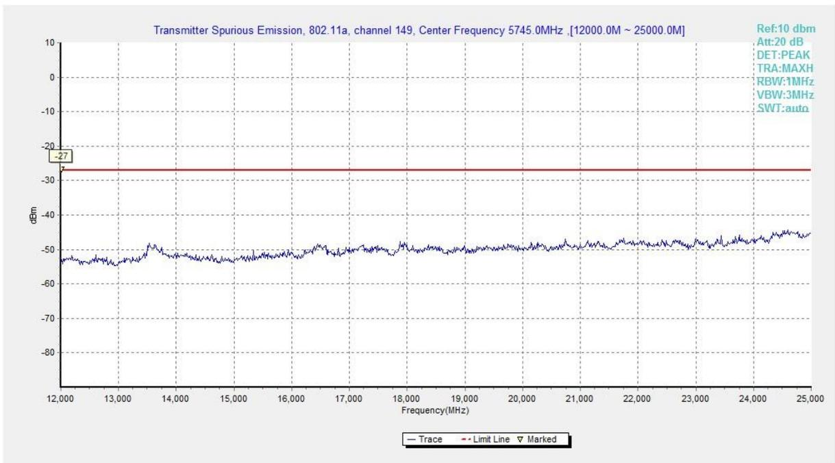
**Fig. 5 Conducted Spurious Emission (802.11a, Ch149, 12 GHz-25 GHz)**
