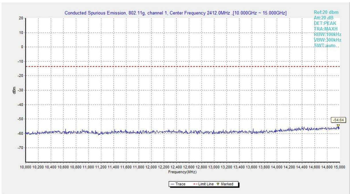
**Fig.A.6.1.132 Transmitter Spurious Emission - Conducted (802.11g, Ch1, 10 GHz-15 GHz)**
