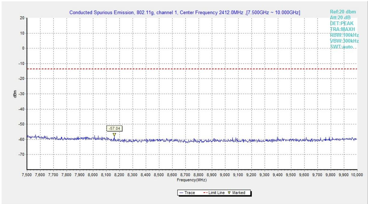
**Fig.A.6.1.131 Transmitter Spurious Emission - Conducted (802.11g, Ch1, 7.5 GHz-10 GHz)**
