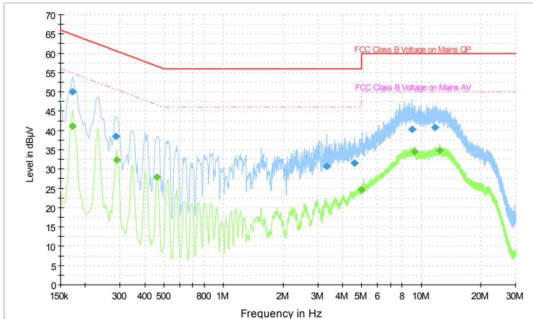
**Fig.A.9.2 AC Powerline Conducted Emission-Idle EUT3(M2001J2G)+AE1+AE3+AE6**
