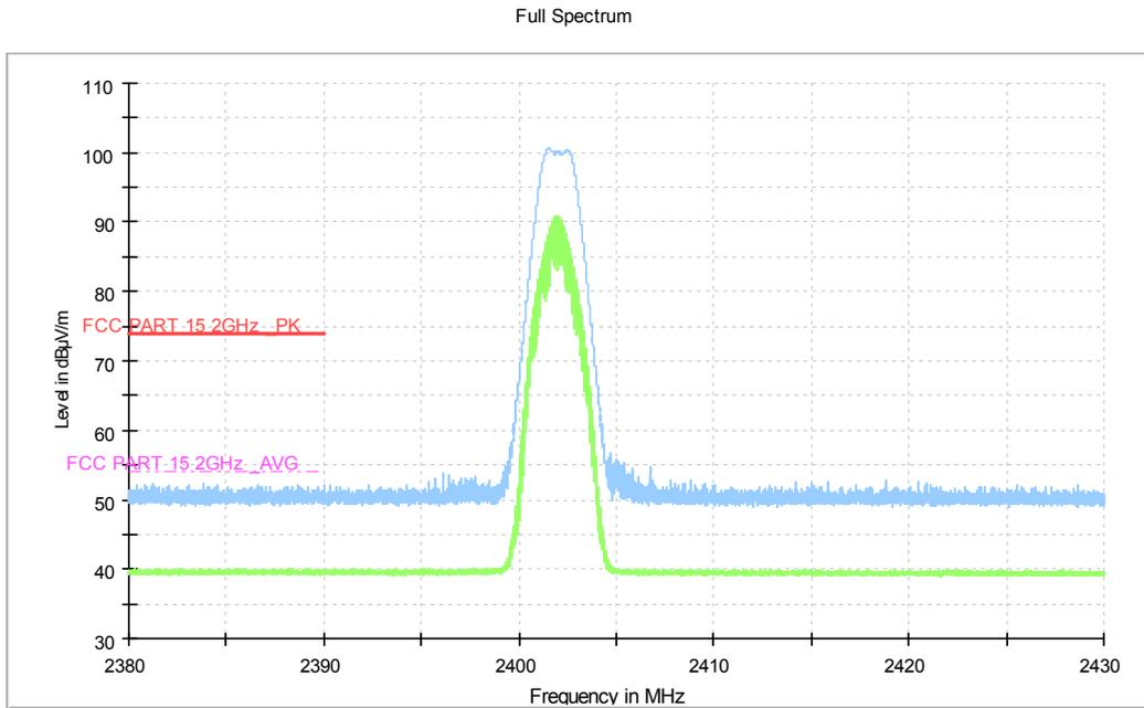
**Fig.5. Frequency Band Edges: EUT3 ANT3 BLE 5.0 GFSK, 2402 MHz, Hopping Off, 2.38 GHz – 2.45GHz**
