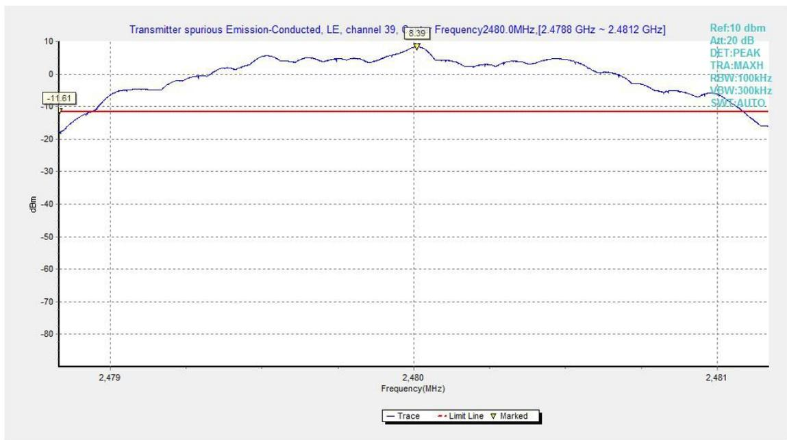
**Fig.21.** Transmitter Spurious Emission - Conducted: GFSK, 2480 MHz
