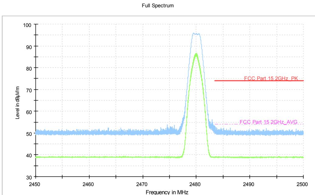
**Fig.6. Frequency Band Edges: EUT3 ANT3 BLE 5.0 GFSK, 2480 MHz, Hopping Off , 2.45 GHz - 2.50GHz**
