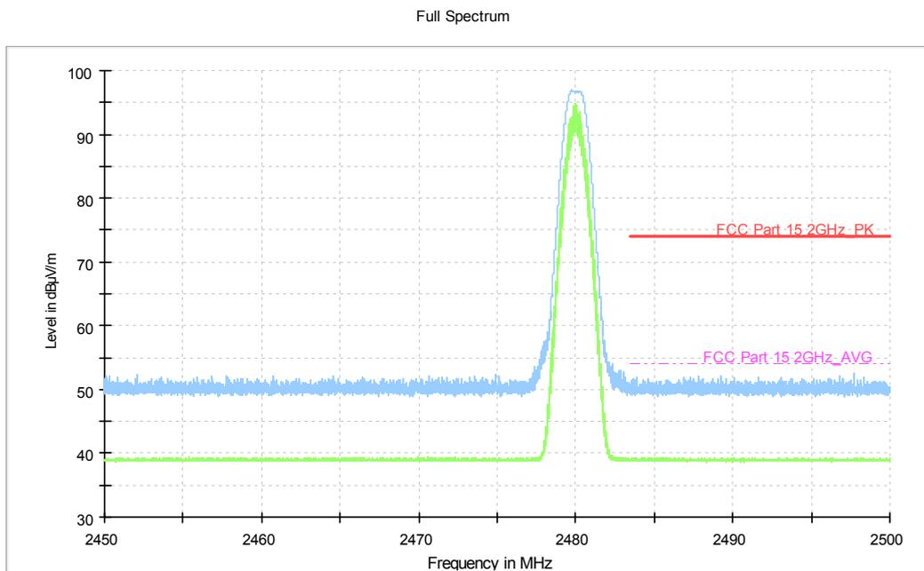
**Fig.8. Frequency Band Edges: EUT4 ANT4 BLE 4.0 GFSK, 2480 MHz, Hopping Off , 2.45 GHz - 2.50GHz**
