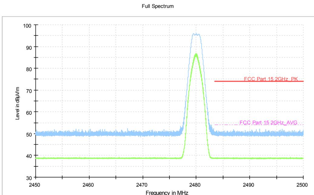
**Fig.10. Frequency Band Edges: EUT4 ANT4 BLE 5.0 GFSK, 2480 MHz, Hopping Off , 2.45 GHz - 2.50GHz**
