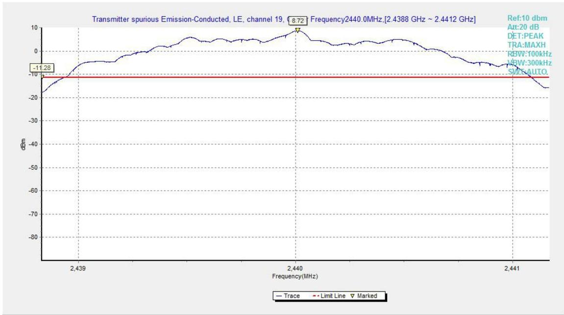
**Fig.16.** Transmitter Spurious Emission - Conducted: GFSK, 2440MHz
