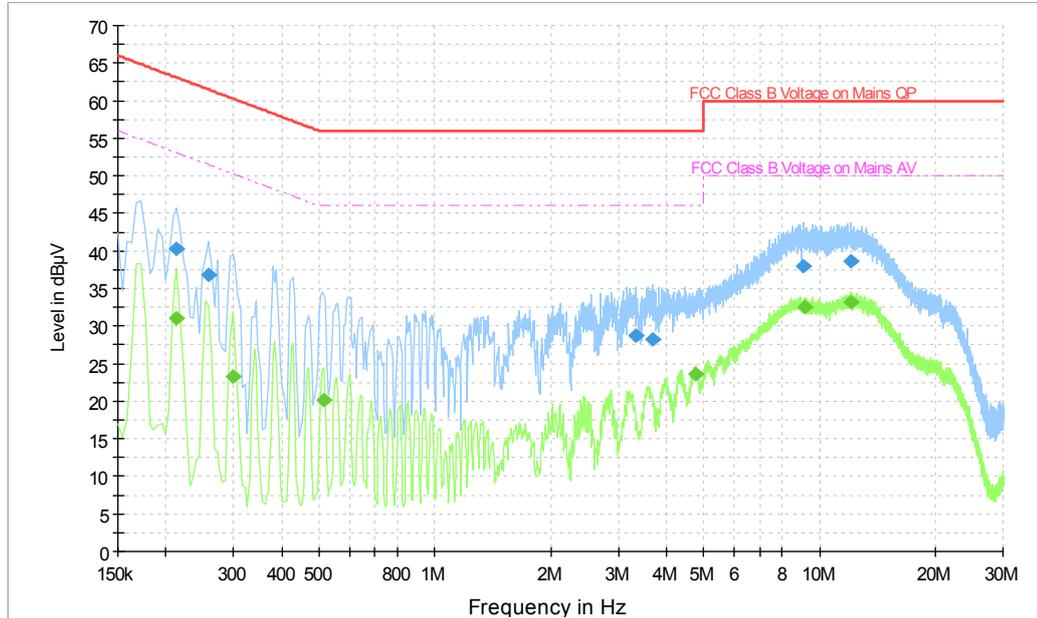
**Fig.A.9.1 AC Powerline Conducted Emission- Bluetooth EUT3(M2001J2G)+AE1+AE3+AE6**
